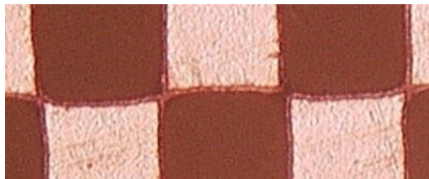
Figure 4.5.1. Localised over-etching observed in the 1.94mm PSL etched onto the 0.76mm substrate and photographed using the Hirox imager.
