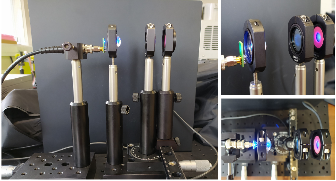
Figure A.1: Reference to the test setup employed for the validation. On the left, the test setup is seen from the side. The black wall in the background is used to keep an opaque dark cover to avoid any background illumination interference. On the top right, a test setup close-up. On the bottom right, the test setup is seen from the top.
