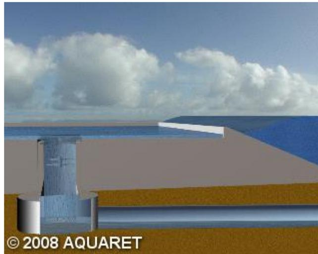
Figure 1.4 generic view of overtopping devices (EMEC)
