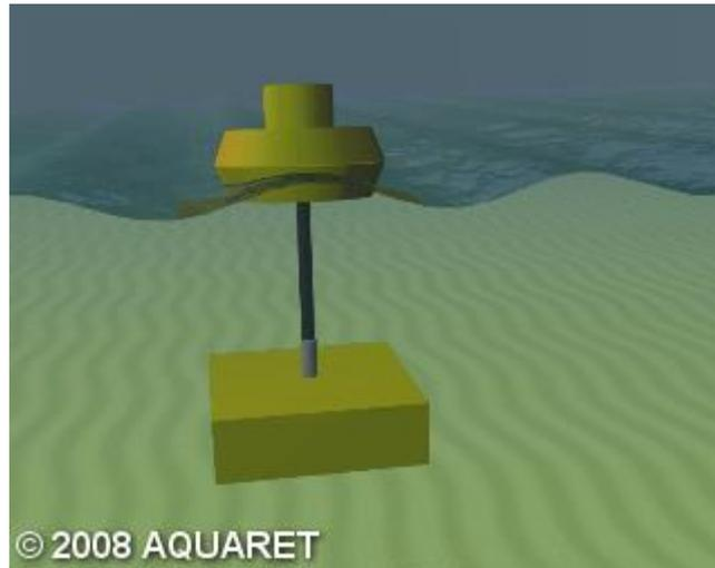
Figure 1.2 Generic view of point absorber type WEC (EMEC)
