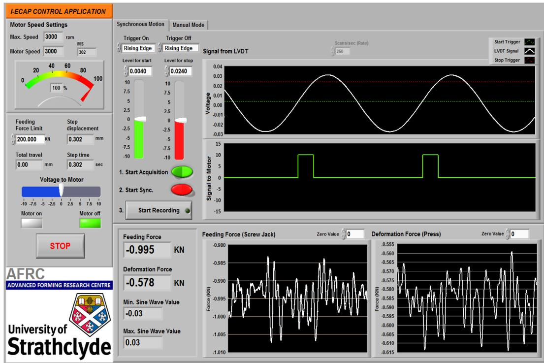
Figure 3.13: IECAP custom virtual instrument front panel.
