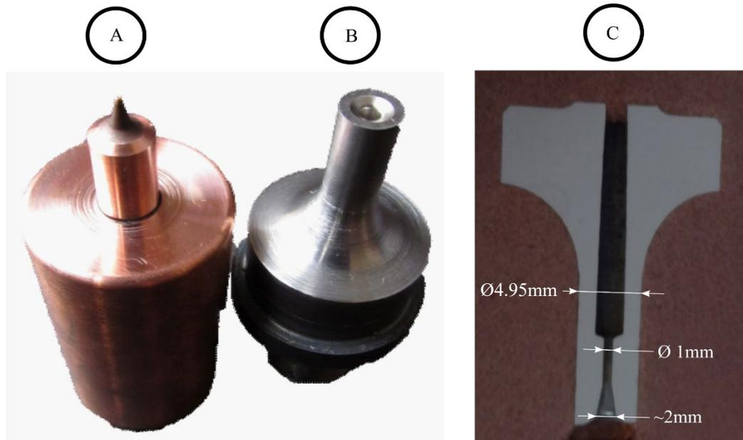
**Figure 3.24:** *A- the copper electrode used for the sink EDM manufacture of the single pin punch. B- the fully fabricated single pin punch. C- single pin punch sectioned in half so the profile of the cavity can be verified.*
