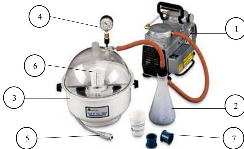
**Figure 3.4:** *Castable Mounting Equipment: (1) Vacuum pump, (2) air filtration chamber, (3) vacuum chamber, (4) vacuum pressure indicator, (5) motorised base for rotating specimens, (6) EpoThin 2 resin and hardener mixed and ready for pouring, (7) casting moulds.*
