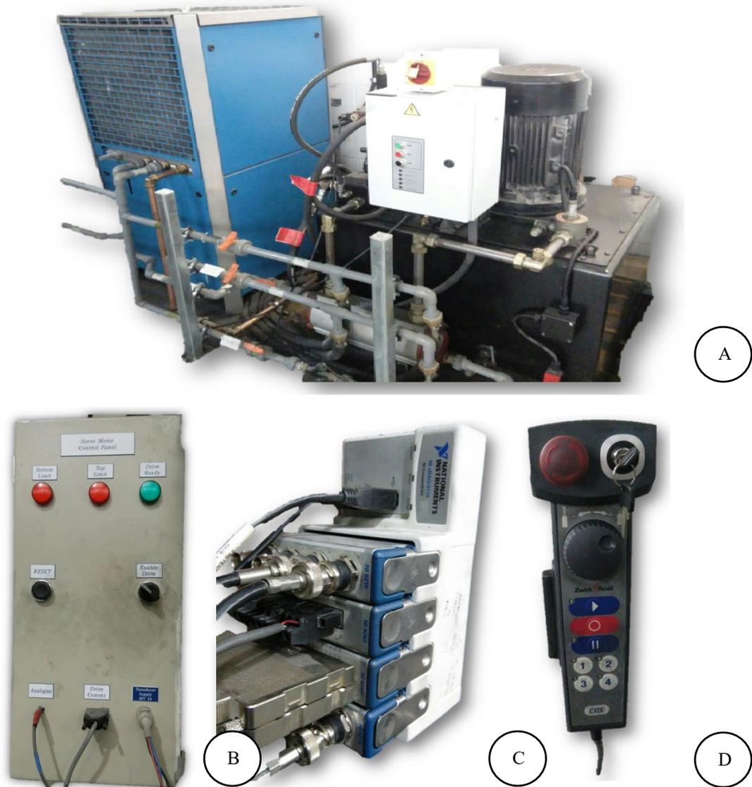
**Figure 3.12:** *Other hardware used for the IECAP rig. A- the black hydraulic storage tanks and pump, the blue chiller. B- rig's electrical components control and safety box. C- 4 National instruments modules used to control and record rig movement. D- manual control hand controller.*
