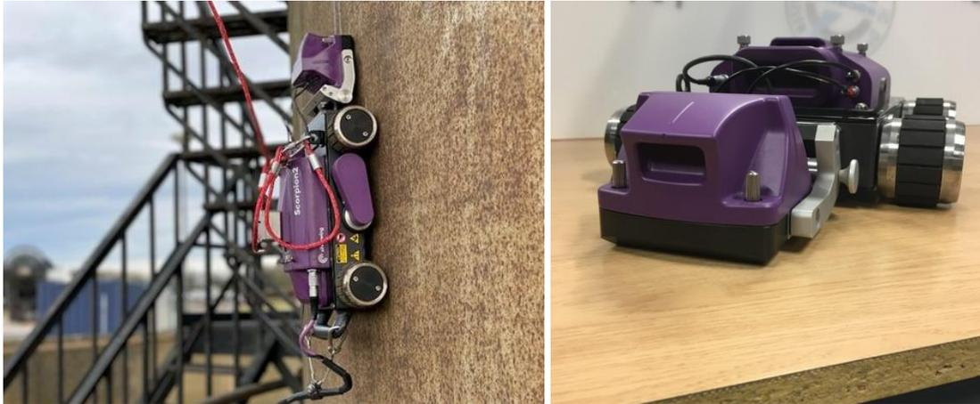
*Fig. 14 A) The Scorpion 2 vertically traversing a ferromagnetic above ground tanker wall [83]. B) A close shot of the Scorpion 2 showing the dry coupled sensor head [84].*
