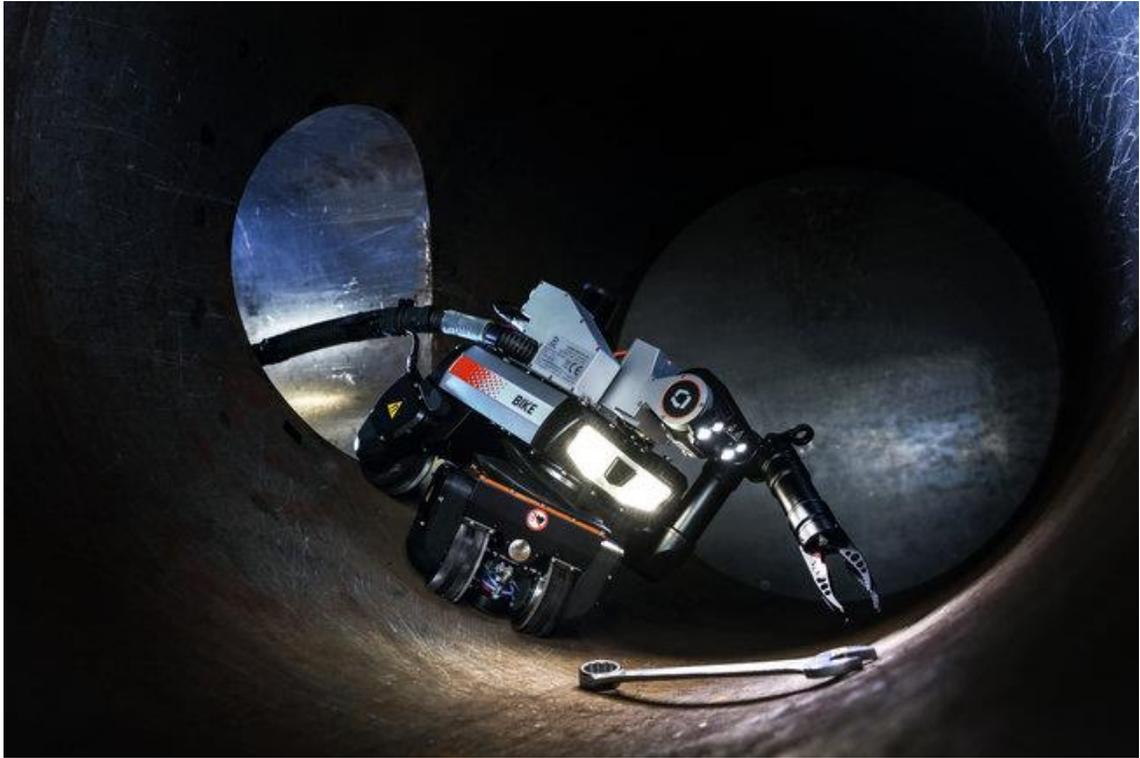
*Fig. 13 The Waygate Technologies BIKE, equipped with manipulating arm and a piezoelectric ultrasonic transducer. This robot is remote controlled and the operator utilises the camera in between the lights to inspect the subject. Adapted from [47].*
