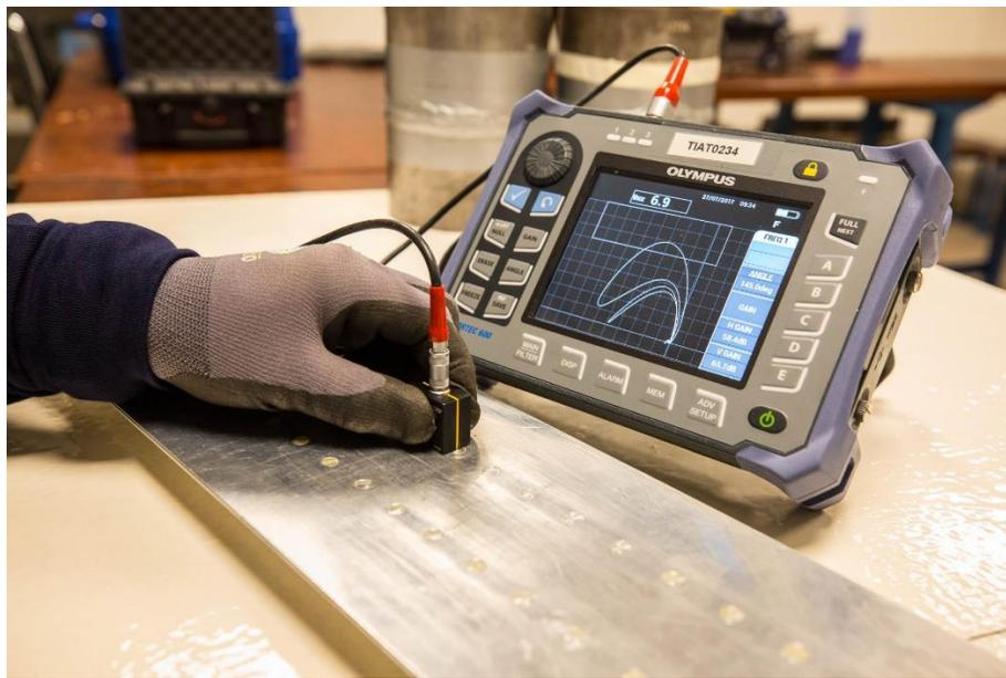
*Fig. 12 An example of typical Eddy Current inspection measuring plate thickness [62].*
