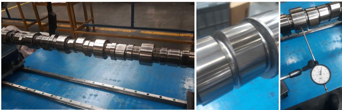
Figure 5-12: Camshaft curvature and gears were checked, all lobes were inspected and measured.
