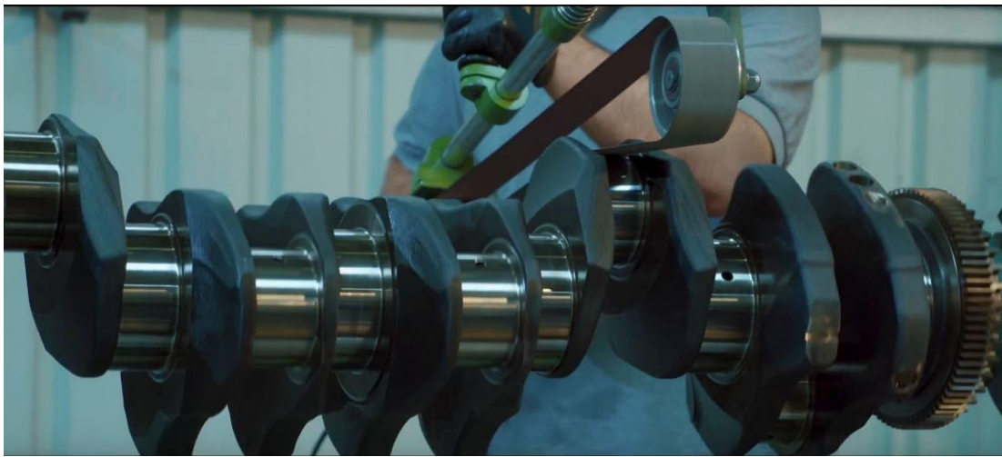
Figure 5-13: Crankshaft polishing after grinding operation.
