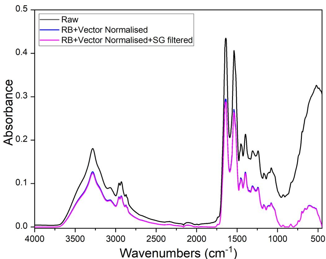
Figure 2-13: Final step of pre-processing where SG filter is applied for noise reduction (shown in magenta).
