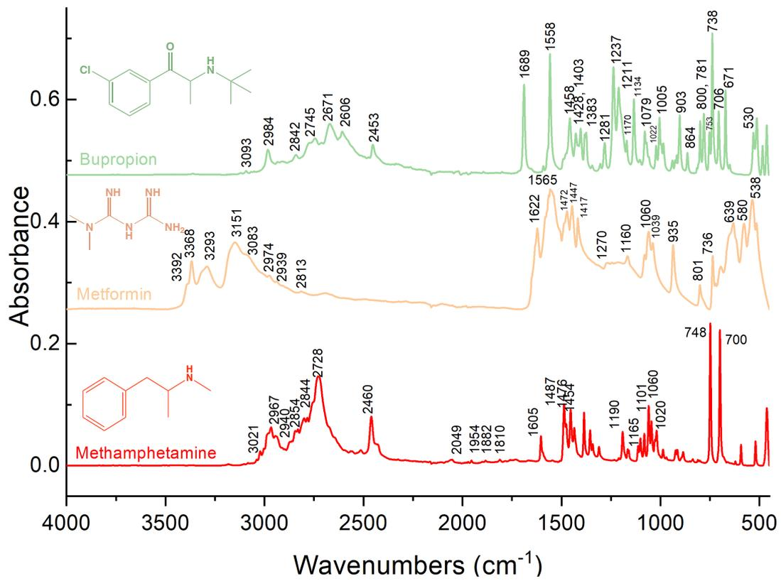
Figure A3-2: Stacked spectra for powder bupropion and metformin with labelled peaks.
