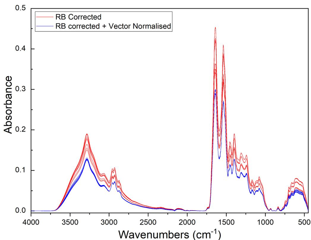
Figure 2-12: Baseline corrected spectra in red show variation across repeats, which is significantly reduced in the vector normalised spectra shown in blue.
