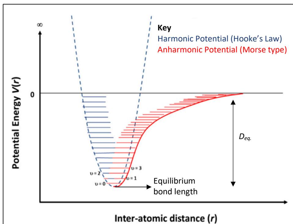
Figure 2-3: Morse potential energy diagram for harmonic (blue) and anharmonic (red) oscillation (adapted from Baker *et al.* 2016).
