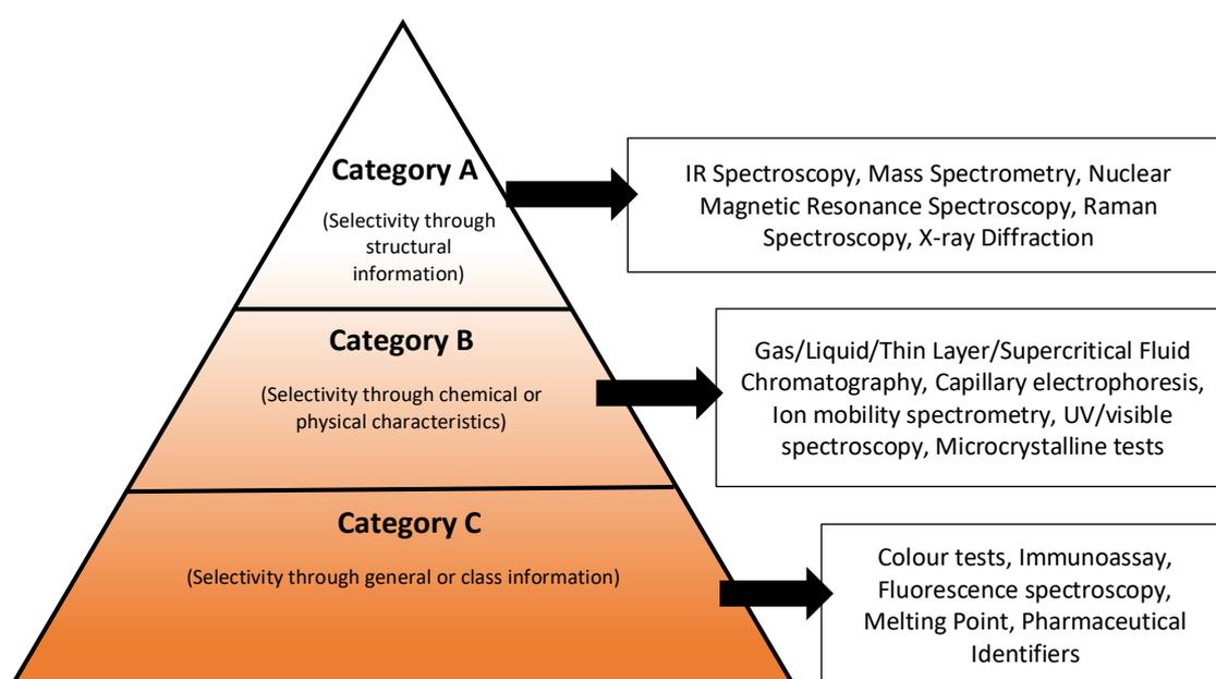
Figure 1-3: Schematic showing the categories of various analytical techniques employed in the analysis of seized drug samples. The image is adapted from SWGDRUG documentation.
