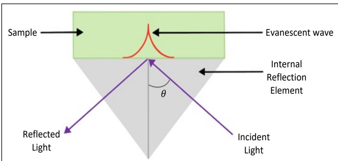
Figure 2-7 Schematic representation of the ATR sampling mode through a traditional diamond crystal (here labelled as internal reflection element), where  $\theta$  represents the angle of incidence.
