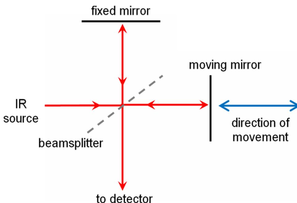
Figure 2-5: Schematic of a Michelson interferometer used to measure an FTIR interferogram. Figure adapted from Baker *et al.* 2016.
