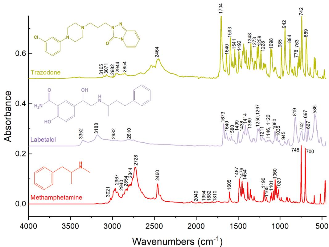
Figure A3-1: Stacked spectra of powder MA, Labetalol and Trazodone with labelled peaks.
