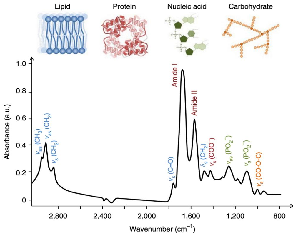
Figure 2-9: FTIR spectrum showing the four primary types of biomolecules found in a biological sample. The spectrum is labelled with peaks assigned to specific vibrations found in each of these biomolecules. (Reproduced from Baker *et al.* 2016).
