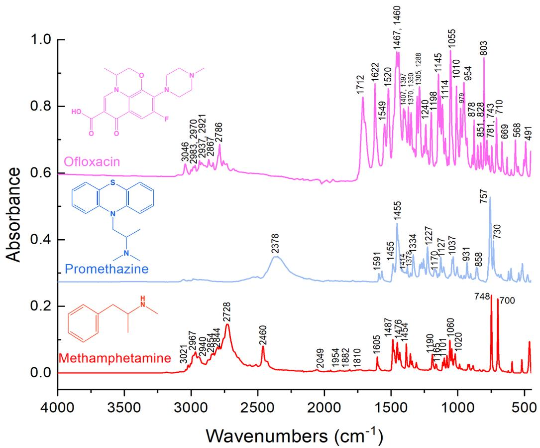
Figure A3-3: Stacked spectra for powder promethazine and ofloxacin with labelled peaks.
