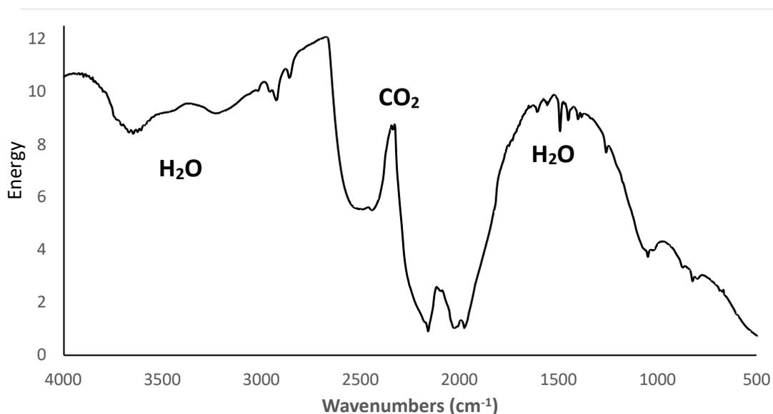
Figure 2-6: A background spectrum collected before sample analysis that shows atmospheric gases such as water vapour and carbon dioxide.
