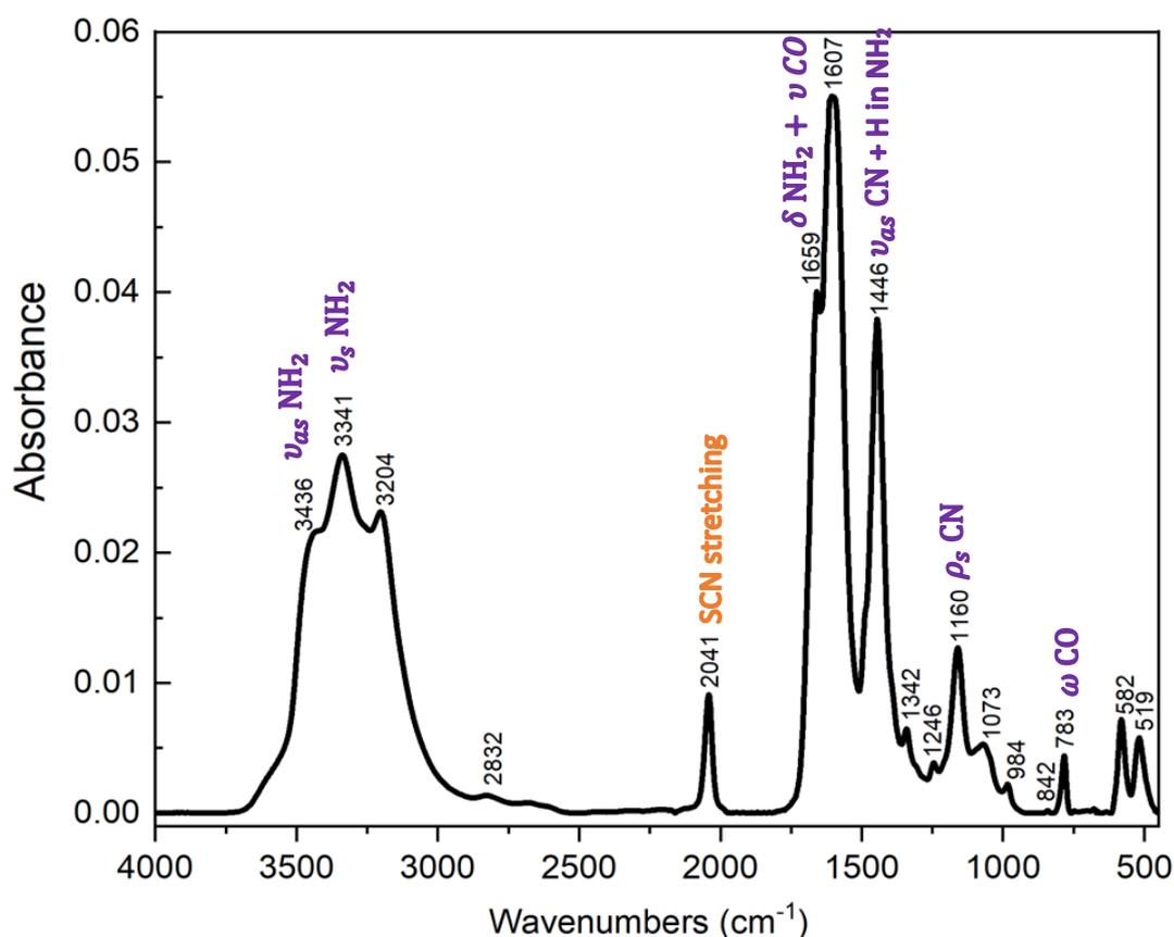
Figure 2-10: Air dried FTIR spectrum of artificial urine (Surine™) with tentative vibrational mode assignments.
