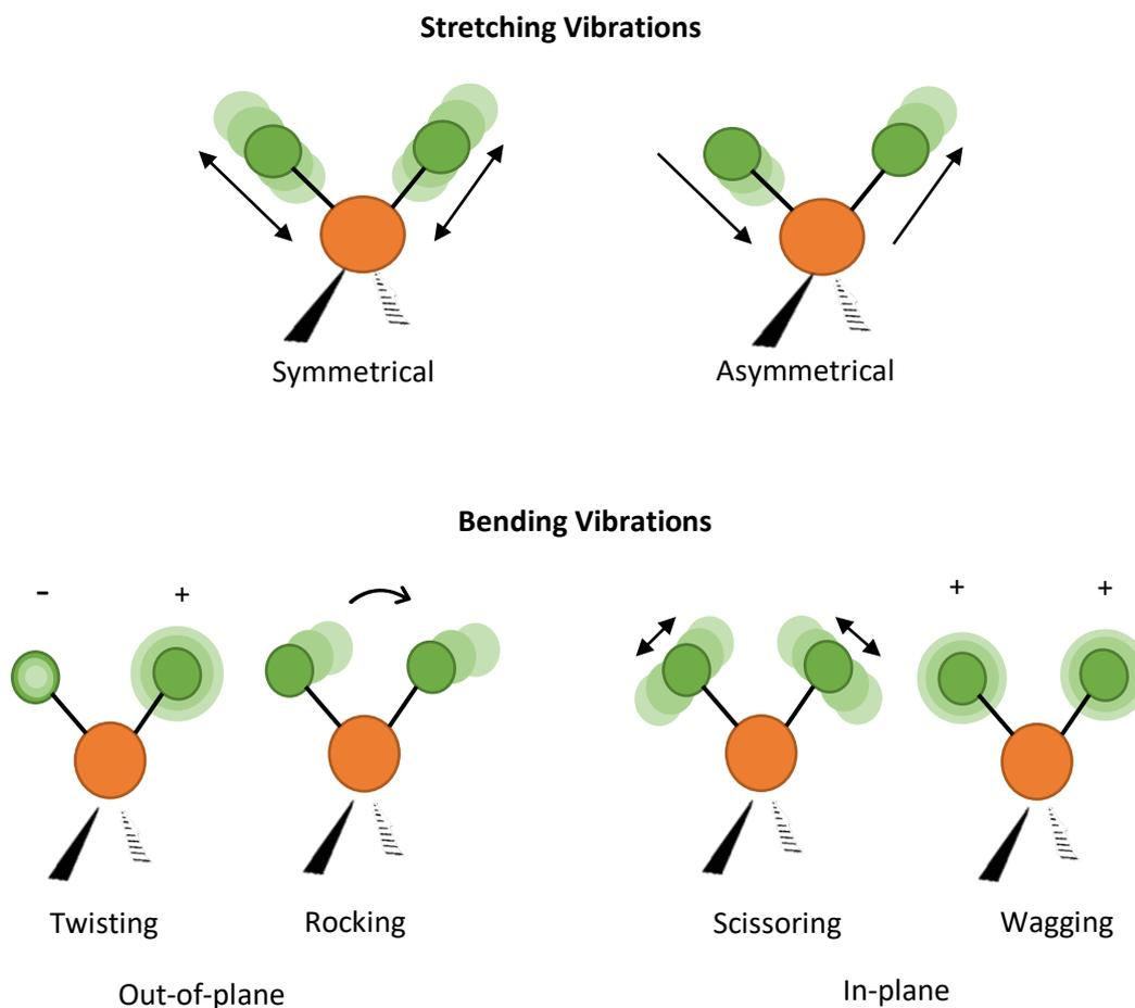
Figure 2-4: Molecular vibrations observed for non-linear molecules in mid-IR spectroscopy.
