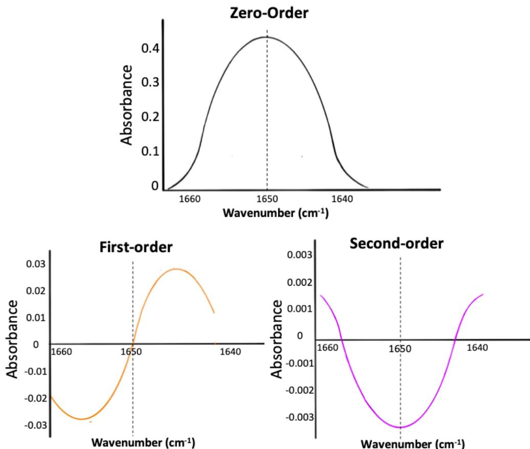
Figure 2-14: Representation of zero-order absorption band (top) and their corresponding first-order (bottom left) and second-order (bottom right) derivatives.
