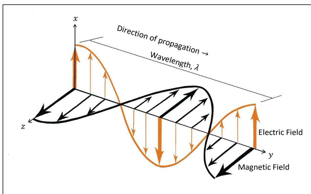
Figure 2-1: Perpendicular relationship between electric and magnetic fields of an electromagnetic wave, showing wavelength,  $\lambda$ .
