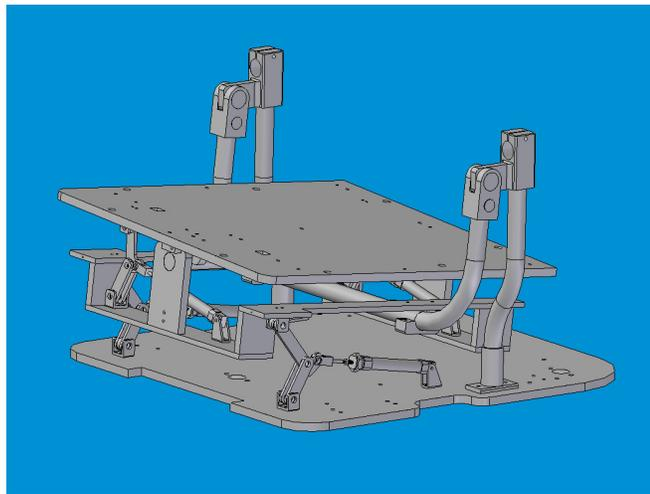
**Figure 4.8 – CAD model of final tilt assembly (shown with armrest assembly in place)**
