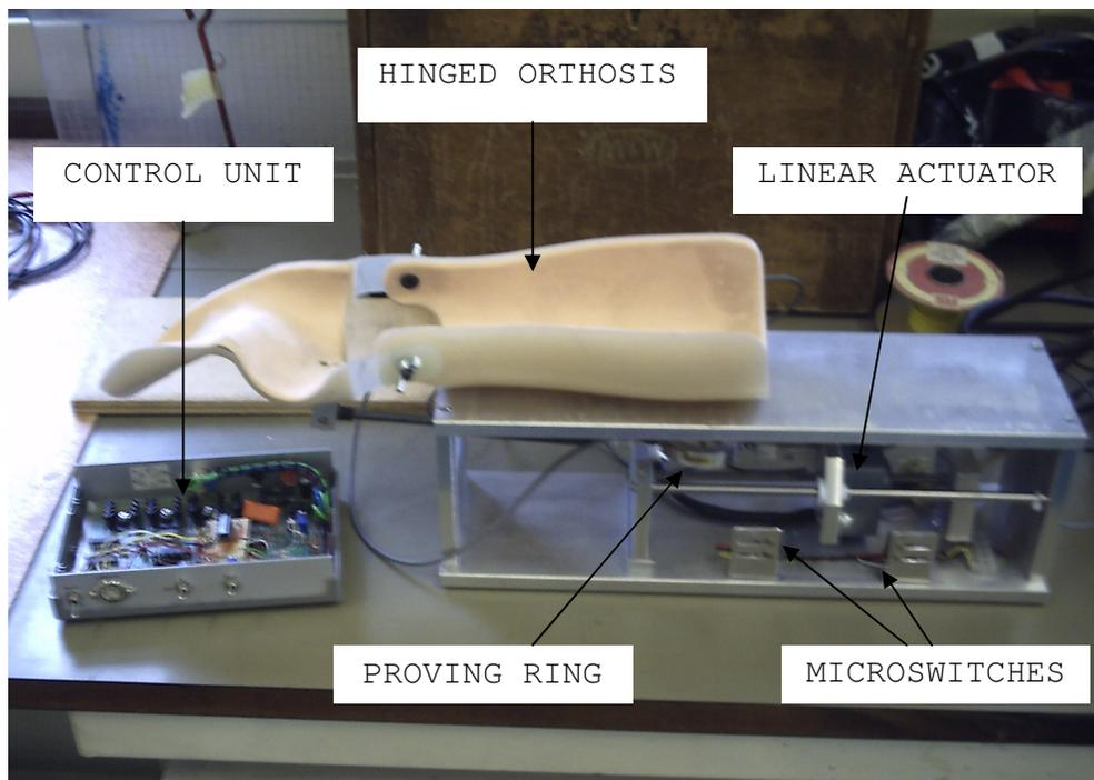
**Figure 5.2 – Prototype active dynamic orthosis**
