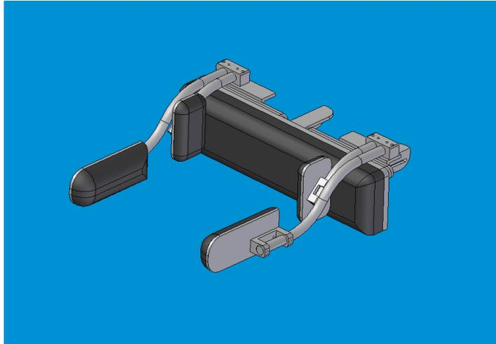
**Figure 4.20 – CAD model of full lateral support assembly (used in prototype)**
