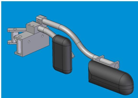
**Figure 4.19 – CAD model of dynamic version of lateral support assembly**
