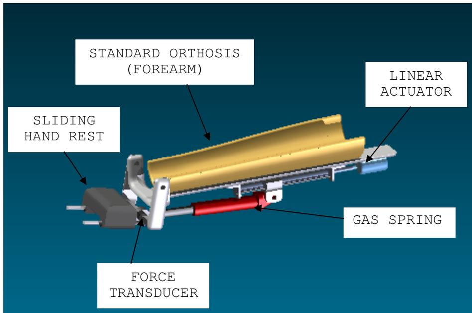
**Figure 5.1 – CAD model of active dynamic orthosis for the wrist**
