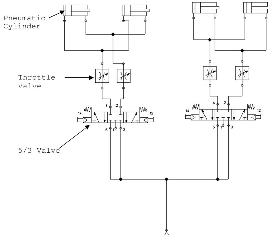
**Figure 4.9 – Schematic diagram of pneumatic circuit used to provide coronal and sagittal tilt (drawn with reference to ISO 1219 parts 1 and 2: Fluid power systems and components – Graphic symbols and circuit diagrams)**
