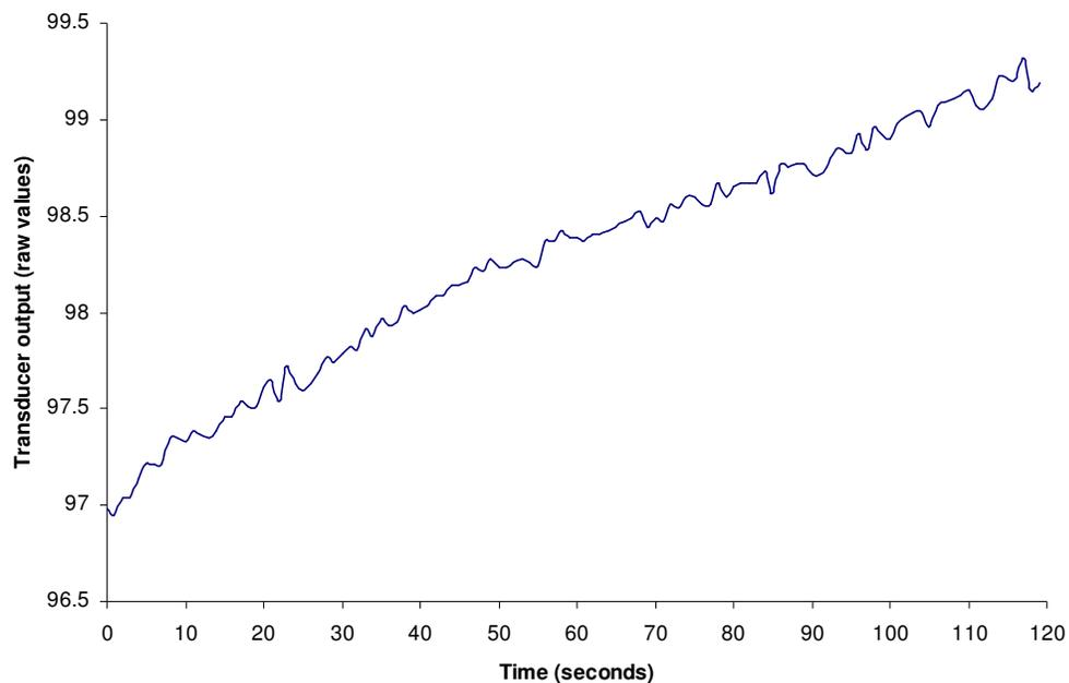
**Figure 7.5 – Output from transducer loaded with a constant pressure of 350mmHg**
