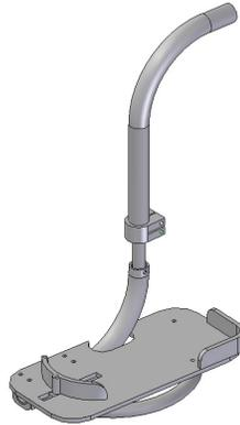
**Figure 4.18 – CAD model of final footrest assembly (right hand side)**
