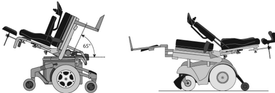
**Figure 2.6 – Tilting adaptive seating system (left) and reclining adaptive seating system (right) (<http://msktc.washington.edu>)**
