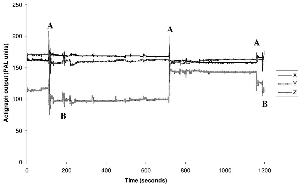
**Figure 6.2 – Example of data output from test session with distinct postural changes (marked A) and transient postural changes (marked B) indicated. X represents changes in the sagittal plane, Y coronal plane and Z tranverse plane. A change of one PAL unit is equivalent to a change in the inclination of the monitor of 1° in the relevant plane.**
