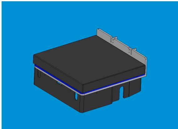
**Figure 4.10 – CAD model of seatbase assembly**
