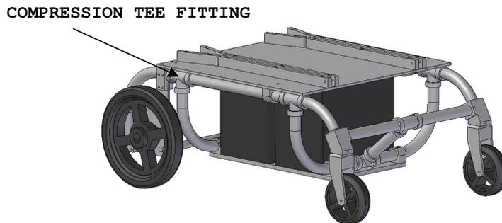
**Figure 4.6 – Final design for powered base unit (prototype version; note plumbing fittings to connect tubing)**
