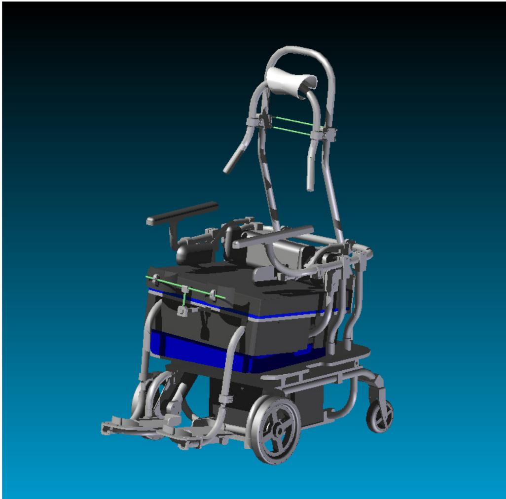
**Figure 4.3 – Rendered CAD model of final design. It is shown here in powered mode and with all orthotic supports in place**
