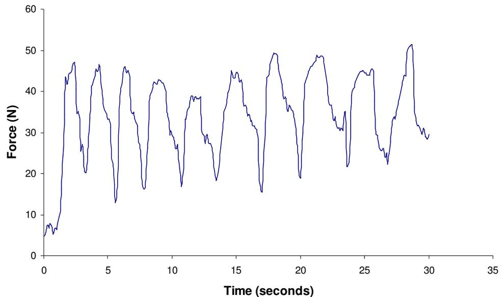
**Figure 5.5 - Force profile from ADO as wrist flexes (x10) and stepper motor is on (test 3)**
