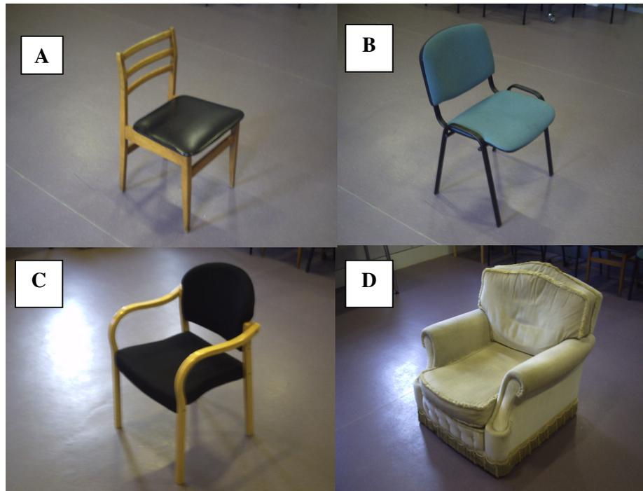
**Figure 6.1 - Chairs used in test. Chair A: a simple wooden framed chair with minimal cushioning on the seat base and an almost vertical, uncushioned, mid-height backrest; Chair B: cushioning on both the seat base and its mid-height and a more reclined backrest than the previous chair; Chair C: more cushioning on both the seat base and the mid-height backrest and armrests (uncushioned); Chair D: a standard well upholstered armchair with cushioned armrests and a relatively high backrest.**
