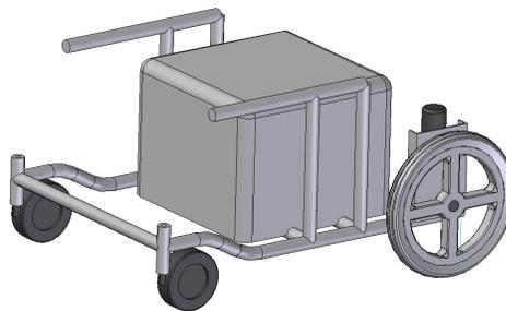
**Figure 4.5 – An early version of the powered base unit**
