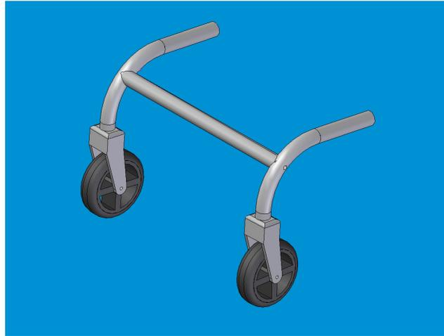
**Figure 4.24 – CAD model of early version of front casters**
