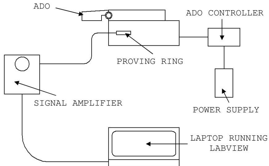
**Figure 5.3 – Test setup for ADO prototype**
