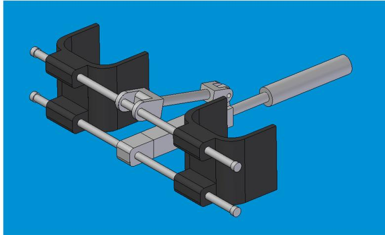
**Figure 4.22 – CAD model of dynamic knee block**
