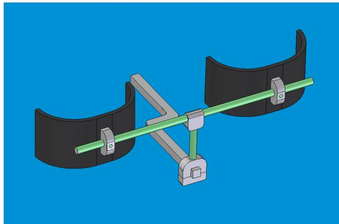
**Figure 4.23 – CAD model of static knee block assembly**
