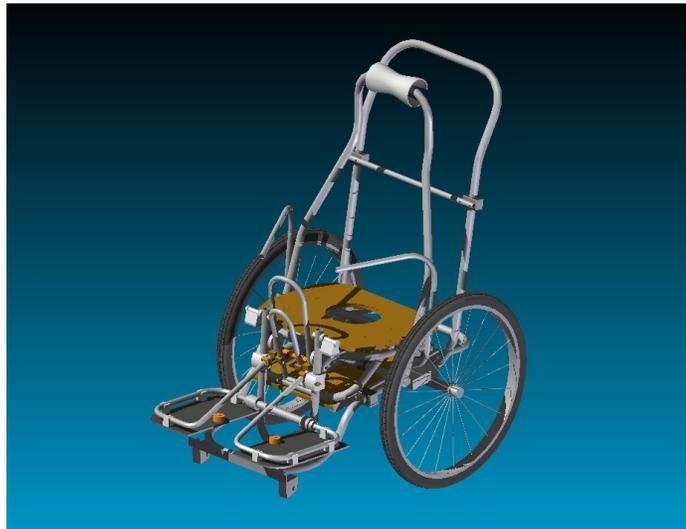
**Figure 4.1 – A fully rendered 3D CAD model of the Meyer adaptive seating system. It is shown here in manual mode and without the custom moulded cushion that the user sits on.**
