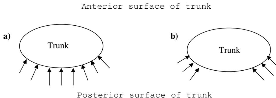
**Figure 4.2 – Forces applied to trunk in a) standard seat and b) Meyer support**
