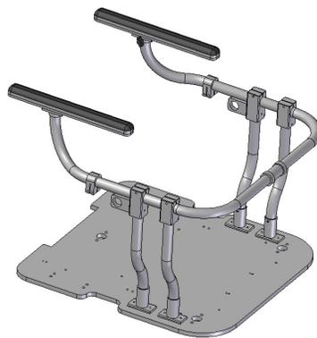
**Figure 4.13 – CAD model of final version of armrest assembly**
