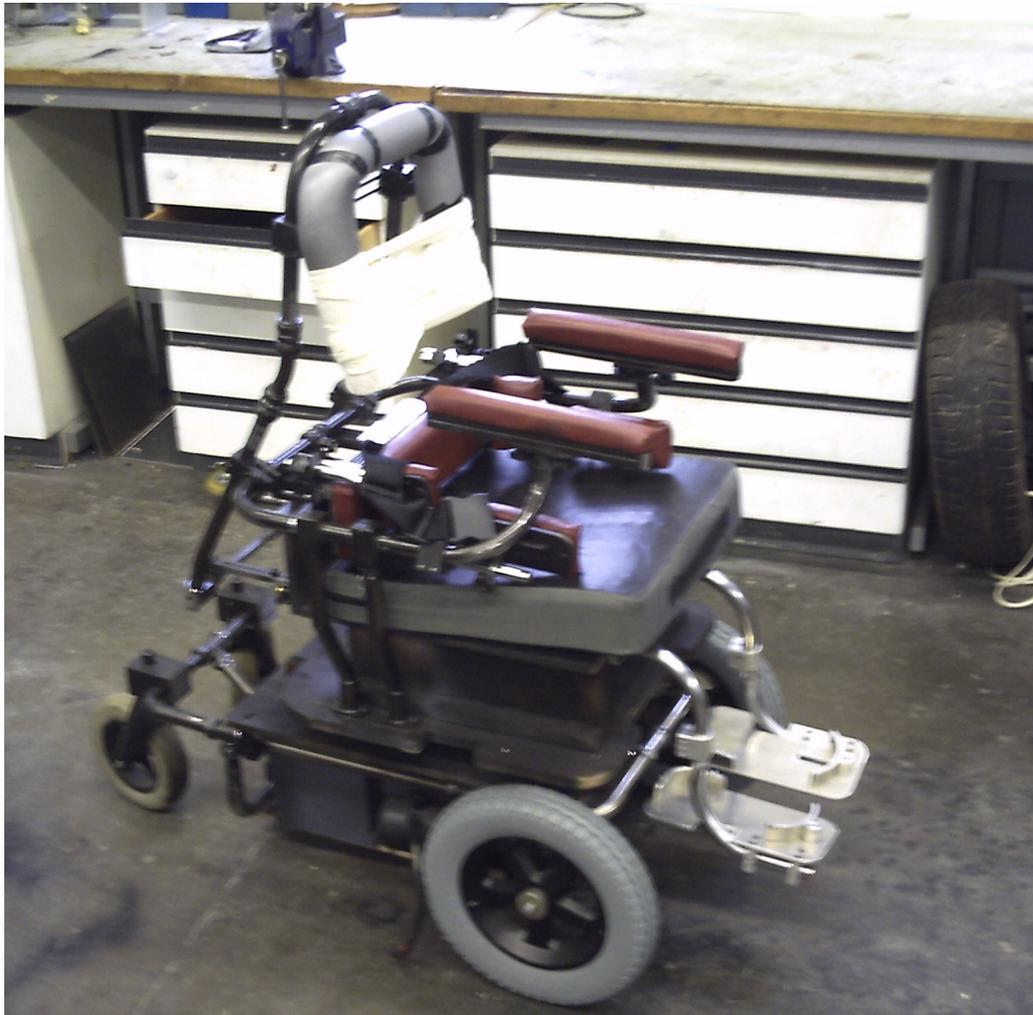
**Figure 4.27 – Prototype of novel adaptive seating system**
