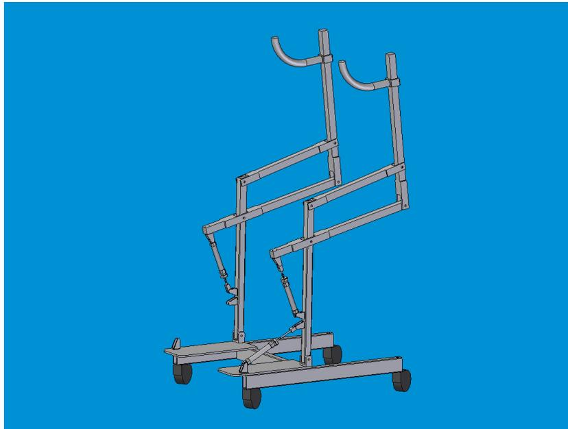
**Figure 4.26 – CAD model of sit-to-stand frame**
