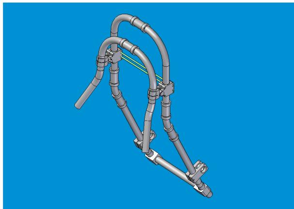
**Figure 4.15 – CAD model of final backrest assembly (prototype version)**
