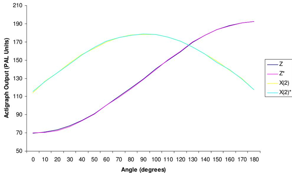
**Figure 6.4 – Results from test 2: rotating actigraph around the Y axis. Z:** output from Z channel from 0 - 180°; **Z\*:** output from Z channel from 180 - 0°; **X(2):** output from X channel from 0 - 180°; **X(2)\*:** output from X channel from 180 - 0°. Data are means taken across three individual trials.
