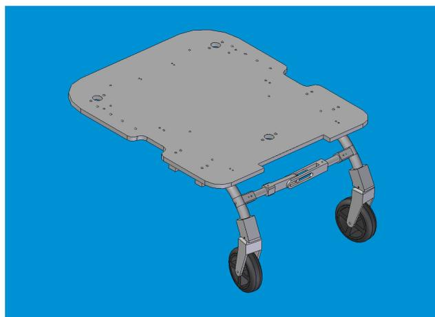
**Figure 4.25 – CAD model of final design for front caster assembly**
