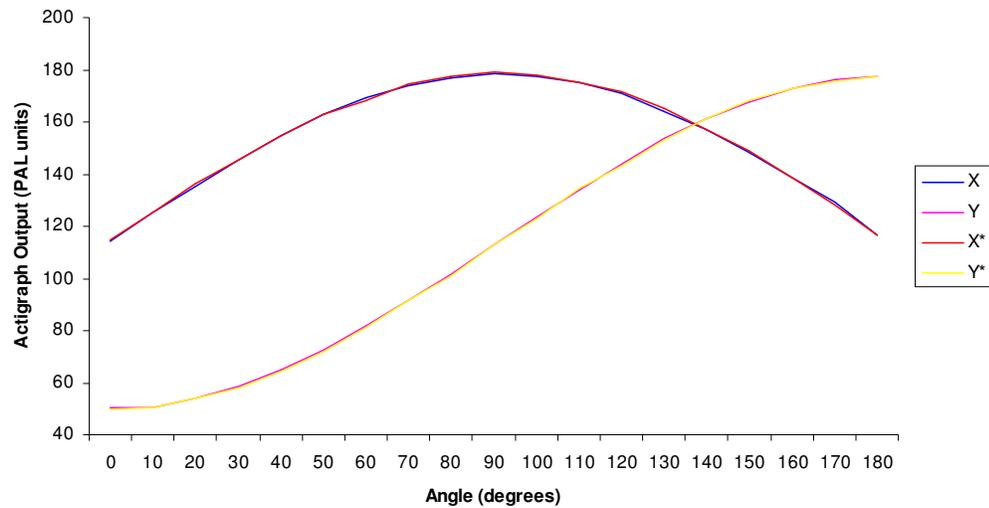
**Figure 6.3 – Results from test 1: rotating actigraph around the Z axis. X:** output from X channel from 0 - 180°; **X\*:** output from X channel from 180 - 0°; **Y:** output from Y channel from 0 - 180°; **Y\*:** output from Y channel from 180 - 0°. Data are means taken over three individual trials.
