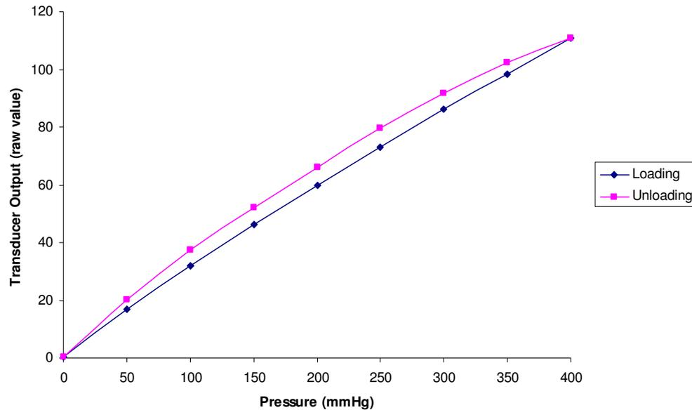
**Figure 7.6 – Graph showing hysteresis effects on transducer output. Values are means taken across the constant load period and across all three tests.**
