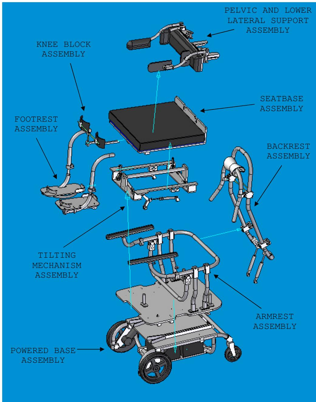
**Figure 4.4 – Final design exploded assembly view**
