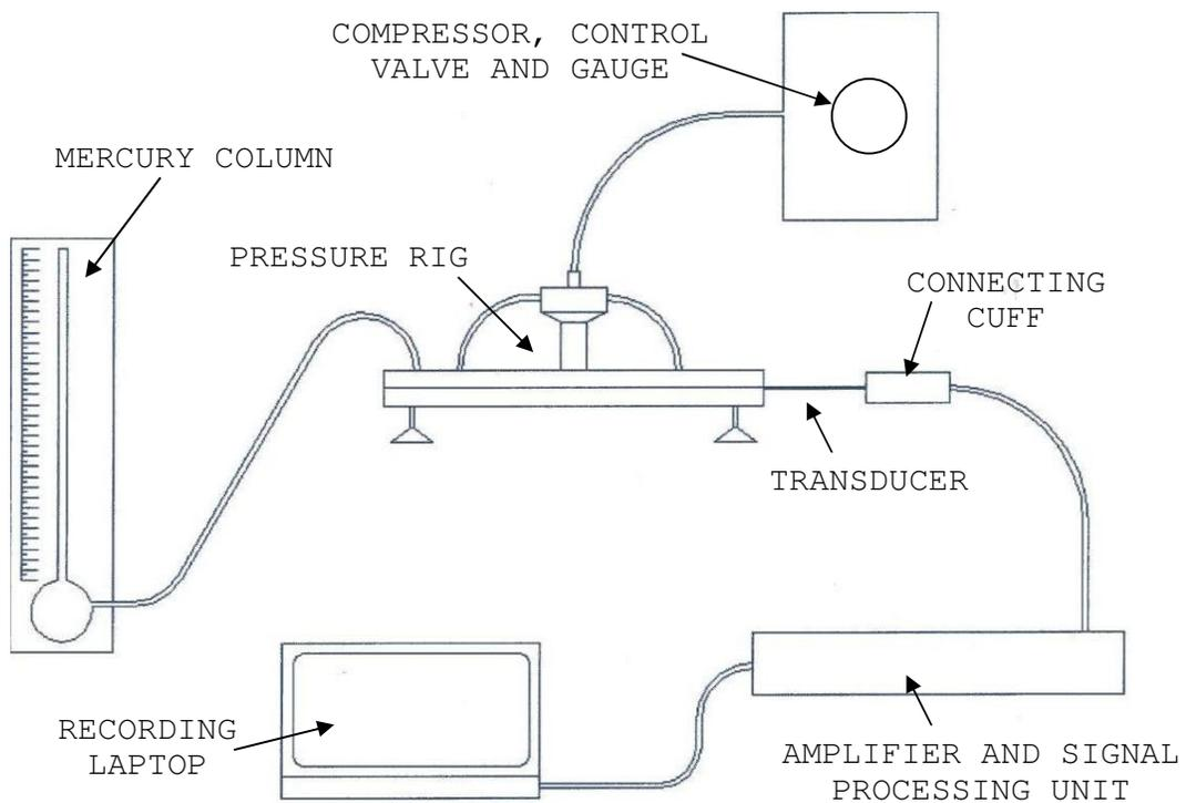
**Figure 7.1 – Calibration and testing set up**
