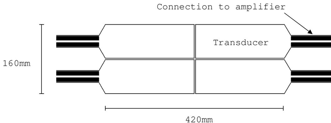
**Figure 7.2 – Pressure transducer set up for seating tests**
