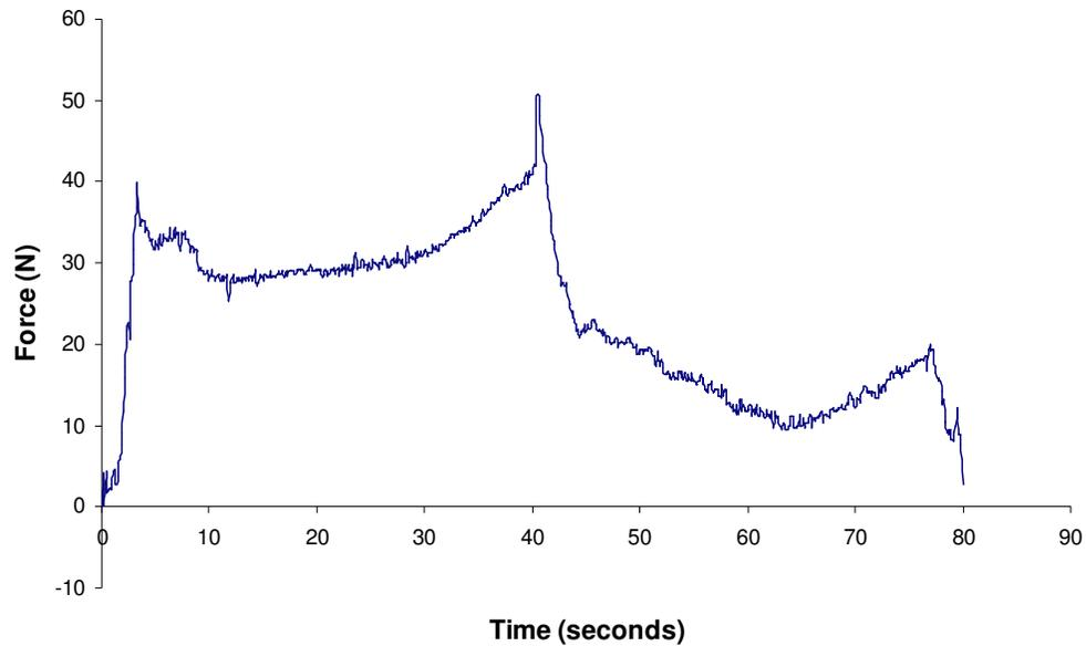
**Figure 5.4 – Typical force profile from ADO (test 1). From 0 to 40 seconds linear actuator is moving to compress the gas spring; from 40 to 80 seconds the actuator is reversing and the cylinder is being decompressed**
