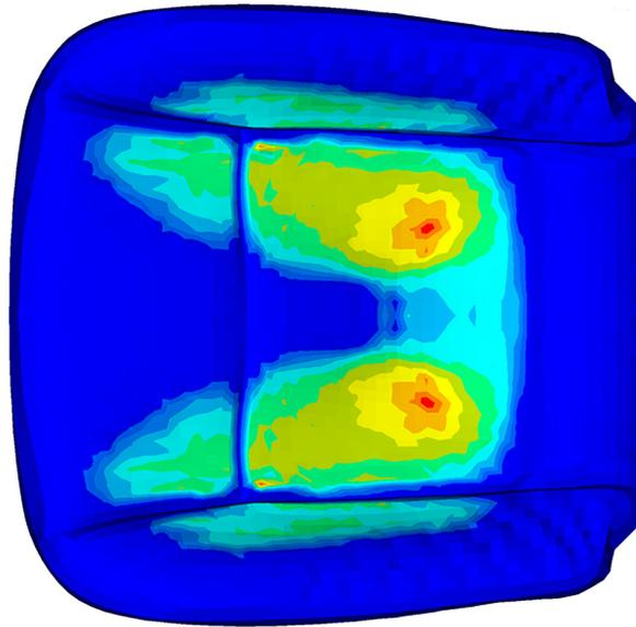
**Figure 2.5 – A typical pressure distribution pattern at the interface between subject and seat ([www.woelfef.de](http://www.woelfef.de)).**
