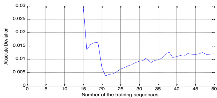
Figure 6.4: Absolute Deviation between the original and estimated value of F_1 = 0.03 according to the number of the training sequences.
