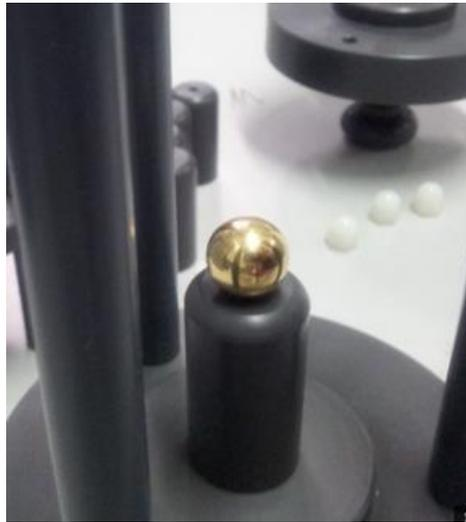
**Figure 3-22.** Ground brass sphere electrode.
