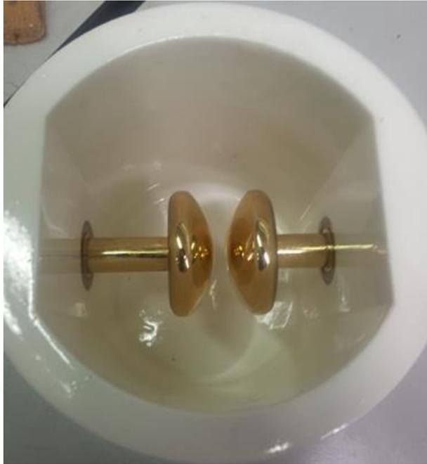
**Figure 3-12.** Practical spherically capped electrode.
