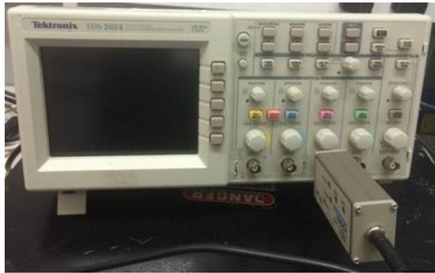
**Figure 3-15.** Tektronix digitising oscilloscope.
