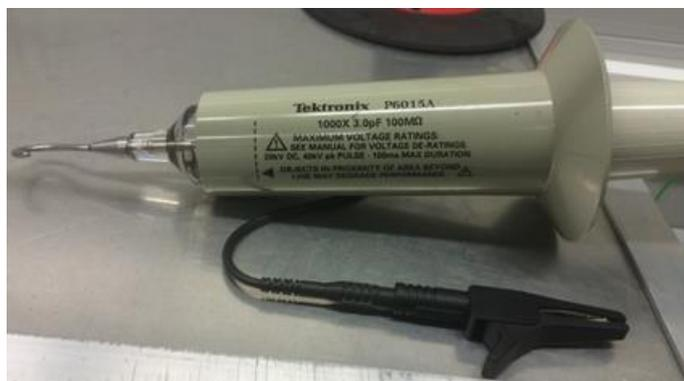
**Figure 3-14.** Tektronix P6015A HV probe.
