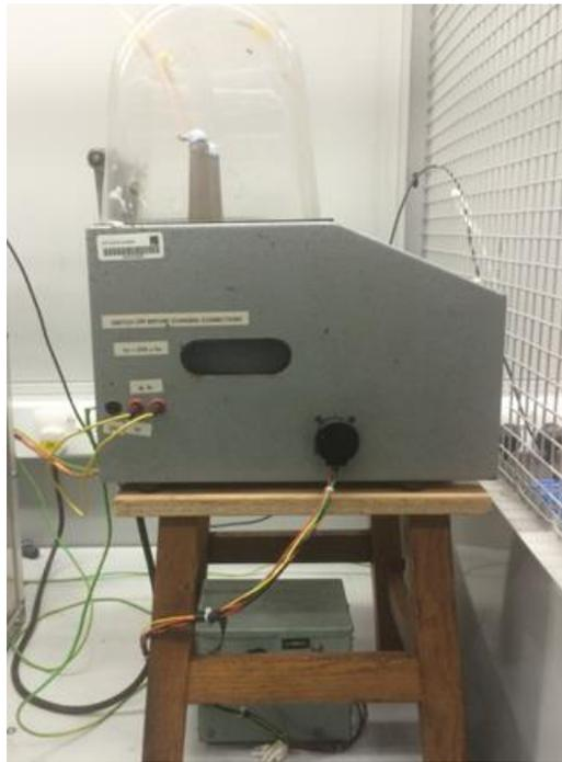
(a): AC Foster breakdown test apparatus.
