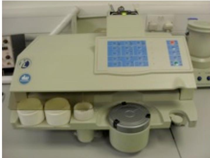
**Figure 3.9:** *The automated spiral plater (Don Whitley Scientific, Shipley, UK). The agar plate is placed on the central rotating disk, and liquid samples drawn under negative pressure and distributed over the agar surface: linear distribution for spread plates and logarithmic distribution for spiral plates.*
