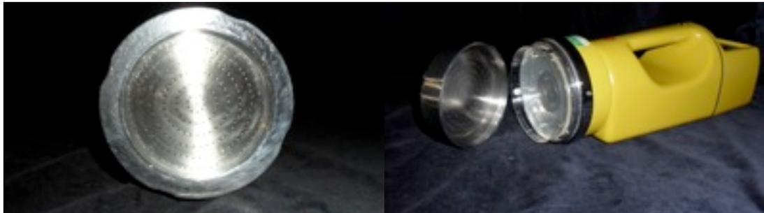
**Figure 3.4:** SAS Super 180 air sampler head (left) with 219 machine-perforated holes, and placement of agar plate within air sampler (right).
