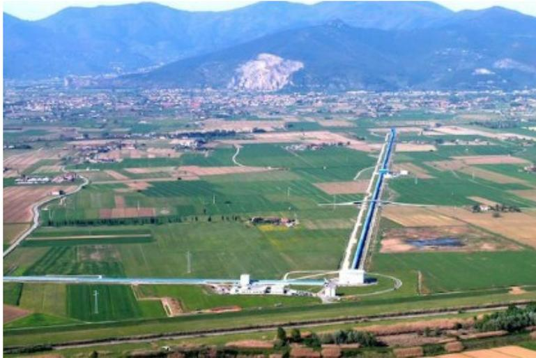
Figure 1.5: Advanced Virgo detector. The gravitational wave detector consists of a Michelson interferometer with arm lengths of 3 km. The site is located in Cascina, Italy. Photograph taken from [44].
