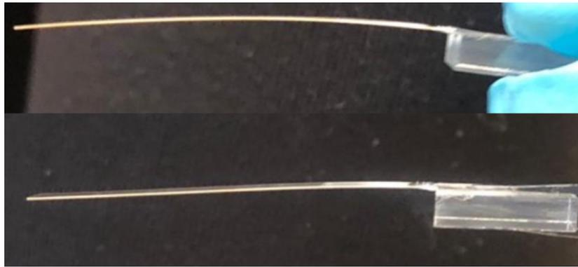
Figure 5.10: Side-view images illustrating the changes in thin film stress on the silica cantilever resonators. The upper image represents the stress on the cantilever due to the deposited coating with no heat treatment. The bottom image illustrates the change in stress after a heat treatment at  $500^\circ\text{C}$ .
