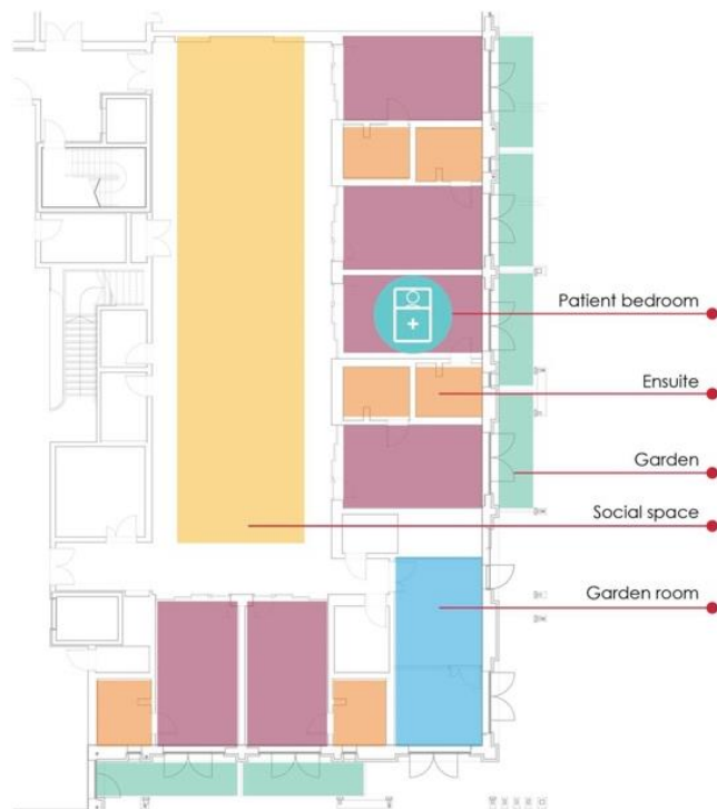
Figure 8-3 Diagram of all important elements of the Sengetun layout within one of the units.
