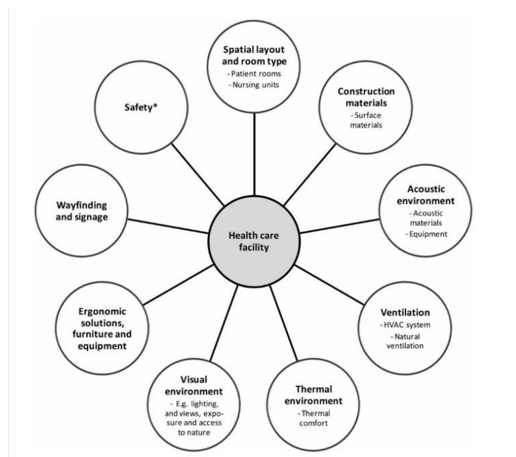
Figure 3-6 Physical design features identified through a literature review to be of important within healthcare facilities (Salonen et al, 2013, p5).
