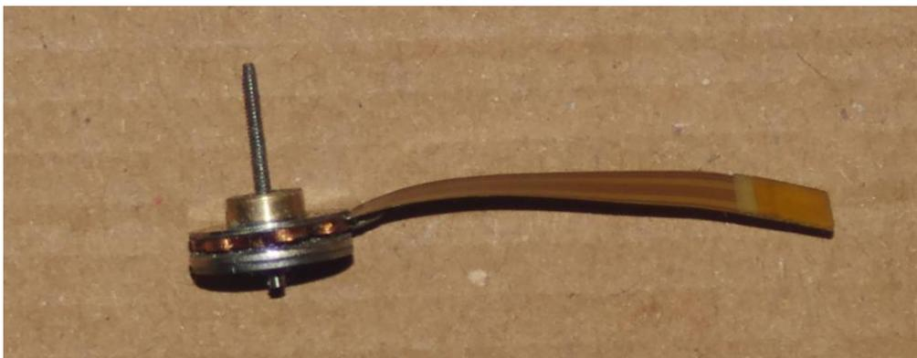
**Figure 28.** Modified Maxon DC motor
