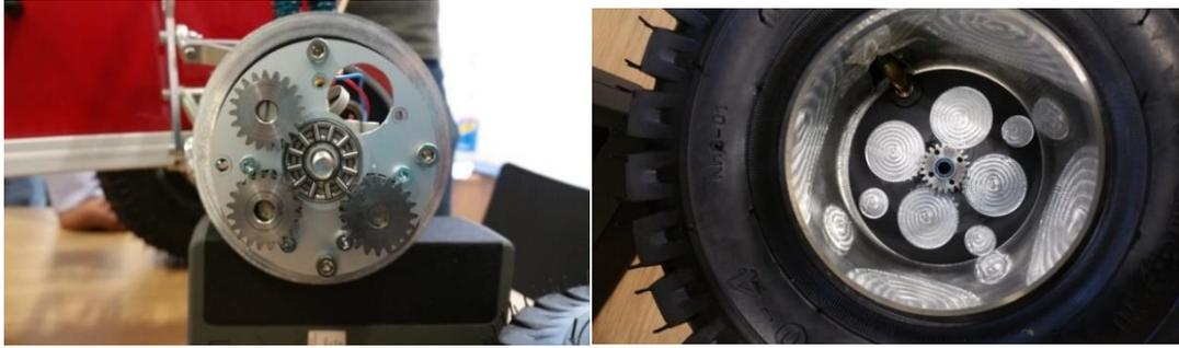
Figure 52. Wheel hub transmission of the first-generation rover
