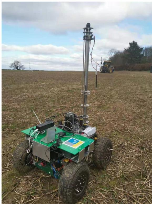
Figure 2. AgriRover, prototype with soil sampling and analysis system in a field
