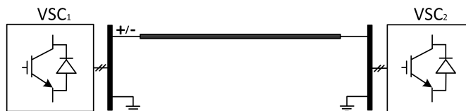
Figure 2.4: Asymmetric monopole - ground return.
