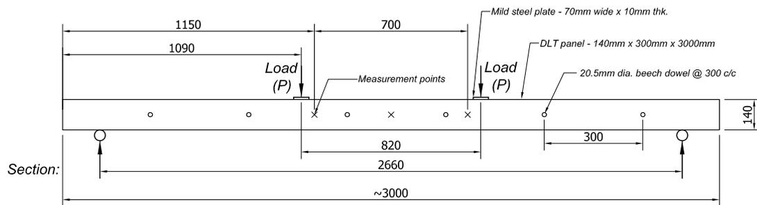
Figure 8-7: Full scale DLT panel four point bending test.
