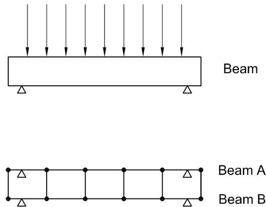
Figure 4-9: Shear analogy grid, adapted from Natterer and Weinand (2008).
