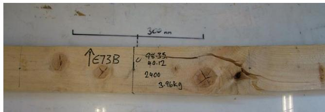
Figure 6-4: Example of a knotty specimen
