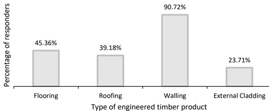
**Figure 2-10: Application suitability of a DLT product according to survey responders.**
