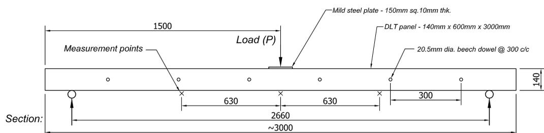
Figure 8-5: Full-scale DLT panel three point bending test arrangement.
