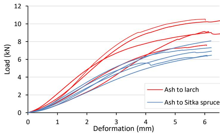
**Figure 6-38 Combined perpendicular embedment – Ash**
