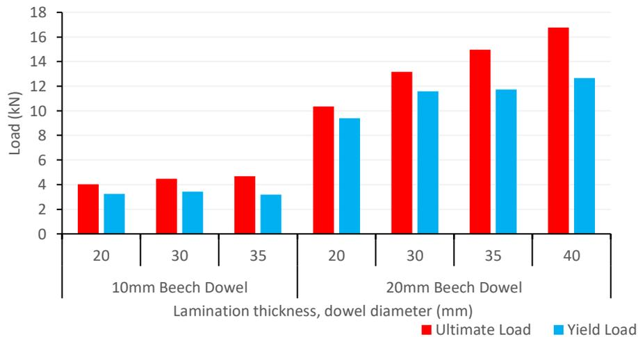
Figure 7-12: Comparison of the mean ultimate and yield load of beech dowels in UK Sitka spruce.
