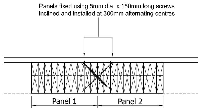
**Figure 9-6: Example of mechanical joint between DLT panel sections.**
