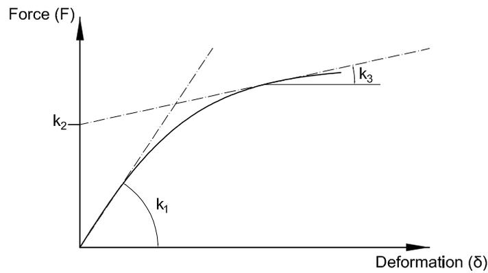
Figure 5-14: Bi-exponential load diagram, adapted from Natterer and Weinand (2008).
