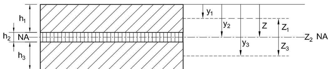
**Figure 8-18: Shear Analogy layers**
