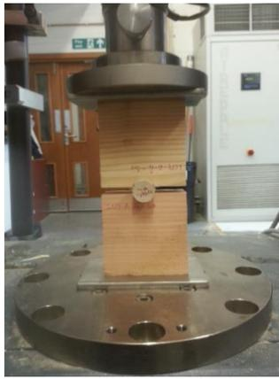
Figure 6-33: Combined embedment test.
