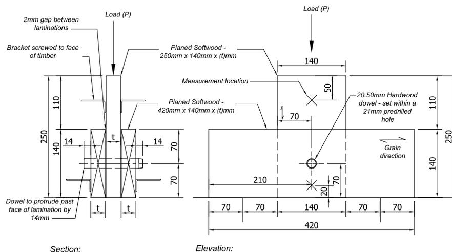
Figure 7-6: Perpendicular to the grain double shear plane testing.
