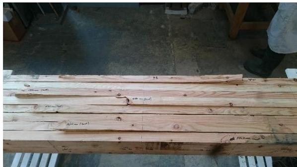
**Figure 8-11: Measuring failure positions in laminations**
