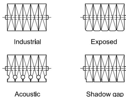
Figure 2-3: Some example finishes of a DLT panel.
