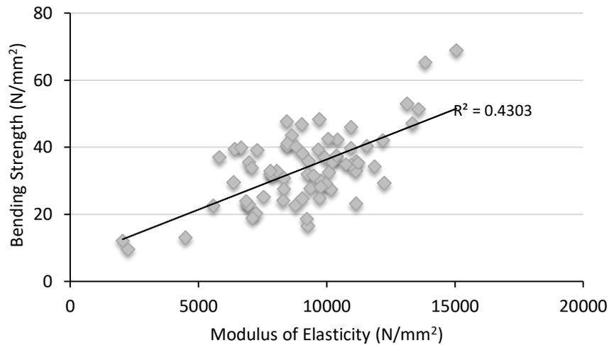
Figure 6-3: Strength vs. Stiffness of UK grown Sitka spruce.
