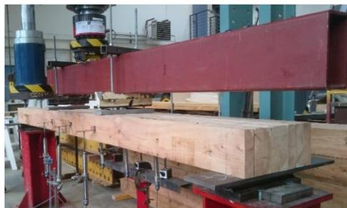
Figure 8-8: Four point bending set-up.
