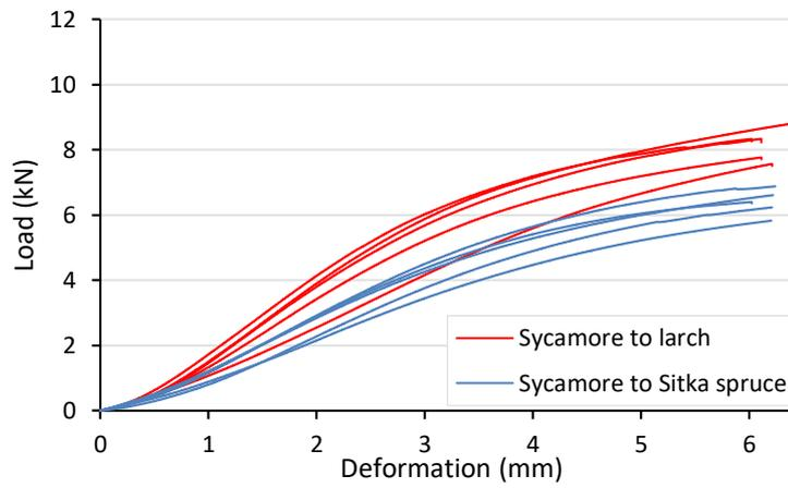
**Figure 6-41: Combined perpendicular embedment - Sycamore**
