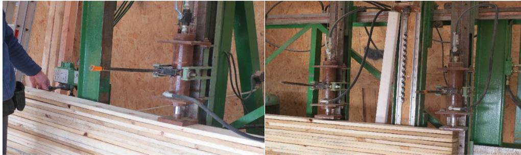
**Figure 8-3: Clamping and drilling of laminations.**
