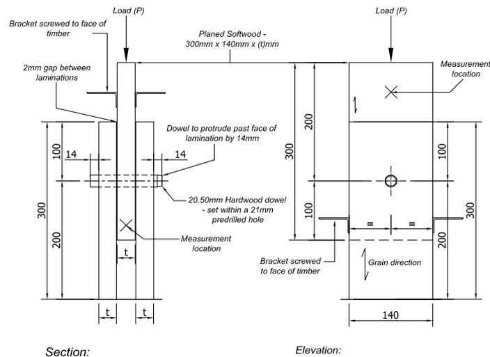
Figure 7-5: Parallel to grain double shear plane tests.
