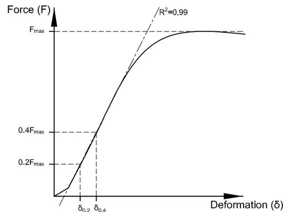
**Figure 7-7: Derivation of initial stiffness**
