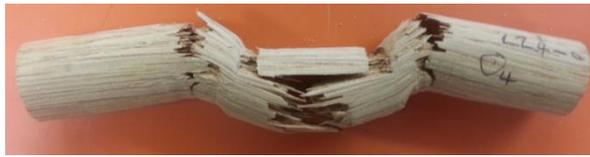
**Figure 7-45: Three hinge failure.**
