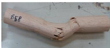
Figure 7-16: Irregular formation of hinges within in Beech dowel during  $V_d$  failure.
