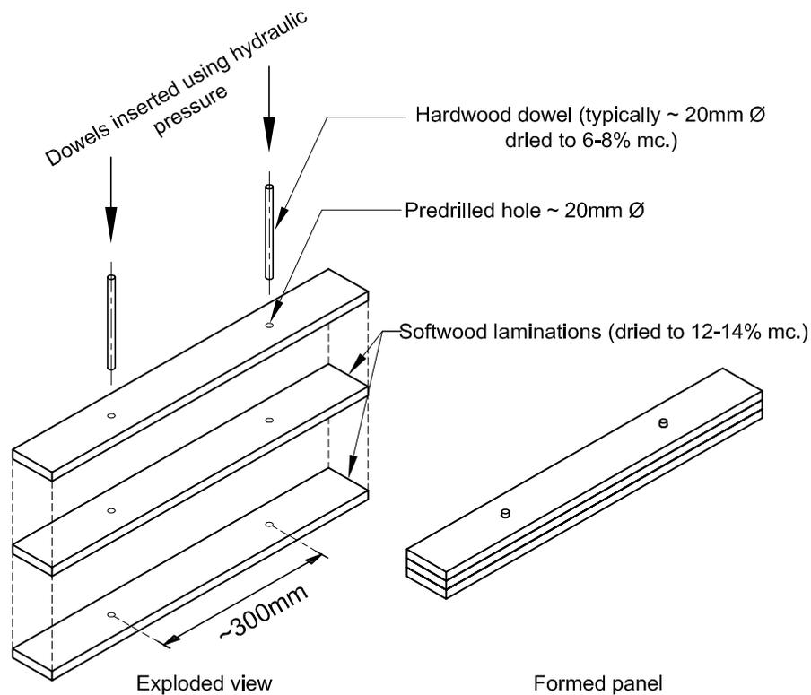
**Figure 2-1: Formation of a DLT panel.**
