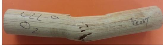
**Figure 7-46: Brittle bending failure.**
