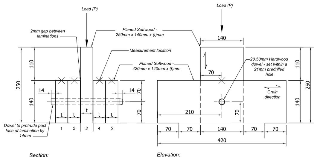
**Figure 7-34: Additional shear plane tests perpendicular to the grain.**
