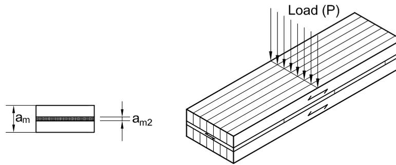
Figure 4-8: Idealised cross-layered DLT panel.
