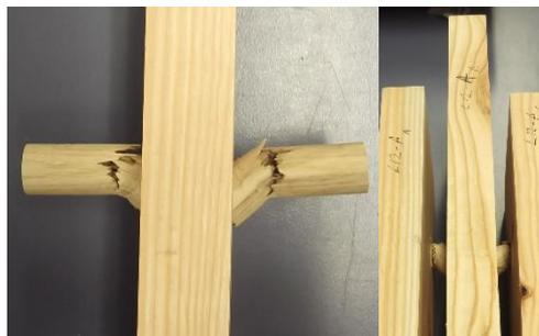
**Figure 7-44: Cross grain shear failure of hardwood dowels.**
