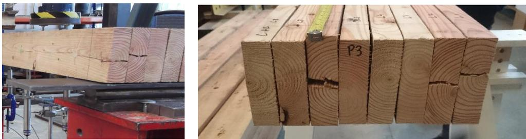
Figure 8-16: Examples of splitting perpendicular to the grain.
