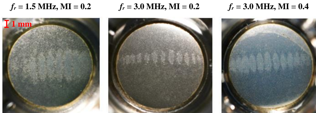
Figure 6-9 Macro Imaging of the Cell Monolayers After Sonication
