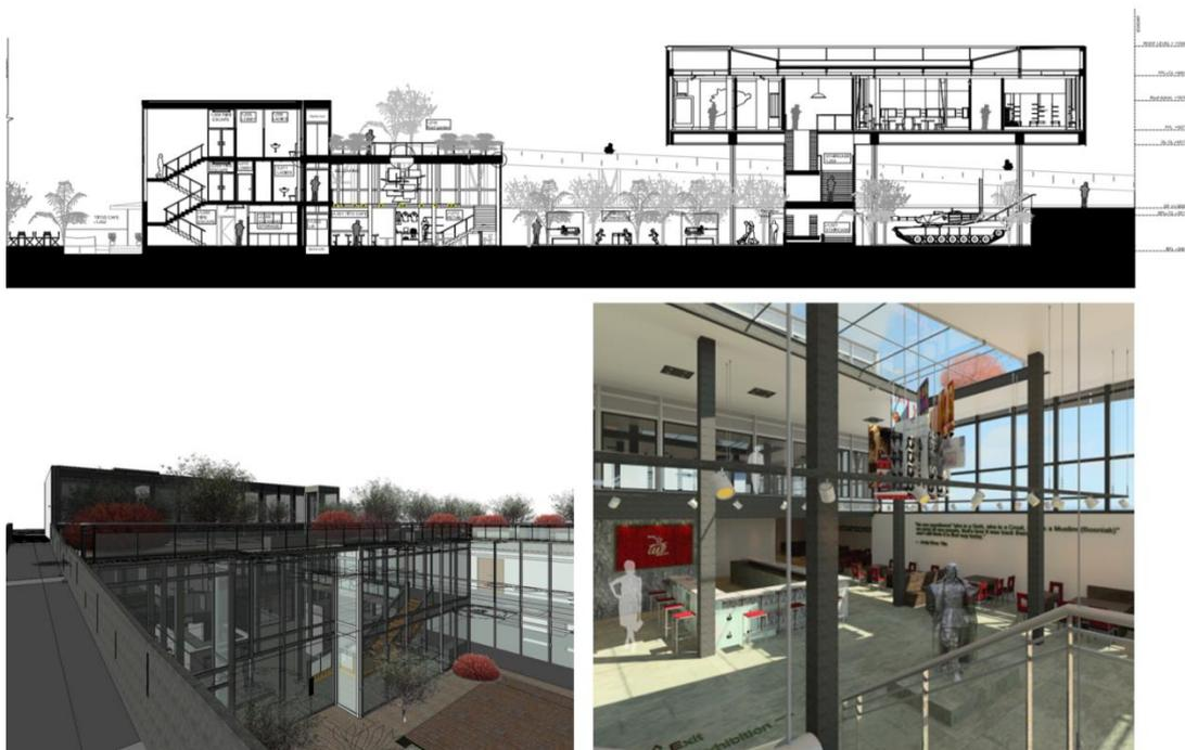
**Fig.7.15** Design Studio Group Project 2013-14, with History Museum of BiH, April 2014; (anti-clockwise from top) Longitudinal Section with Courtyard Extension; View to Courtyard Extension from the roof above Ground level; Interiors of the Courtyard Extension (© Selma Harrington).
