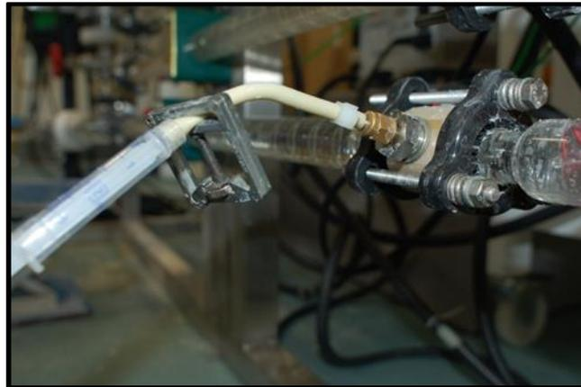
**Figure 4.7: COBC tracer injection port.** Photograph of the COBC setup showing the injection port. A syringe is connected to the port via marprene tubing.
