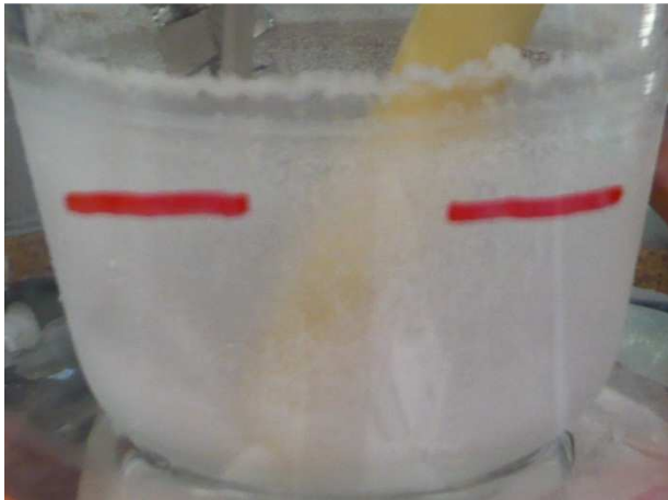
Figure 9.5-14: Bottom view into crystallisation vessel without hot wall or ultrasound indicates fouling on vessel walls
