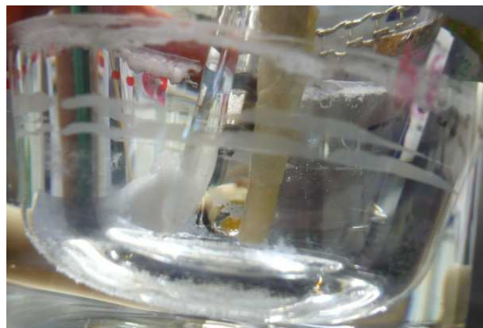
Figure 9.5-21: Bottom view into crystallisation vessel hot wall + ultrasound after run time of 100 min.
