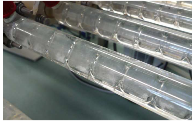
Figure 10.4-22: Sedimentation in COBC indicating poor mixing hydrodynamics or agglomerated heavy crystals
