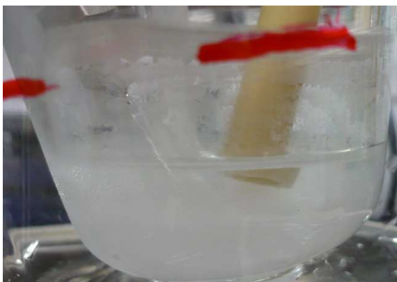
Figure 9.5-18: Bottom view into crystallisation vessel with heated walls. Significantly reduced, uneven fouling in hot wall cold bulk set up
