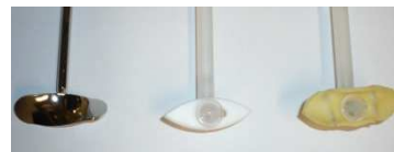
Figure 5.3-4: Stainless steel, PTFE and self-built Marprene stirrer
