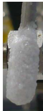
Figure 9.5-17: Fouling on thermocouple
