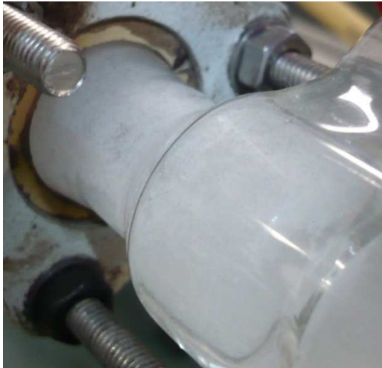
Figure 10.4-21: Fouling in COBC under conditions where the Alpha form nucleates in the presence of Beta seeds
