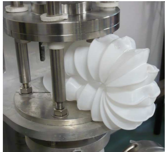
Figure 10.4-23: Buckled bellow after the COBC was blocked due to excessive fouling along the rig
