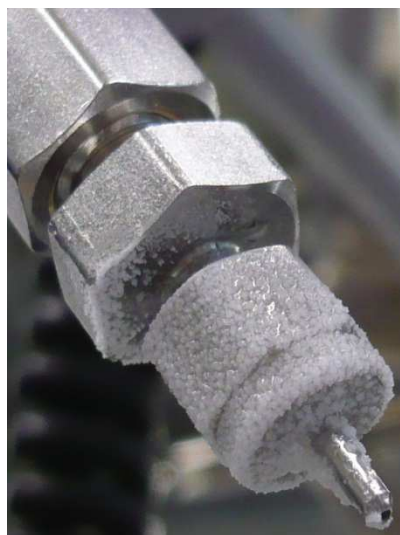
Figure 9.5-19: Fouling on injection nozzle
