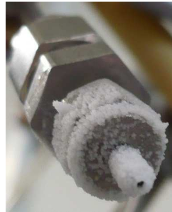
Figure 9.5-15: Fouling on injection nozzle
