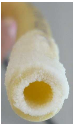
Figure 9.5-16: Fouling on outlet tube
