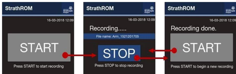
**Figure 3. 5** Graphical User Interface of Smartwatch Application showing interactions between each screen.
