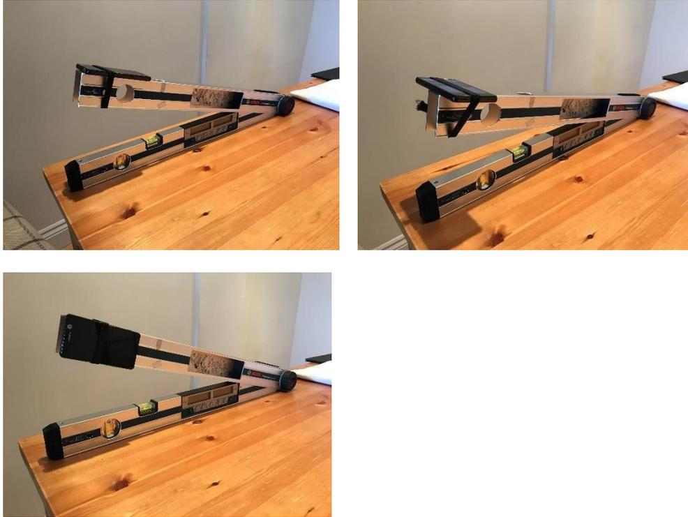
**Figure 4. 1** Bosch GAM 270 MFL Professional Angle measurer with smartphone attached in three orientation to measure a) rotation about pitch axis, b) rotation about roll axis, c) rotation about yaw axis
