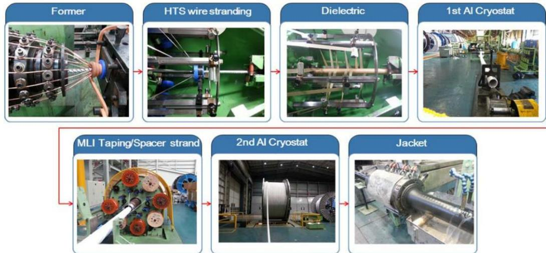
Figure 3.15 Fabrication of HTS DC cable by the manufacturer, LSC [148]
