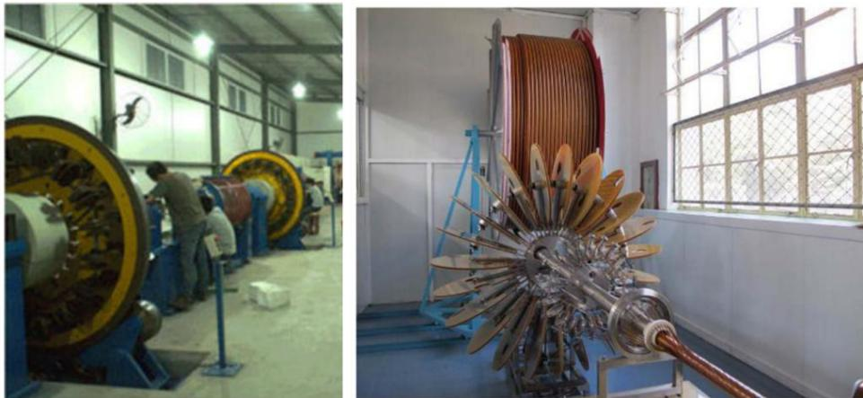
Figure 3.14 Fabrication of the HTS cable core [146], [147]
