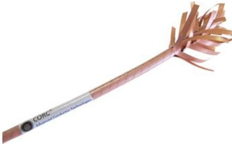
Figure 3.5 CORC cable 7 mm in diameter with 30 tapes [123]
