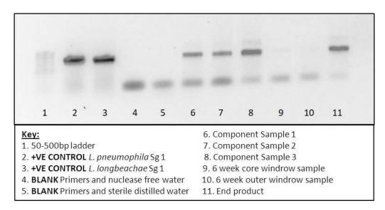
Figure 6.4: An electrophoresis agarose gel image of JP PCR products from the green waste composting site
