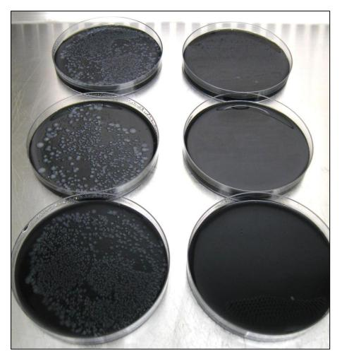
Figure 6.3: Triplicate samples on BCYE-α agar after eight days incubation in humid conditions at 37°C. Left-hand side plates represent samples from week six taken from the outer layer of the windrow. Right-hand side plates represent samples from week six taken from the core of the windrow.
