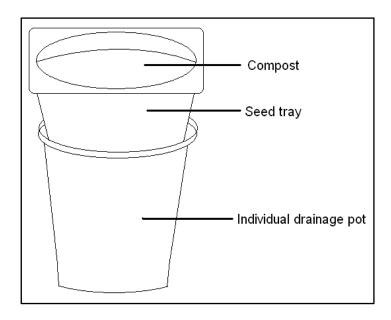
Figure 5.2 : Individual drainage system for compost batches used in NSGH to prevent cross-contamination through water flow.
