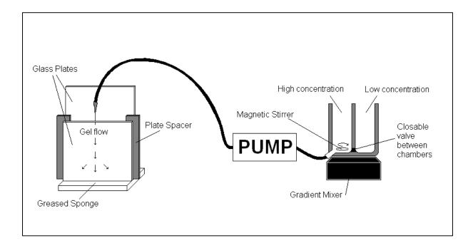
Figure 4.1: A simplified diagram of DGGE gel formation equipment
