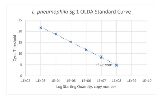
Figure 4.6 Standard Curve for *L. pneumophila* Sg 1 OLDA. Slope = -3.394. Efficiency = 97.08%.
