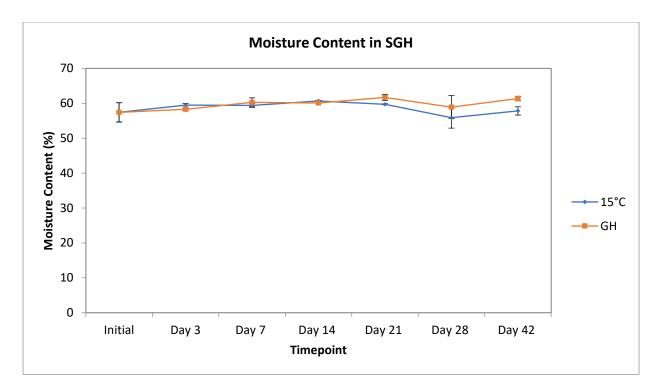
Figure 5.3: Moisture content of control compost (Batch 1) measured at different time points during the spiked greenhouse experiment
