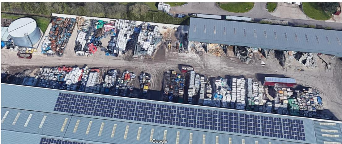
Figure 3-4. A 3D view of a recycling centre. On the left we can see a tank for liquid storage that could float/collapse under floods/debris impact and release the containment. The storing of waste is mostly directly on the ground, and the rain coverage on the right of the picture for selected types of waste won't protect against flooding. ©2022 Google, Imagery ©2022 CNES / Airbus, Getmapping plc, Infoterra
