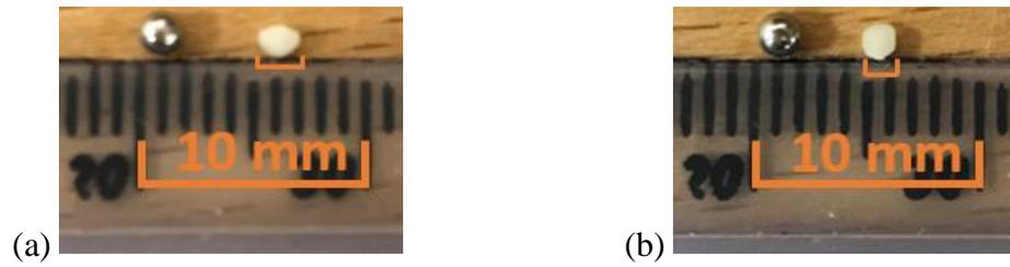
*Figure 6.28 Illustration of the size and shape of the TMM particle. The 2 mm ball bearing is used as a reference.*
