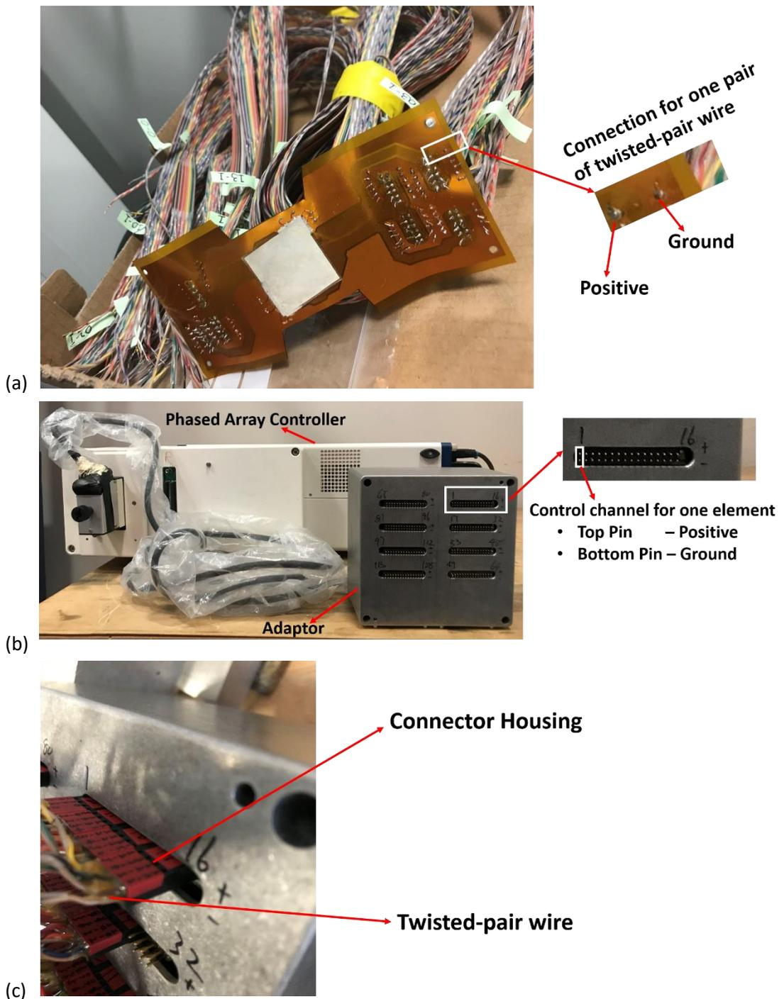
Figure 4.20 (a) Illustration of how the twisted-pair wires are connected to the PCB. (b) Illustration of the adaptor and the phased array controller. (c) Illustration of how the twisted-pair wires are connected to the adaptor through external connector housings.
