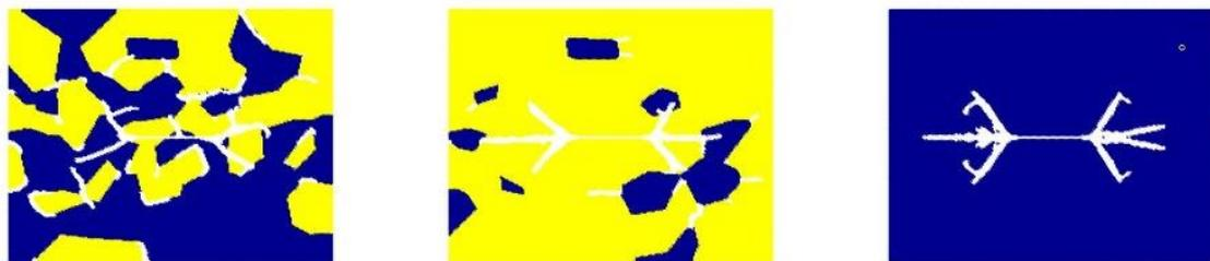
(b) Crack propagation showing the material composition (blue represents silicon carbide).
