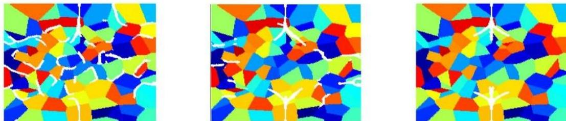
(a) Crack propagation showing the distribution of crystals.
