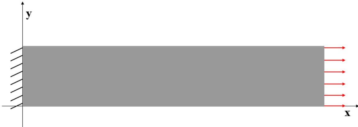
**Figure 5.8** The loading and boundary conditions of Case 2
