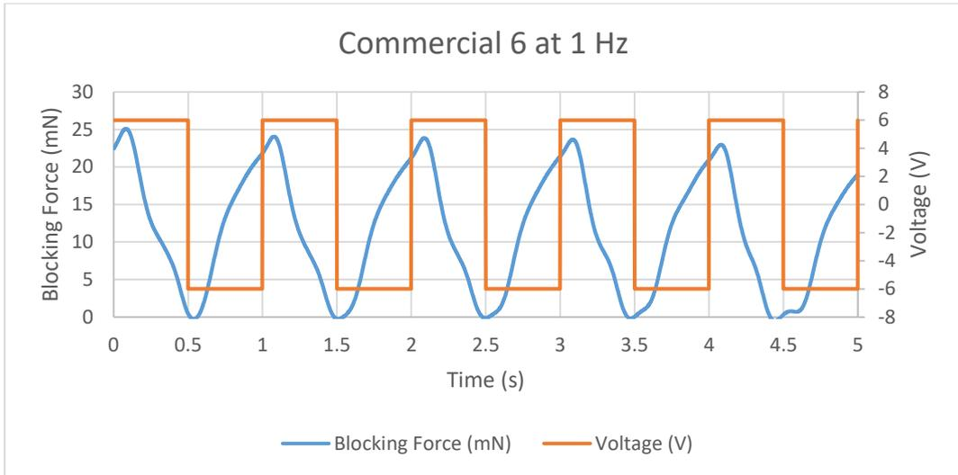
Figure 11.59 Blocking Force of Commercial 6 IPMC at 1 Hz
