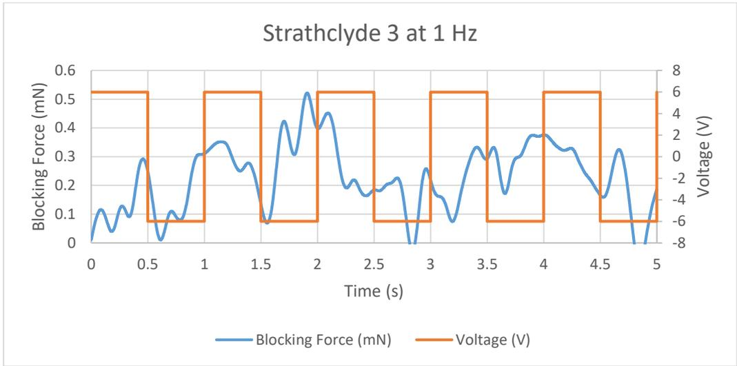
Figure 11.71 Blocking Force of Strathclyde 3 IPMC at 1 Hz
