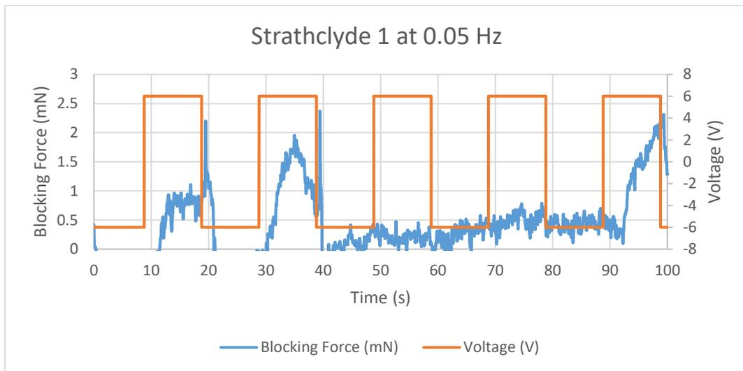
Figure 11.61 Blocking Force of Strathclyde 1 IPMC at 0.05 Hz
