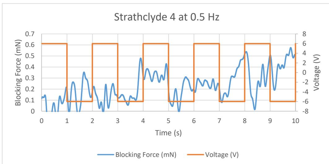
Figure 11.74 Blocking Force of Strathclyde 4 IPMC at 0.5 Hz
