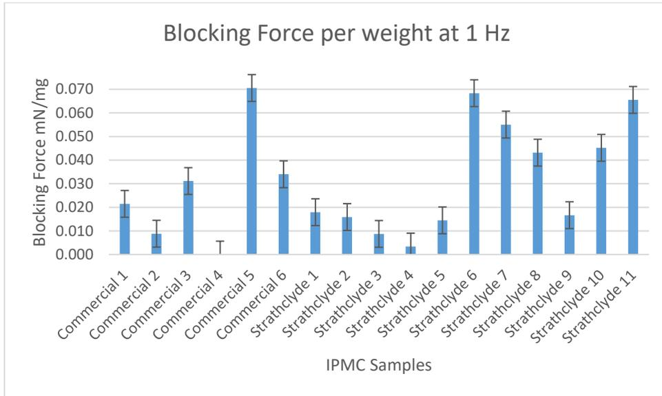
Figure 4.90 Maximum blocking force per weight at 1 Hz
