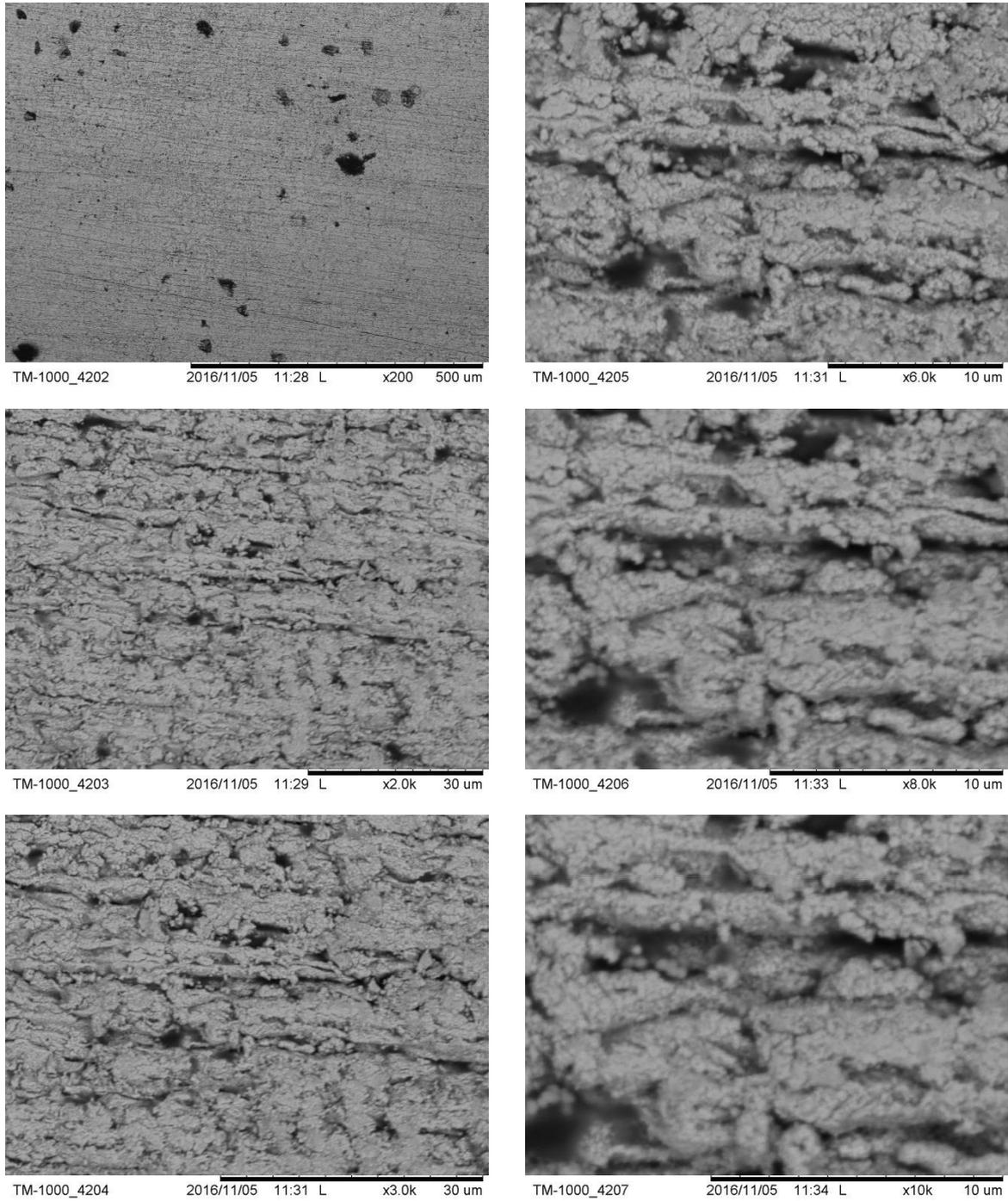
**Figure 4.4 SEM images of the Commercial 5 IPMC**
