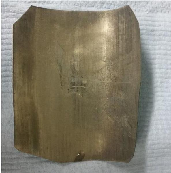
Figure 3.19 Nafion 117 membrane after the Secondary Plating stage
