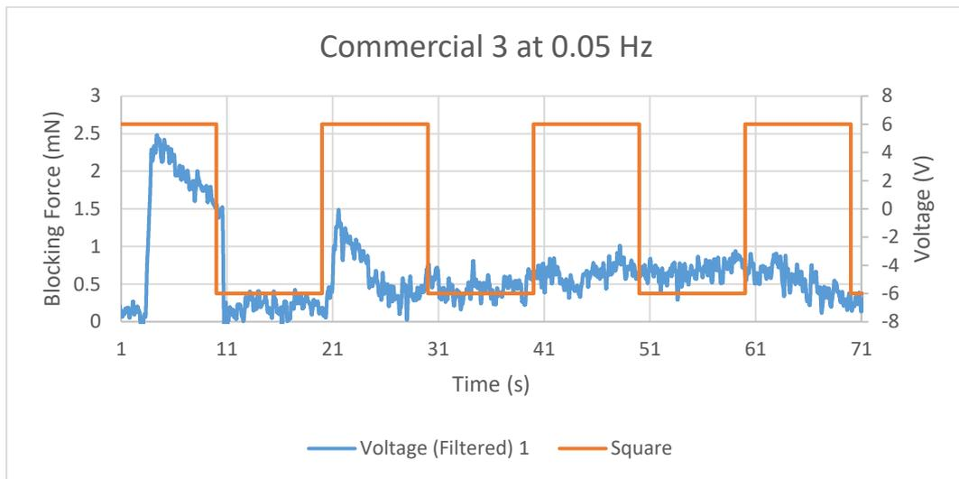
Figure 11.47 Blocking Force of Commercial 3 IPMC at 0.05 Hz
