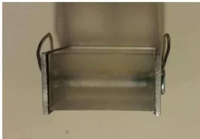
Figure 4.25 Surface resistance testing square
