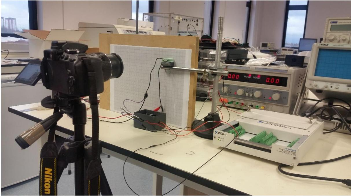
Figure 4.55 The complete experiment setup for displacement test
