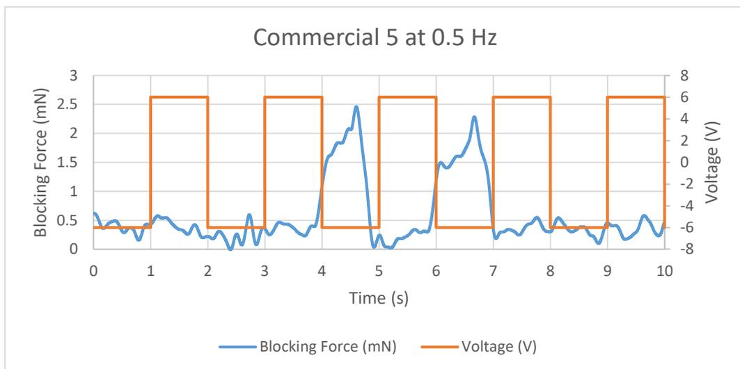
Figure 11.54 Blocking Force of Commercial 5 IPMC at 0.5 Hz
