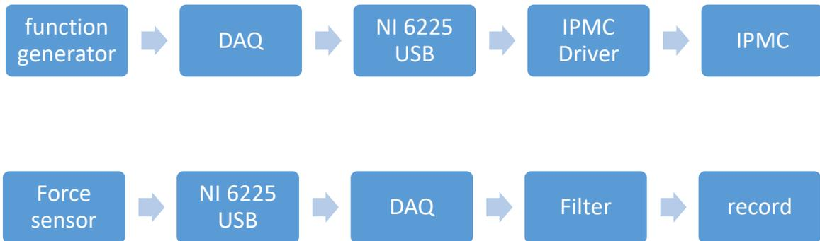
Figure 4.74 Block diagram of the blocking force test
