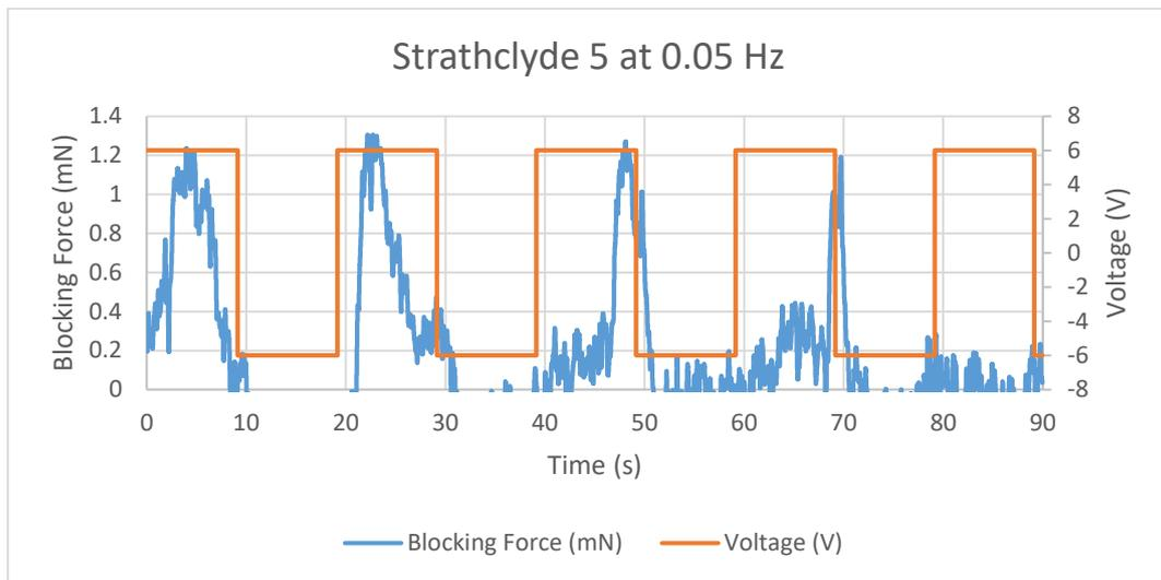
Figure 11.77 Blocking Force of Strathclyde 5 IPMC at 0.05 Hz
