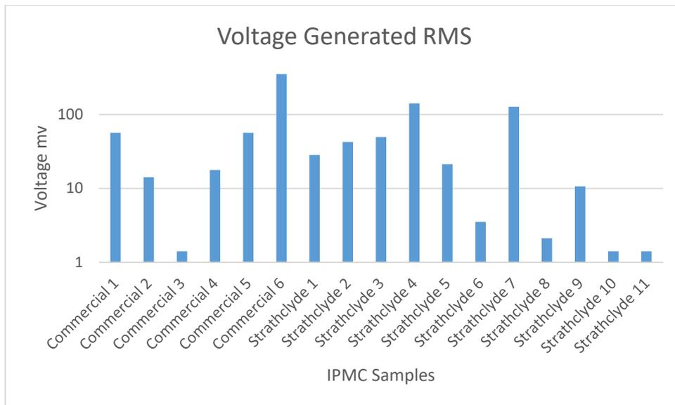
Figure 5.13 RMS voltage generated from all IPMCs
