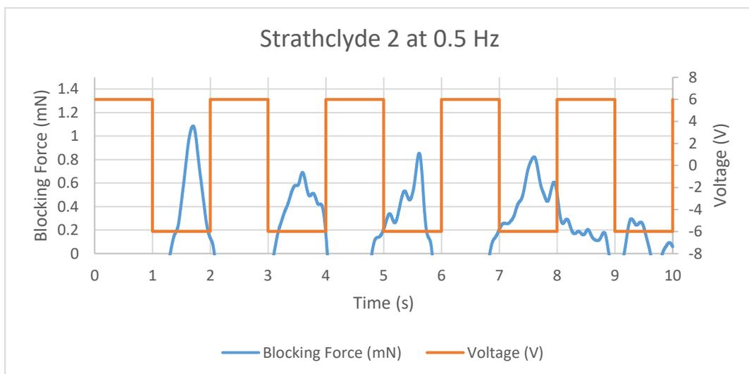
Figure 11.66 Blocking Force of Strathclyde 2 IPMC at 0.5 Hz
