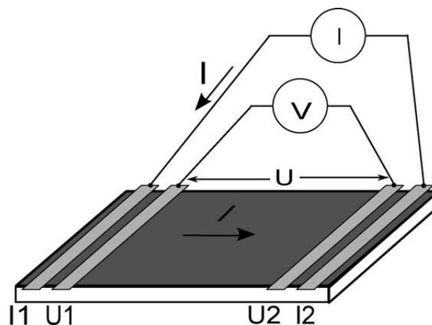
Figure 4.23 Four-point surface resistivity device (Punning, Kruusmaa et al. 2007)
