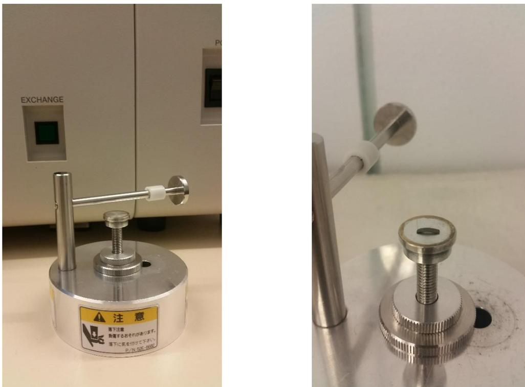
Figure 4.2 The sample holder on the left and the sample ready for scanning on the right.
