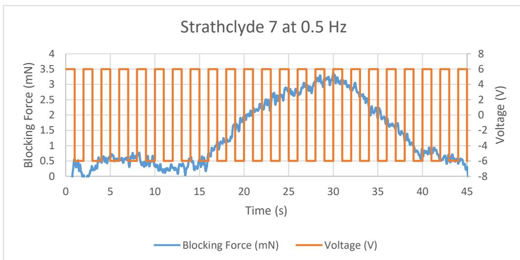
Figure 11.86 Blocking Force of Strathclyde 7 IPMC at 0.5 Hz
