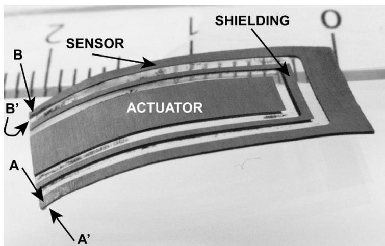
Figure 5.4 Self-sensing IPMC actuator (Kruusamäe, Brunetto et al. 2010)
