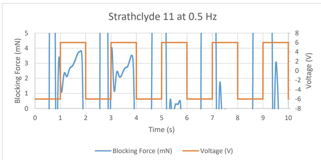
Figure 11.101 Blocking Force of Strathclyde 11 IPMC at 0.5 Hz
