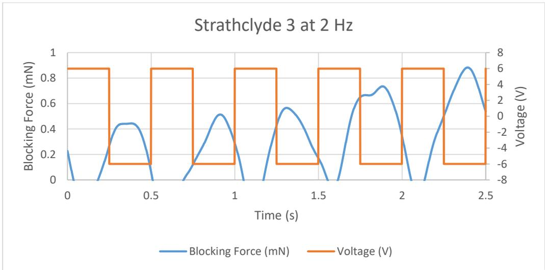
Figure 11.72 Blocking Force of Strathclyde 3 IPMC at 2 Hz
