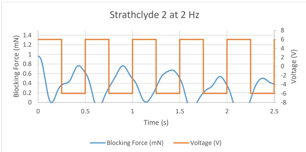
Figure 11.68 Blocking Force of Strathclyde 2 IPMC at 2 Hz
