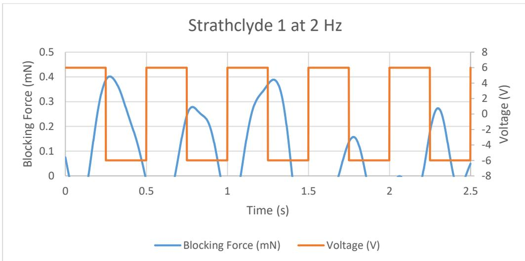
Figure 11.64 Blocking Force of Strathclyde 1 IPMC at 2 Hz
