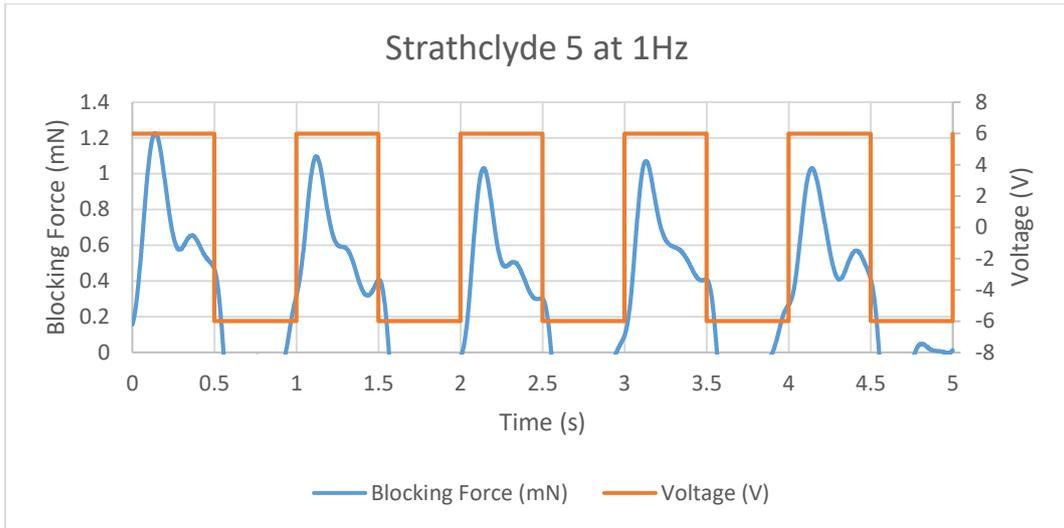
Figure 11.79 Blocking Force of Strathclyde 5 IPMC at 1 Hz
