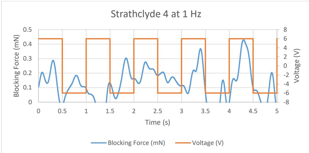
Figure 11.75 Blocking Force of Strathclyde 4 IPMC at 1 Hz
