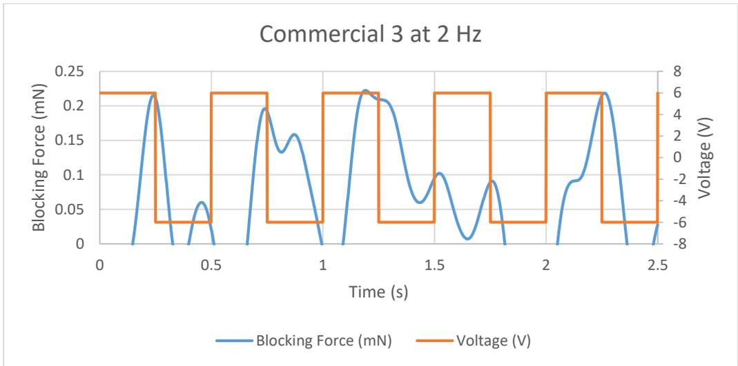
Figure 11.50 Blocking Force of Commercial 3 IPMC at 2 Hz
