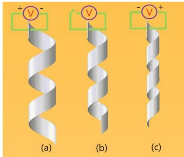
Figure 2.13 IPMC Helical Stent (Li, Kim et al. 2011)
