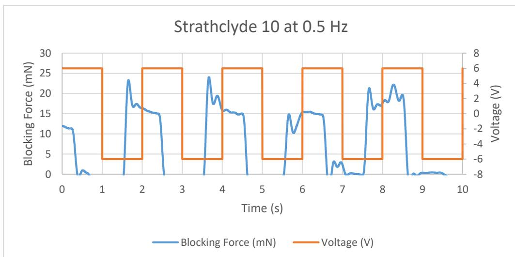
Figure 11.97 Blocking Force of Strathclyde 10 IPMC at 0.5 Hz
