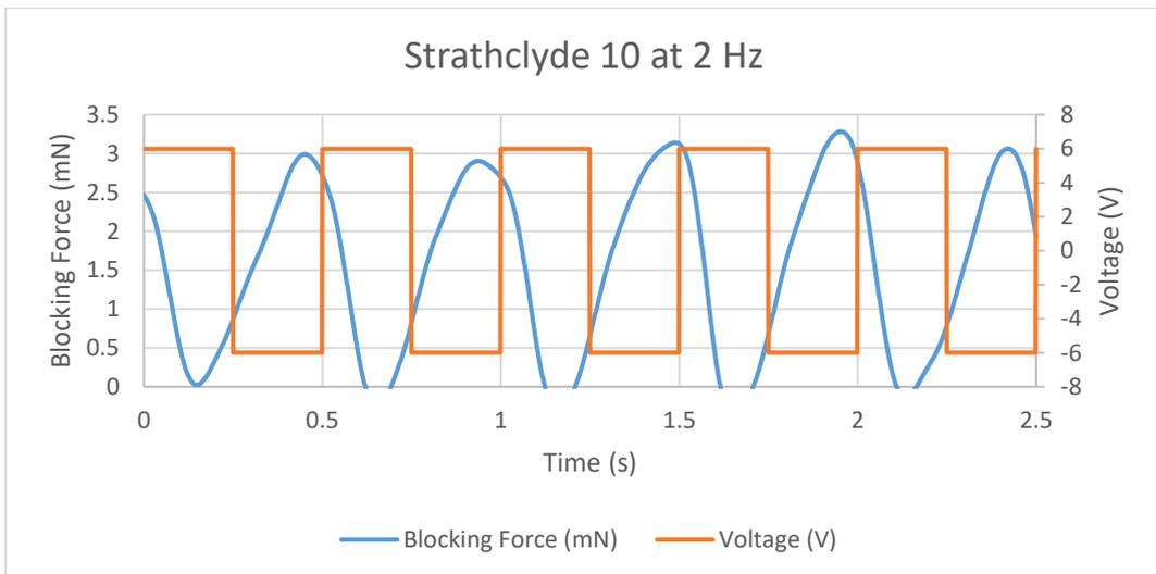
Figure 11.99 Blocking Force of Strathclyde 10 IPMC at 2 Hz
