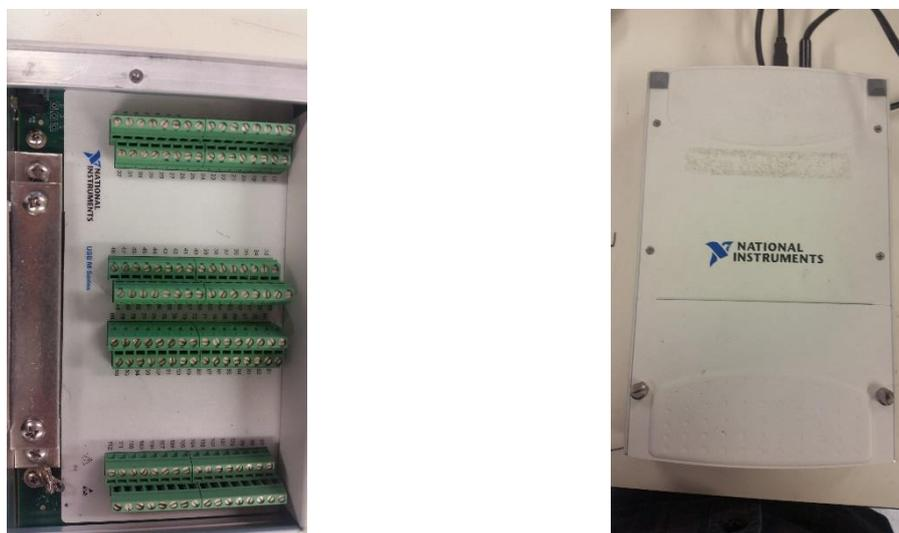
**Figure 4.71 NI 6225 USB DAQ system**
