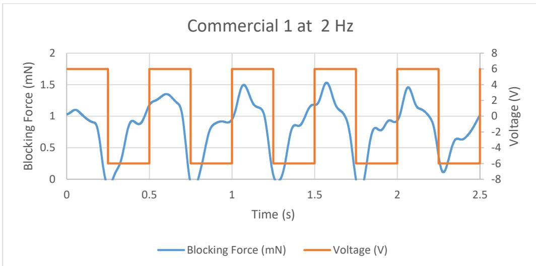
Figure 11.42 Blocking Force of Commercial 1 IPMC at 2 Hz
