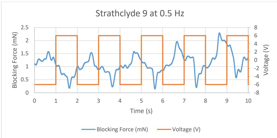
Figure 11.93 Blocking Force of Strathclyde 9 IPMC at 0.5 Hz
