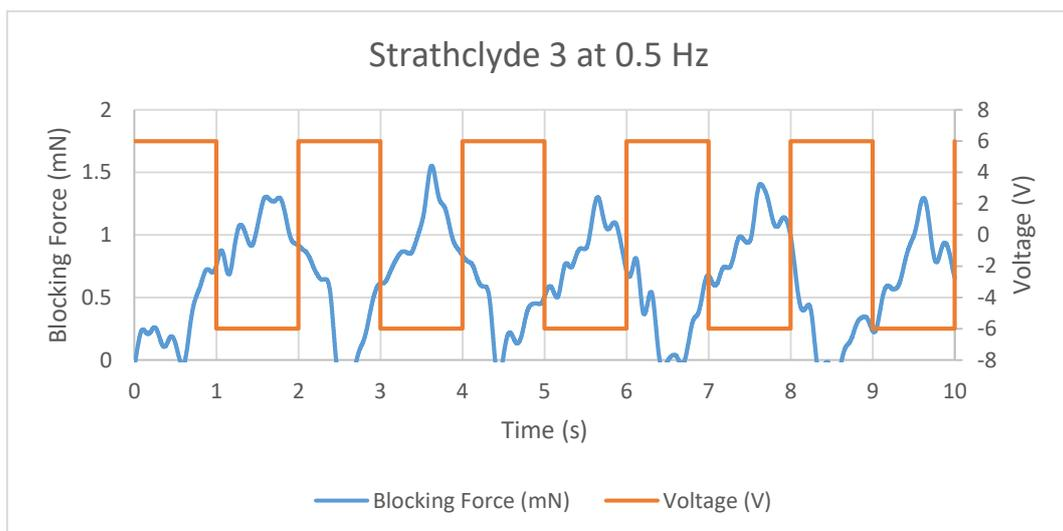
Figure 11.70 Blocking Force of Strathclyde 3 IPMC at 0.5 Hz
