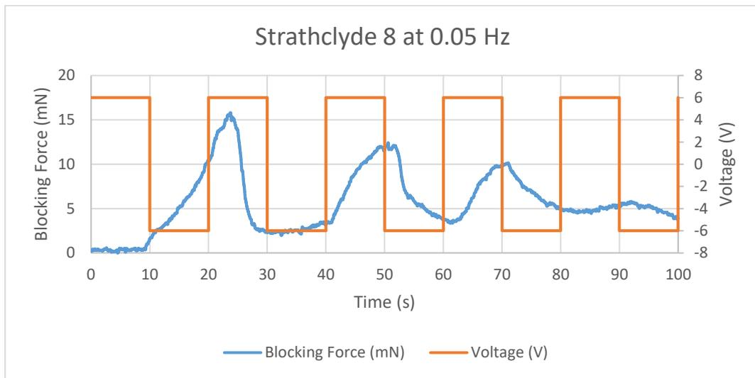
Figure 11.89 Blocking Force of Strathclyde 8 IPMC at 0.05 Hz
