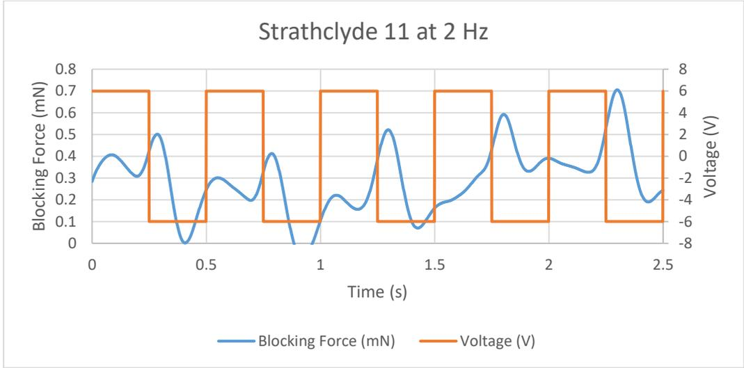
Figure 11.103 Blocking Force of Strathclyde 11 IPMC at 2 Hz
