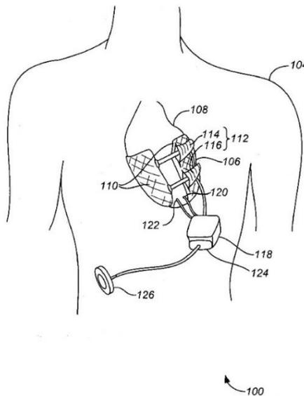
Figure 2.15 EAP Cardiac Apparatus (HEGDE, BUCH et al. 2004)
