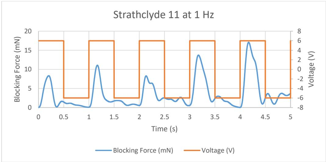
Figure 11.102 Blocking Force of Strathclyde 11 IPMC at 1 Hz
