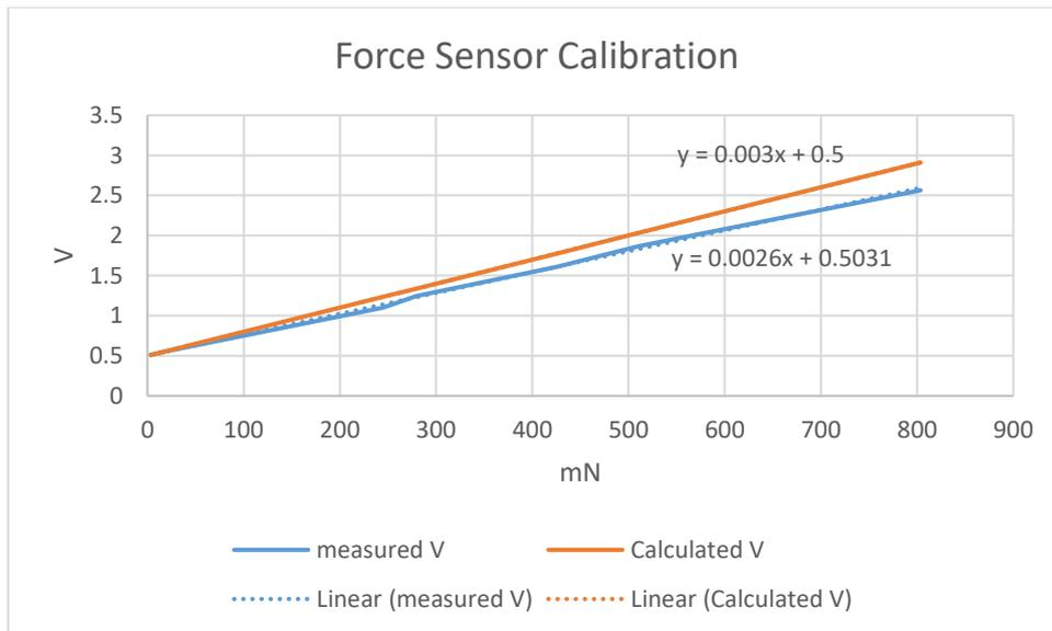
**Figure 4.70 Calibration graph of the force sensor**
