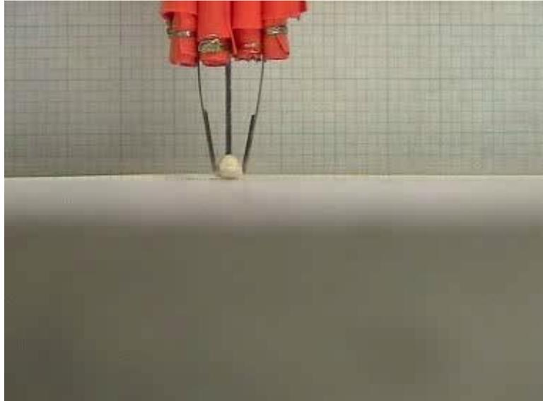
**Figure 2.7 Conducting Polymer Gripper (Alici and Huynh 2006)**
