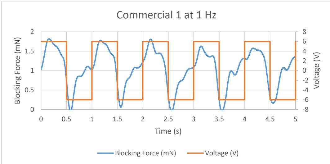
Figure 11.41 Blocking Force of Commercial 1 IPMC at 1 Hz
