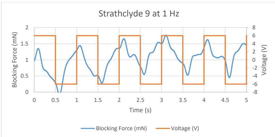
Figure 11.94 Blocking Force of Strathclyde 9 IPMC at 1 Hz
