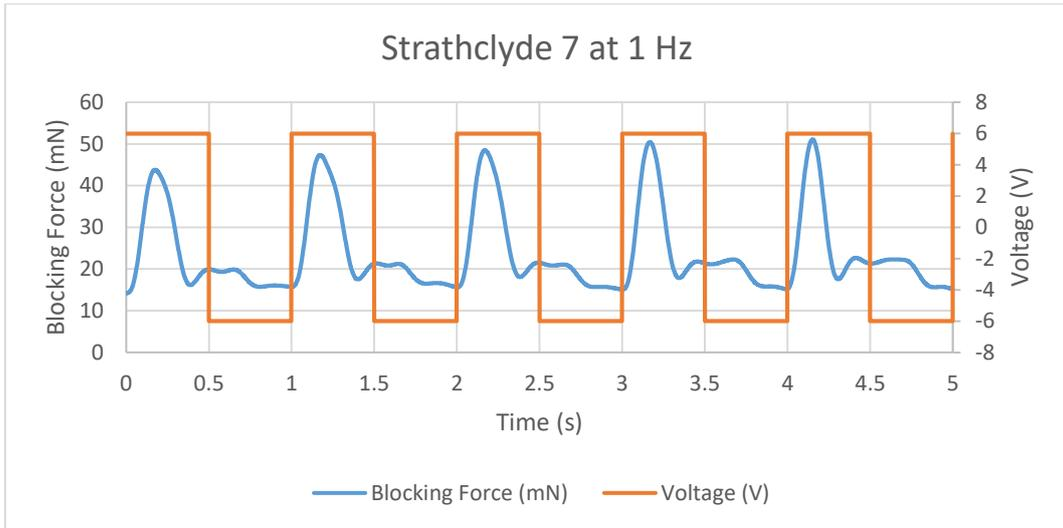
Figure 11.87 Blocking Force of Strathclyde 7 IPMC at 1 Hz
