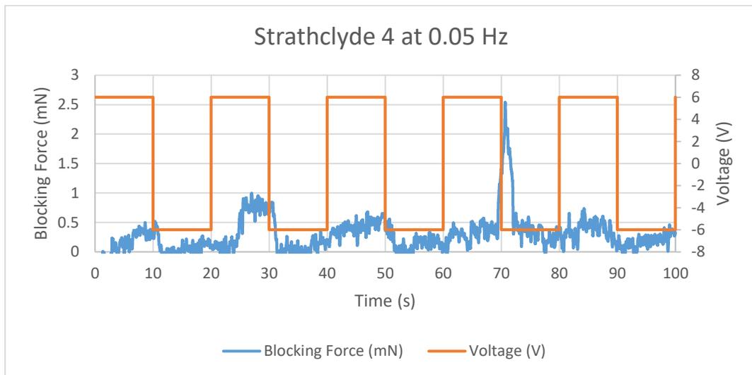
Figure 11.73 Blocking Force of Strathclyde 4 IPMC at 0.05 Hz
