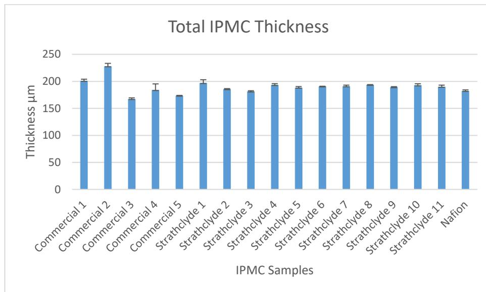
Figure 4.14 Total Thickness of the IPMC samples
