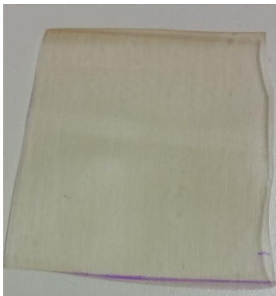
Figure 3.16 Nafion 117 after the surface preparation
