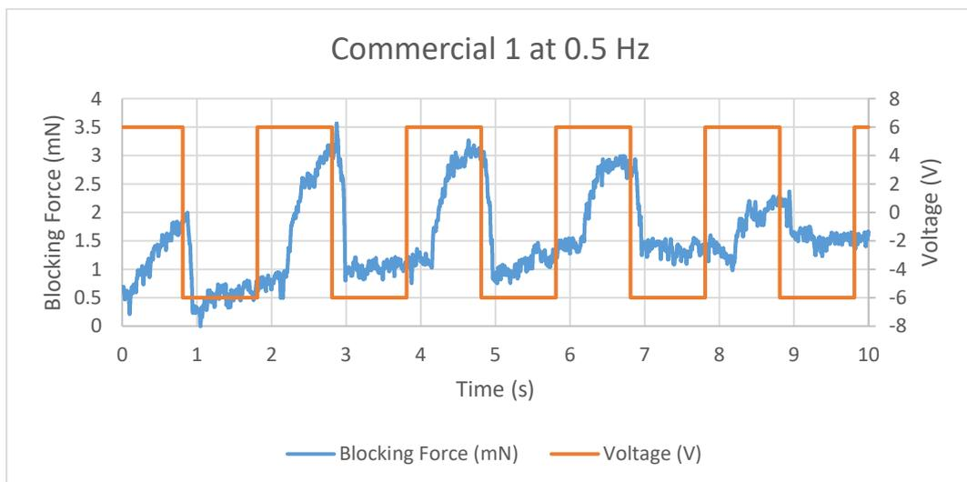
Figure 11.40 Blocking Force of Commercial 1 IPMC at 0.5 Hz
