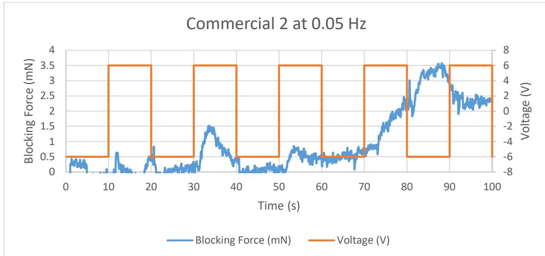
Figure 11.43 Blocking Force of Commercial 2 IPMC at 0.05 Hz
