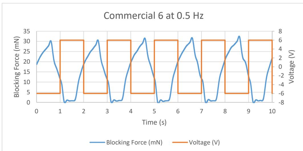
Figure 11.58 Blocking Force of Commercial 6 IPMC at 0.5 Hz
