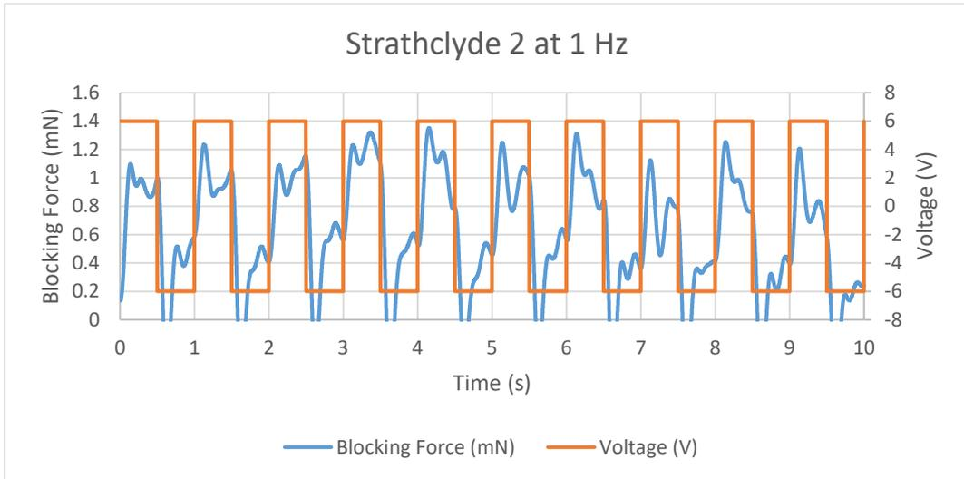
Figure 11.67 Blocking Force of Strathclyde 2 IPMC at 1 Hz
