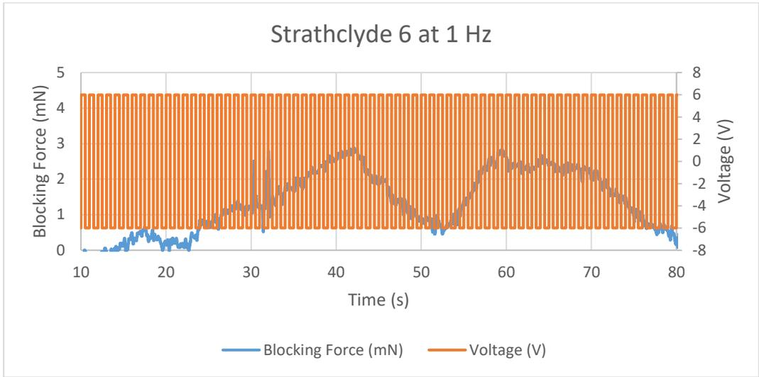
Figure 11.83 Blocking Force of Strathclyde 6 IPMC at 1 Hz
