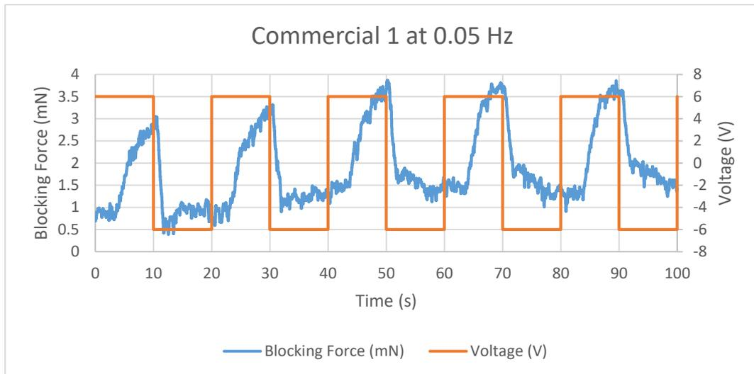
Figure 11.39 Blocking Force of Commercial 1 IPMC at 0.05 Hz
