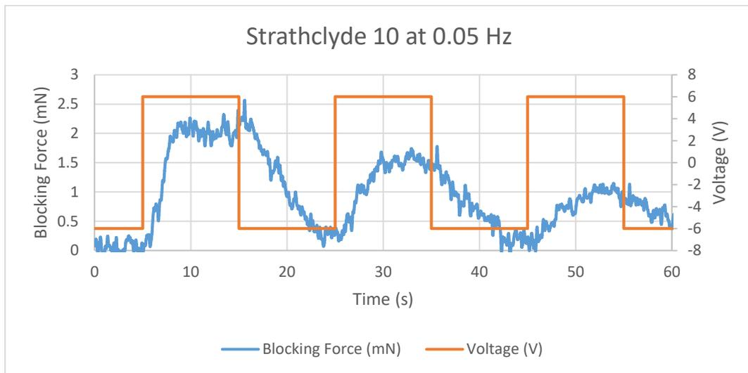
Figure 11.96 Blocking Force of Strathclyde 10 IPMC at 0.05 Hz
