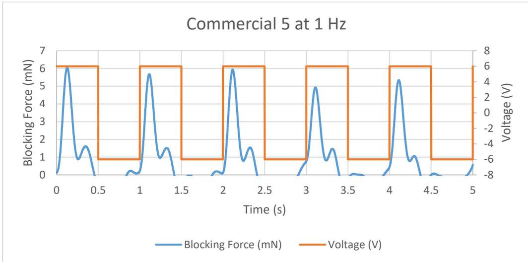
Figure 11.55 Blocking Force of Commercial 5 IPMC at 1 Hz
