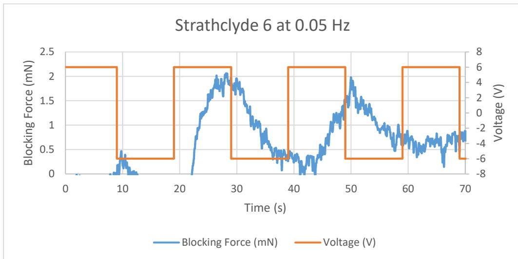
Figure 11.81 Blocking Force of Strathclyde 6 IPMC at 0.05 Hz
