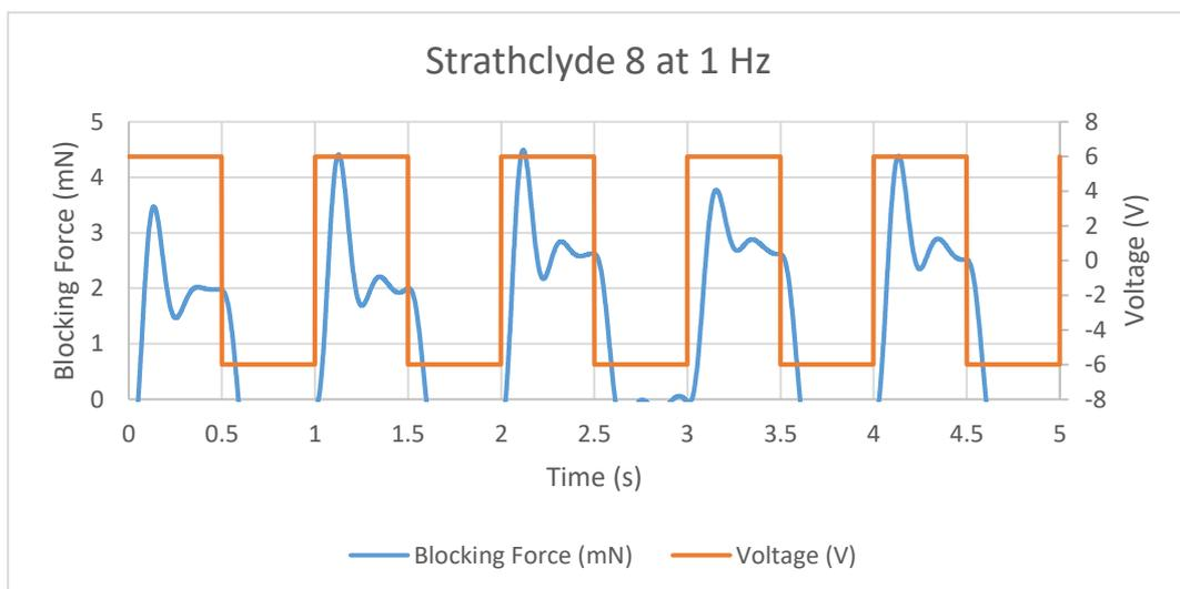
Figure 11.90 Blocking Force of Strathclyde 8 IPMC at 1 Hz
