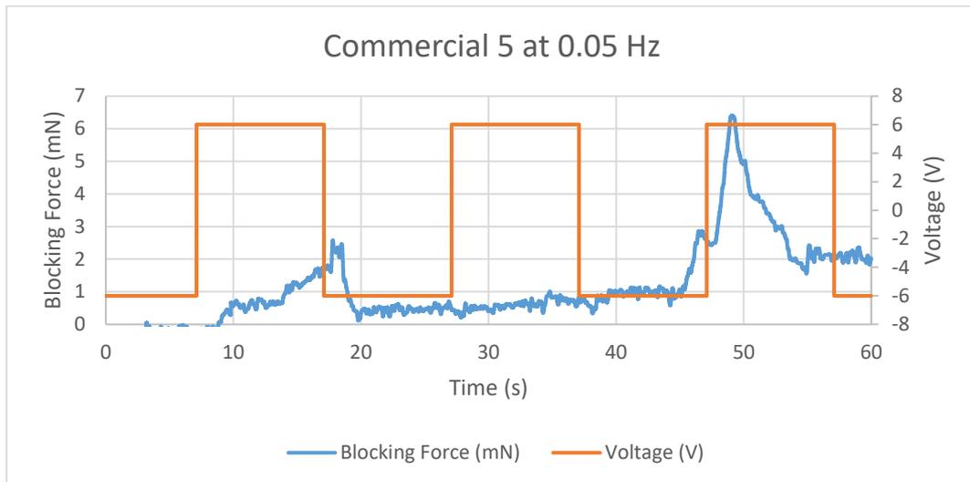
Figure 11.53 Blocking Force of Commercial 5 IPMC at 0.05 Hz
