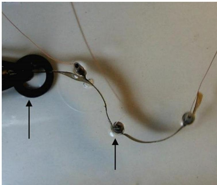
Figure 2.10 Artificial IPMC Cilium (Sareh, Rossiter et al. 2012)
