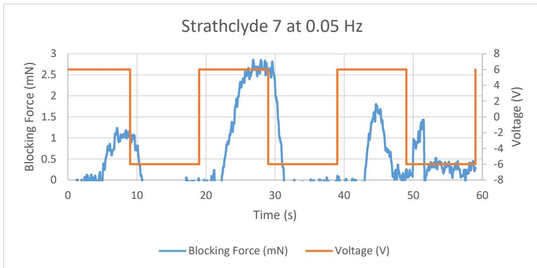
Figure 11.85 Blocking Force of Strathclyde 7 IPMC at 0.05 Hz
