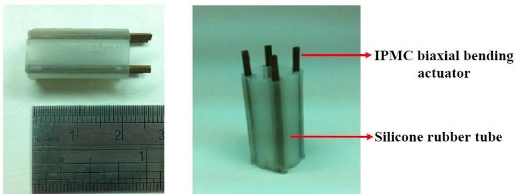
Figure 2.14 Fabricated IPMC-embedded tube showing four embedded IPMC biaxial bending actuators (Liu, Wang et al. 2014)
