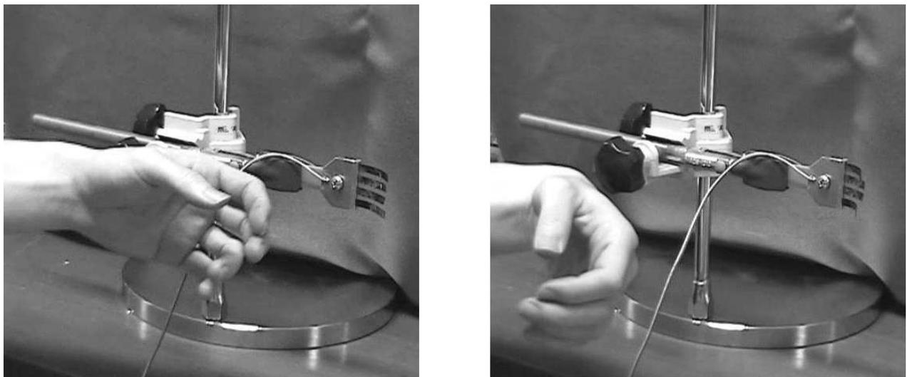
Figure 2.11 IPMC Hand Prosthesis (Lee, Jung et al. 2006)
