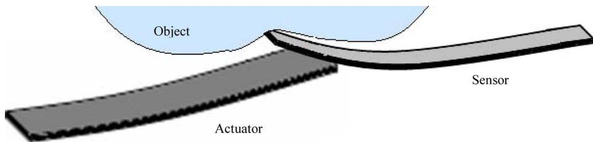
**Figure 2.12 IPMC Tactile Sensor (Bonomo, Brunetto et al. 2008)**
