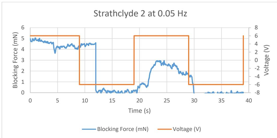
Figure 11.65 Blocking Force of Strathclyde 2 IPMC at 0.05 Hz
