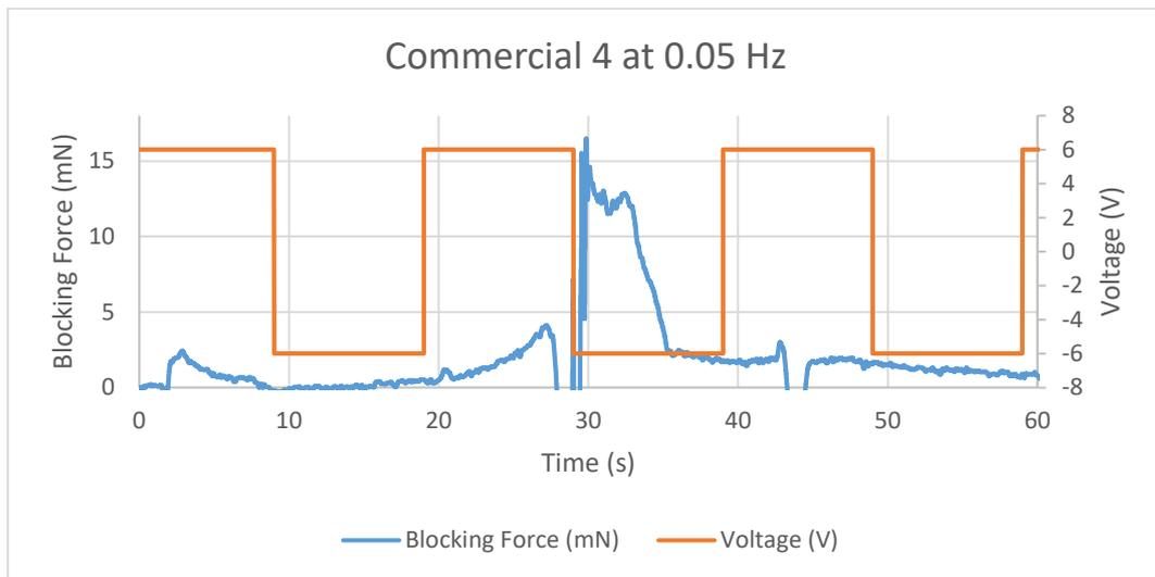
Figure 11.51 Blocking Force of Commercial 4 IPMC at 0.05 Hz
