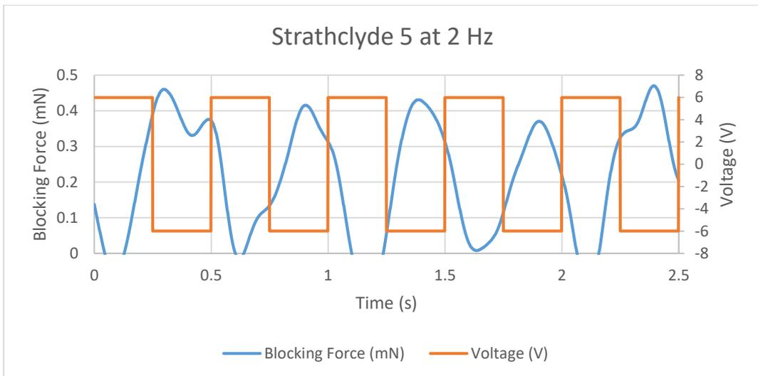
Figure 11.80 Blocking Force of Strathclyde 5 IPMC at 2 Hz
