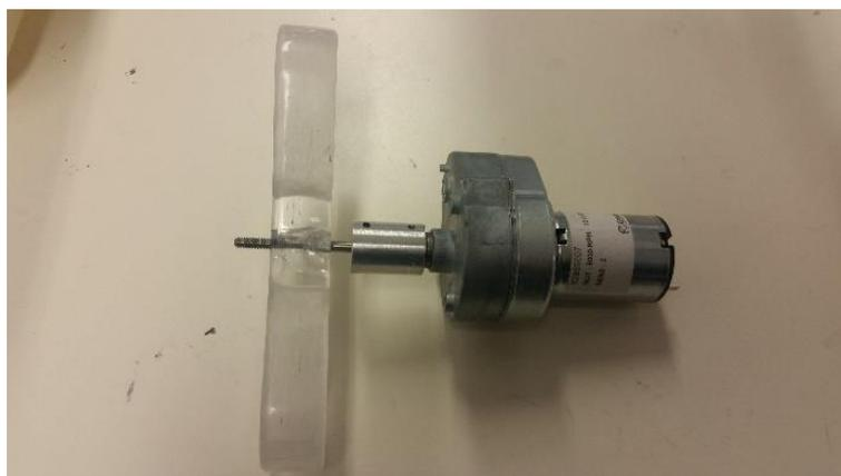
Figure 5.7 DC Motor with a polypropylene arm
