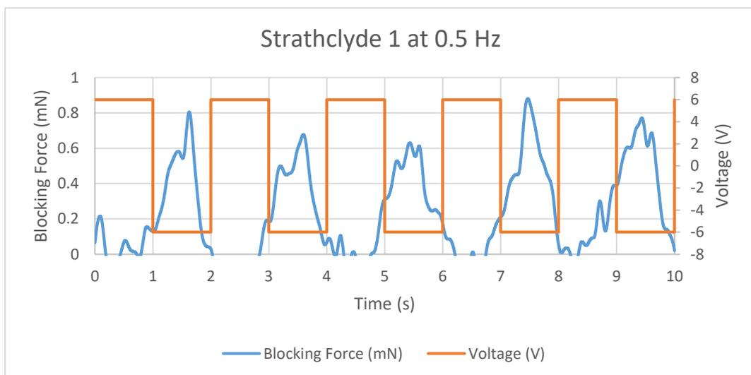
Figure 11.62 Blocking Force of Strathclyde 1 IPMC at 0.5 Hz
