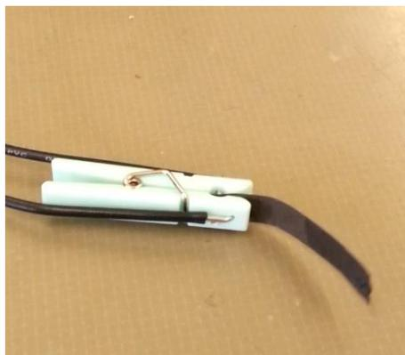
Figure 3.5 IPMC bending
