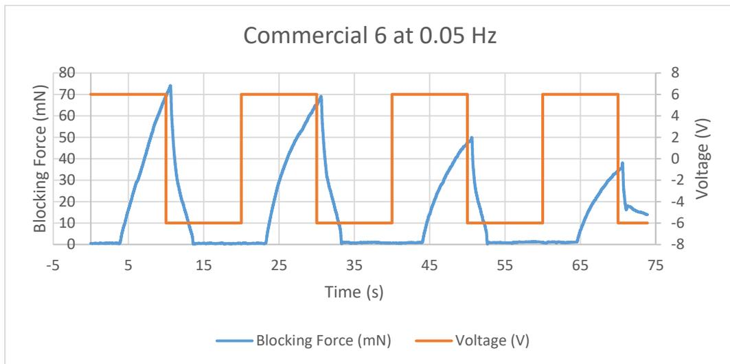
Figure 11.57 Blocking Force of Commercial 6 IPMC at 0.05 Hz
