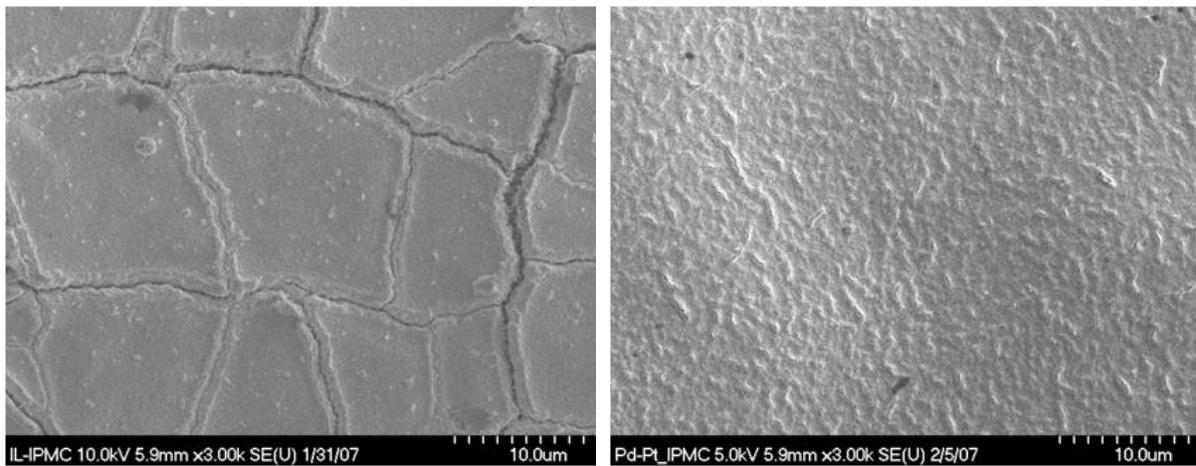
Figure 4.3 SEM images of IPMC without Pd on the left and with Pd on the right
