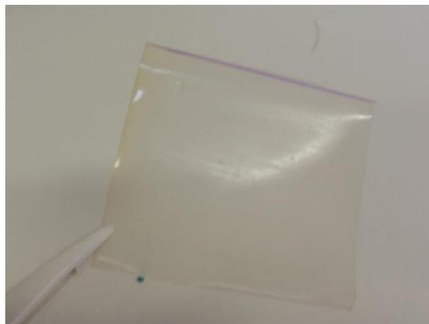
Figure 3.13 Nafion 117 membrane before surface treatment
