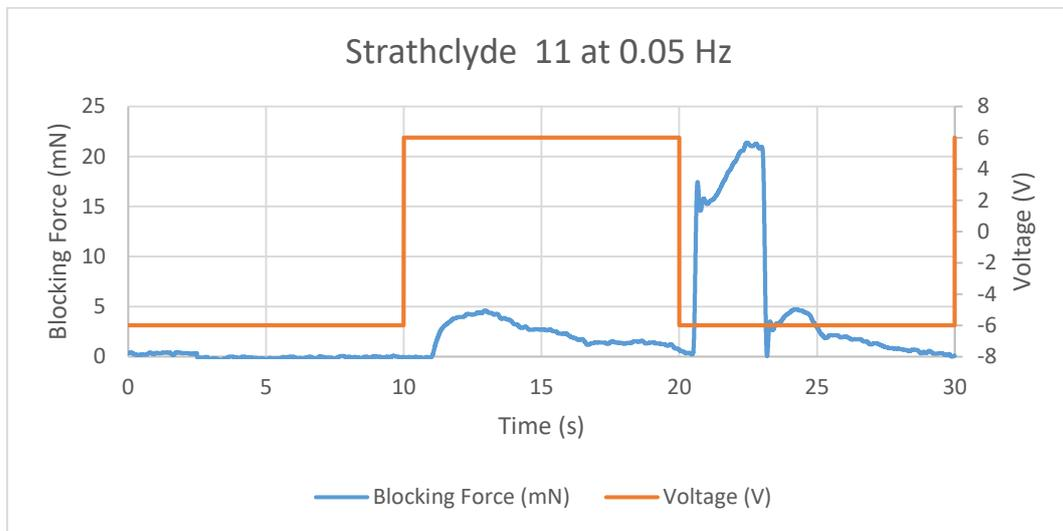
Figure 11.100 Blocking Force of Strathclyde 11 IPMC at 0.05 Hz
