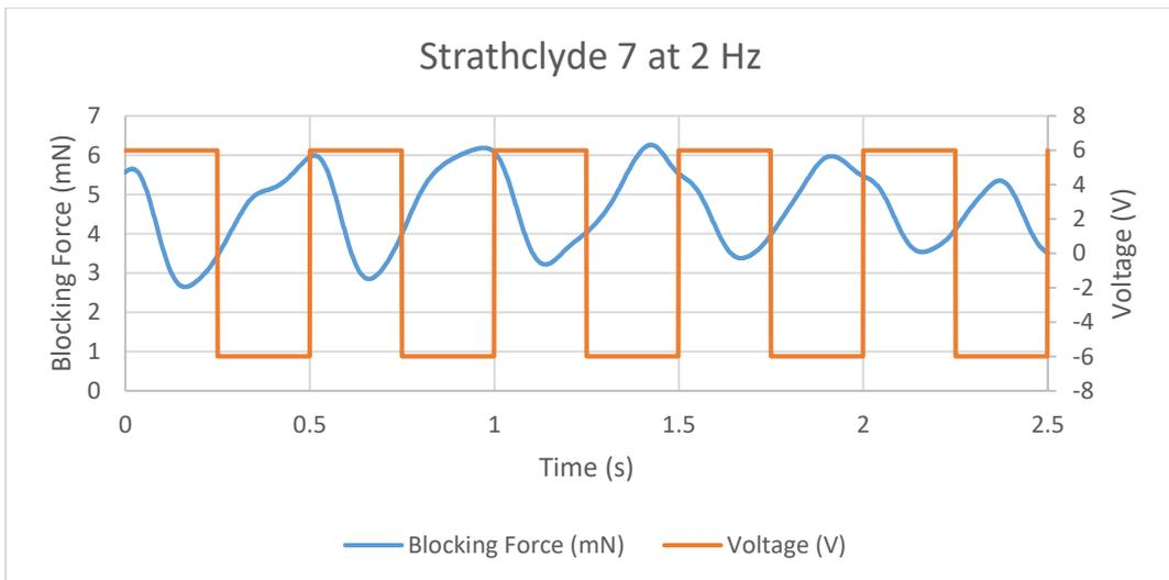
Figure 11.88 Blocking Force of Strathclyde 7 IPMC at 2 Hz
