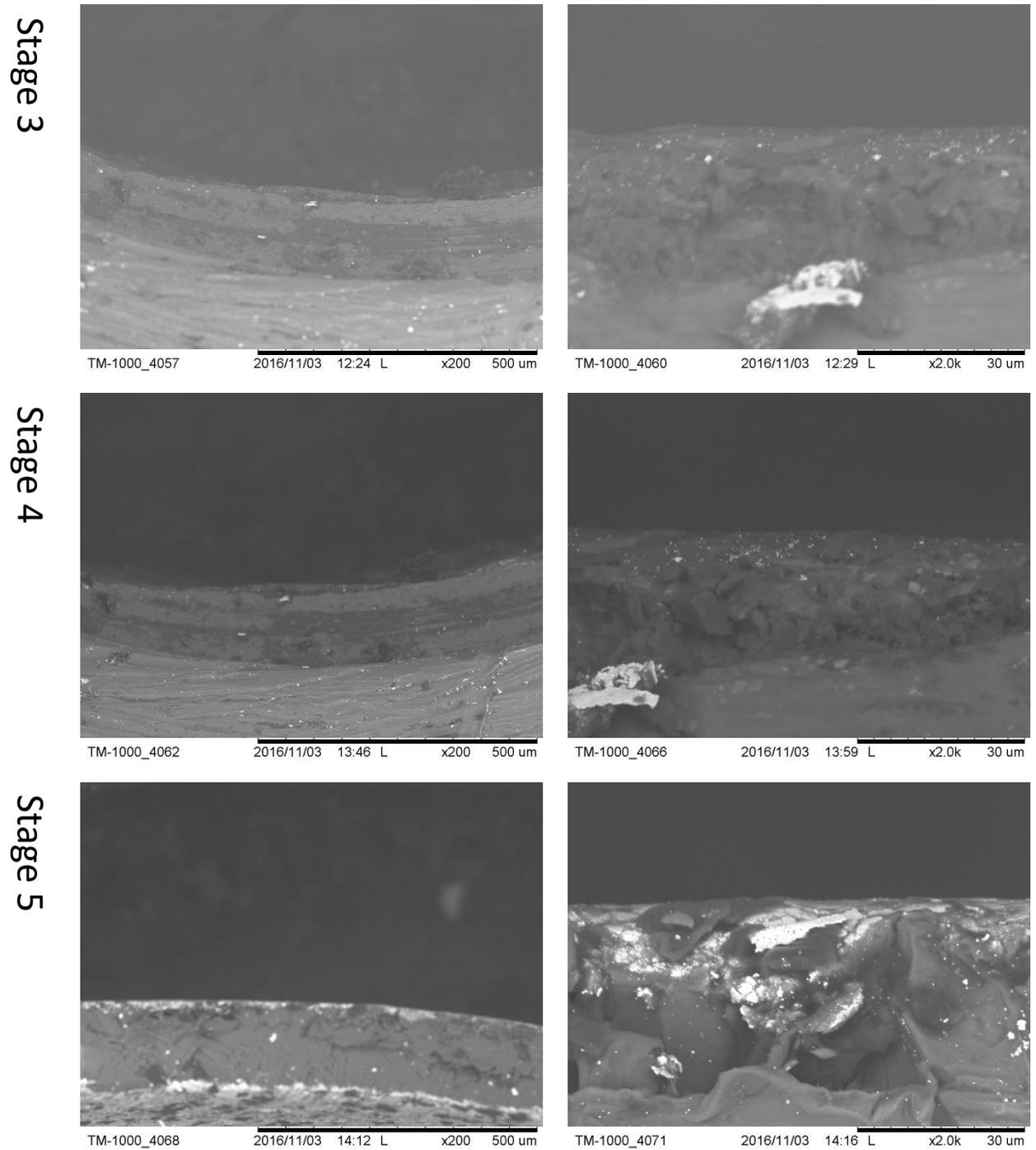
Figure 4.11 Cross Section images of Strathclyde 2 IPMC
