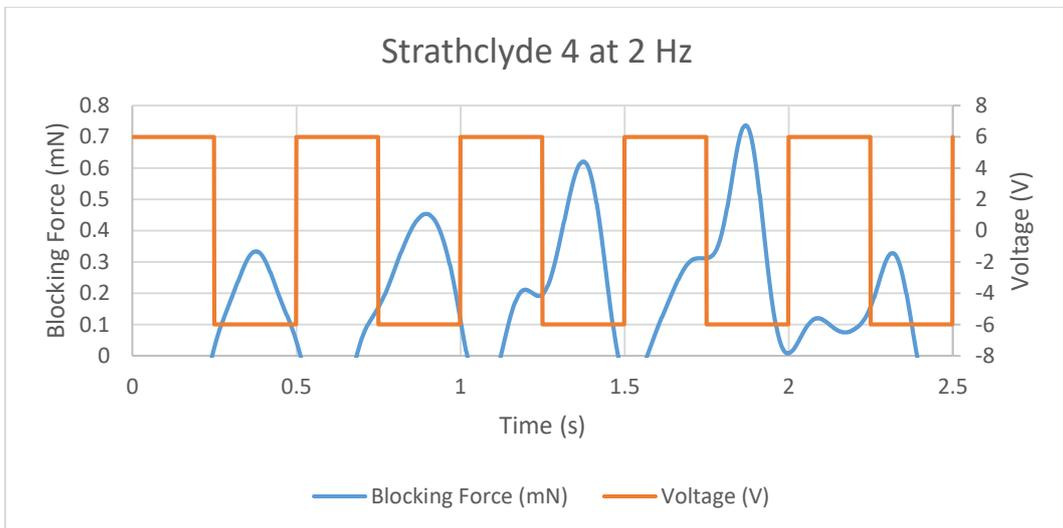
Figure 11.76 Blocking Force of Strathclyde 4 IPMC at 2 Hz
