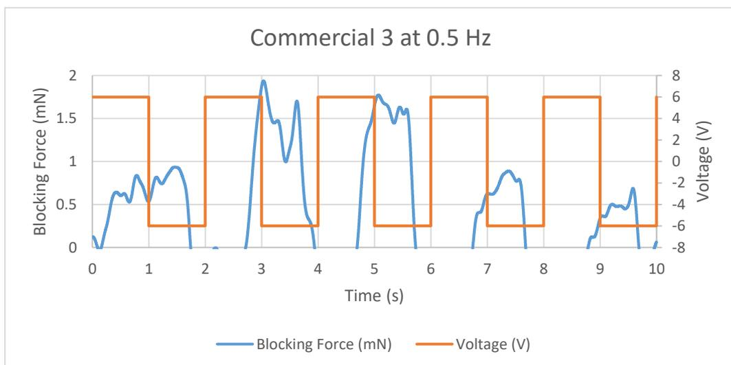
Figure 11.48 Blocking Force of Commercial 3 IPMC at 0.5 Hz
