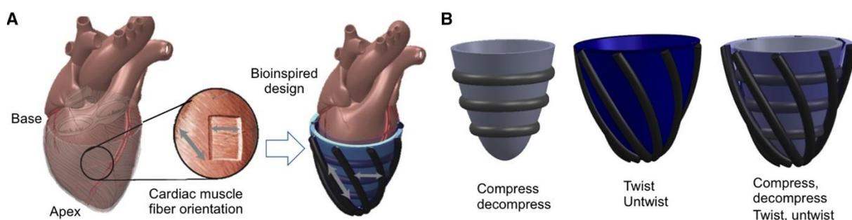
Figure 1.18 Soft Robotic Sleeve (Roche, Horvath et al. 2017)
