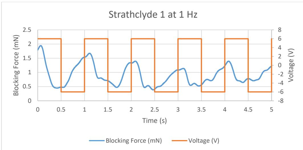
Figure 11.63 Blocking Force of Strathclyde 1 IPMC at 1 Hz
