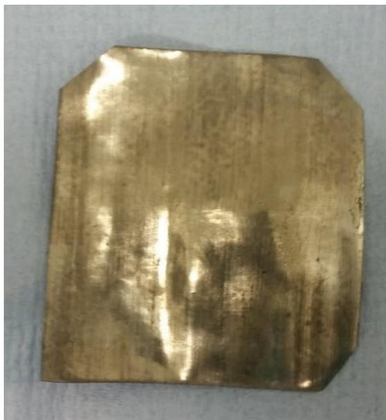
Figure 3.18 Nafion 117 after the Primary Plating stage
