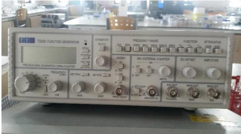
Figure 3.25 Second design function generator
