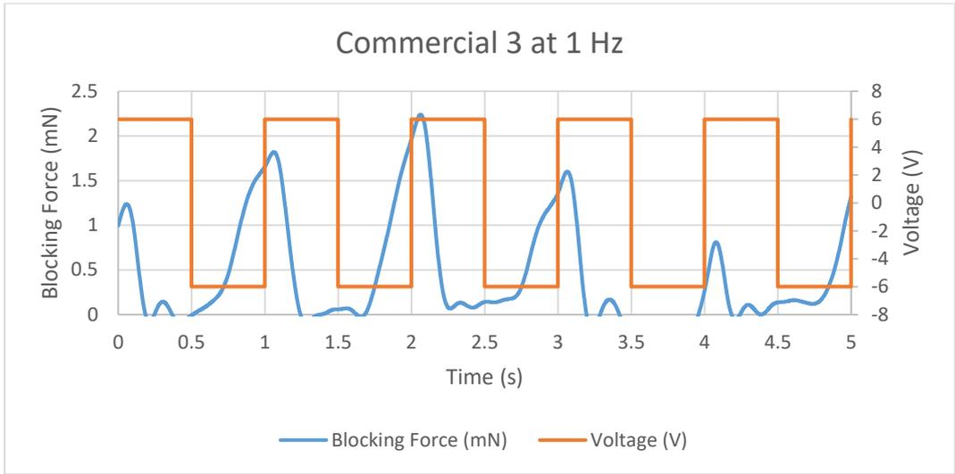
Figure 11.49 Blocking Force of Commercial 3 IPMC at 1 Hz
