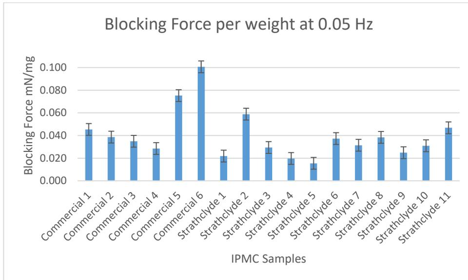
Figure 4.88 Maximum blocking force per weight at 0.05 Hz
