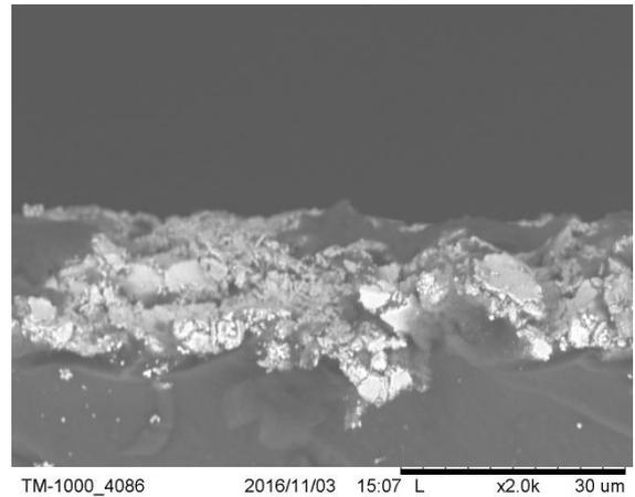
Figure 4.12 Cross Section images of Strathclyde 2 IPMC
