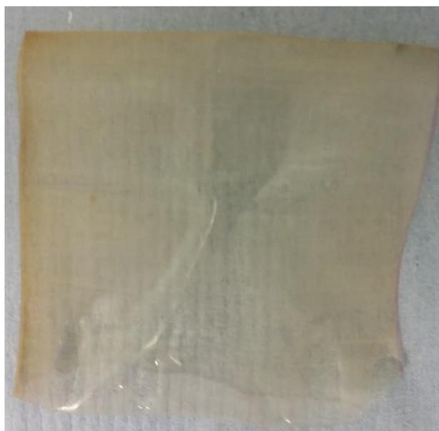
Figure 3.17 Nafion 117 membrane after the Ion-exchange stage.
