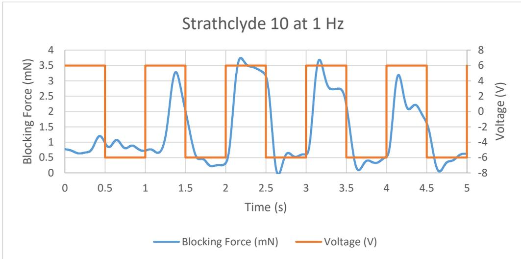
Figure 11.98 Blocking Force of Strathclyde 10 IPMC at 1 Hz
