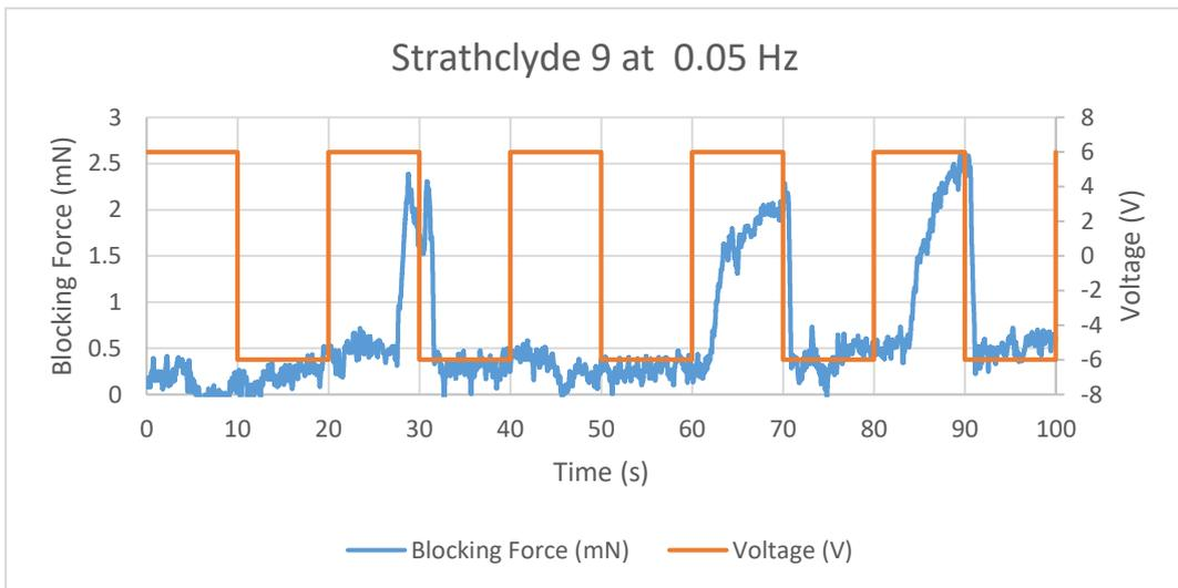
Figure 11.92 Blocking Force of Strathclyde 9 IPMC at 0.05 Hz
