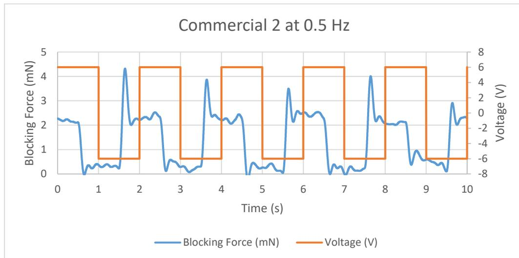
Figure 11.44 Blocking Force of Commercial 2 IPMC at 0.5 Hz
