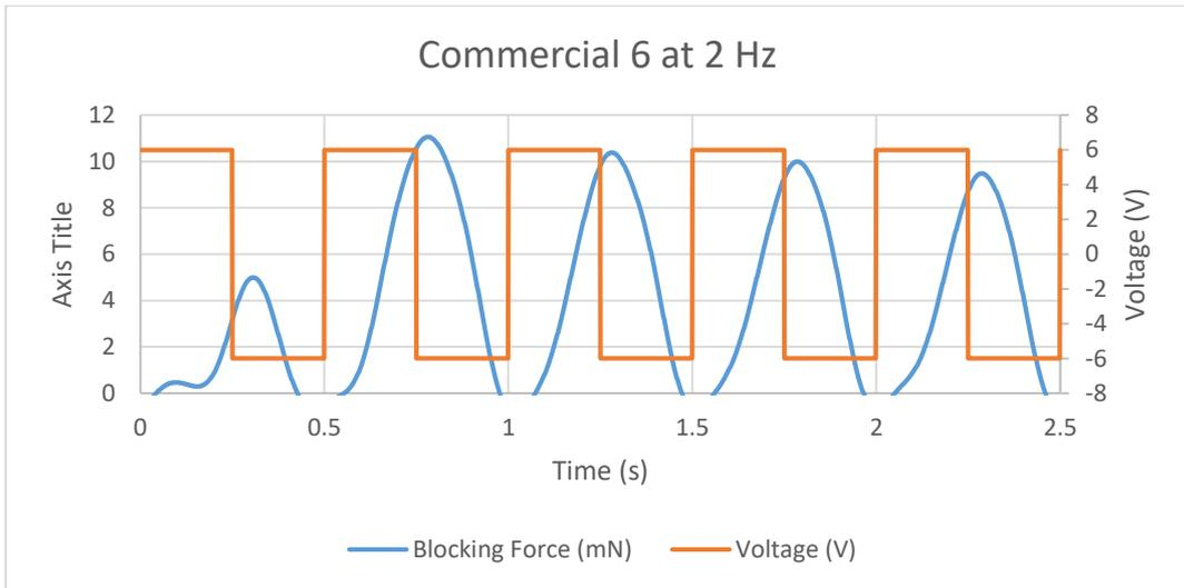
Figure 11.60 Blocking Force of Commercial 6 IPMC at 2 Hz
