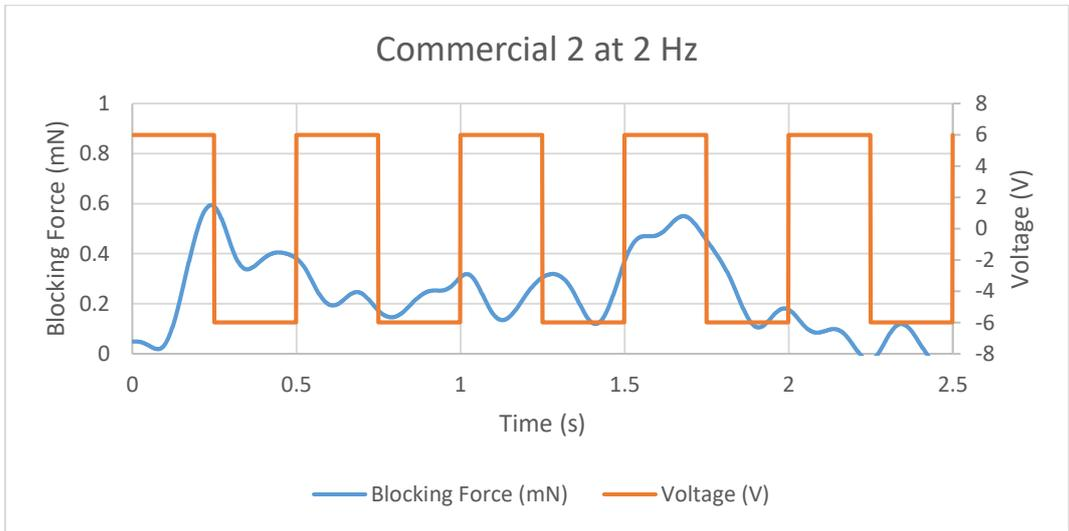
Figure 11.46 Blocking Force of Commercial 2 IPMC at 2 Hz
