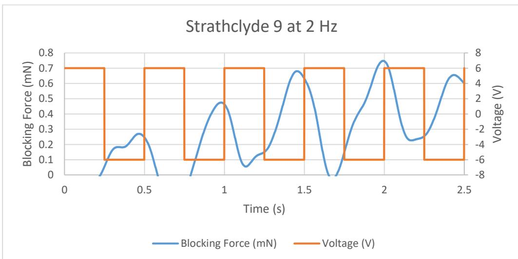
Figure 11.95 Blocking Force of Strathclyde 9 IPMC at 2 Hz
