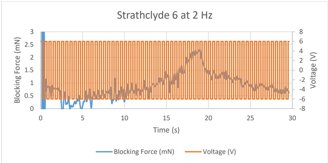
Figure 11.84 Blocking Force of Strathclyde 6 IPMC at 2 Hz
