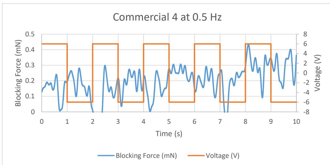
Figure 11.52 Blocking Force of Commercial 4 IPMC at 0.5 Hz
