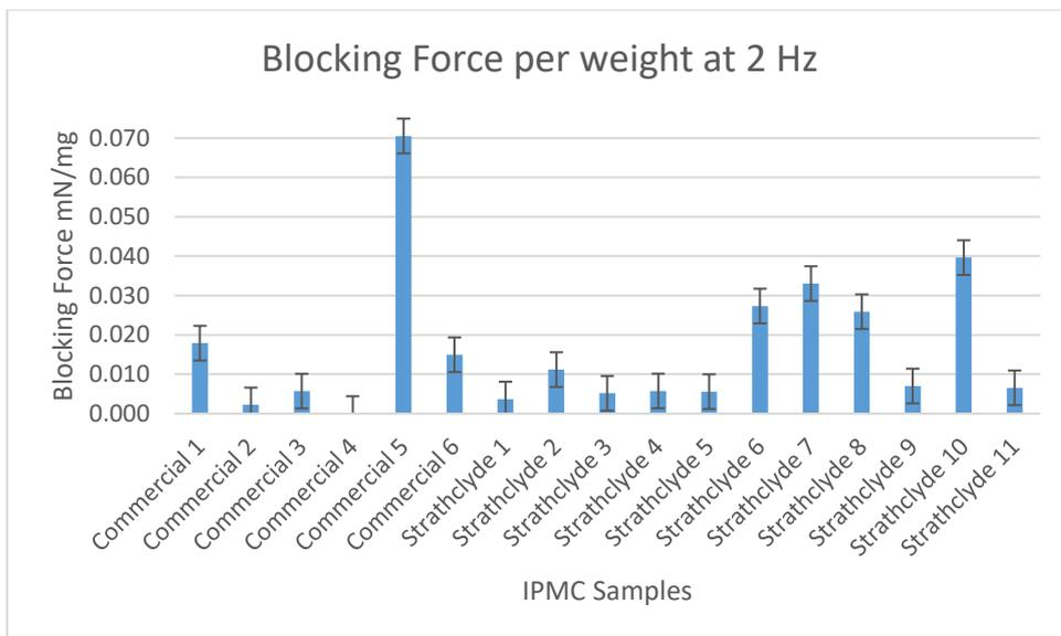
Figure 4.91 Maximum blocking force per weight at 2 Hz
