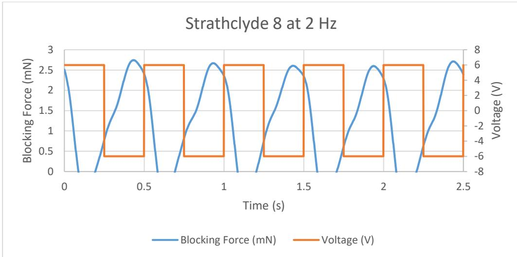
Figure 11.91 Blocking Force of Strathclyde 8 IPMC at 2 Hz
