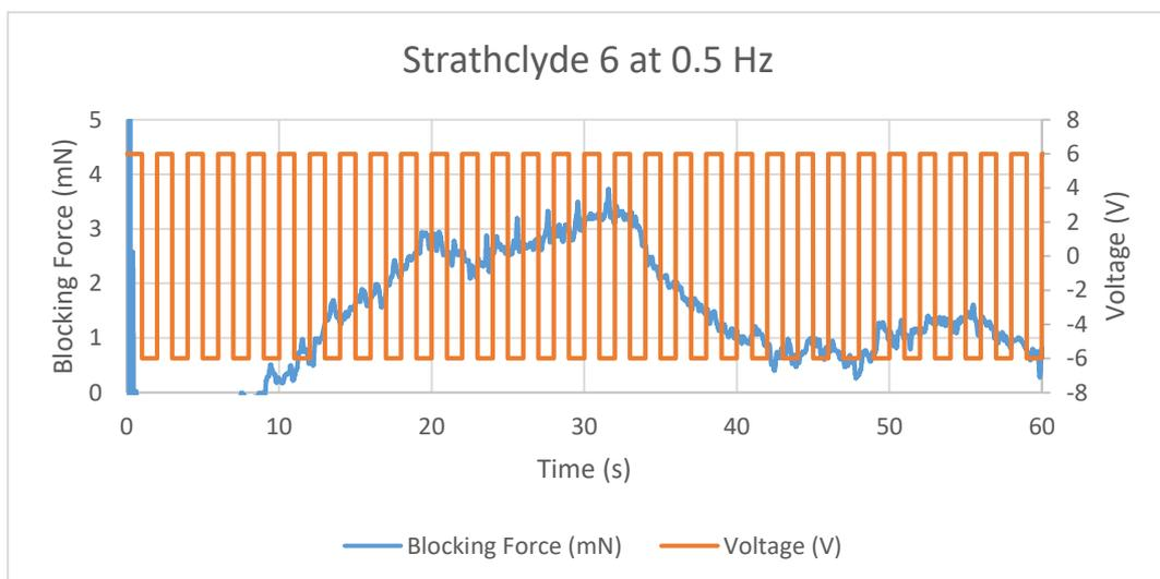
Figure 11.82 Blocking Force of Strathclyde 6 IPMC at 0.5 Hz
