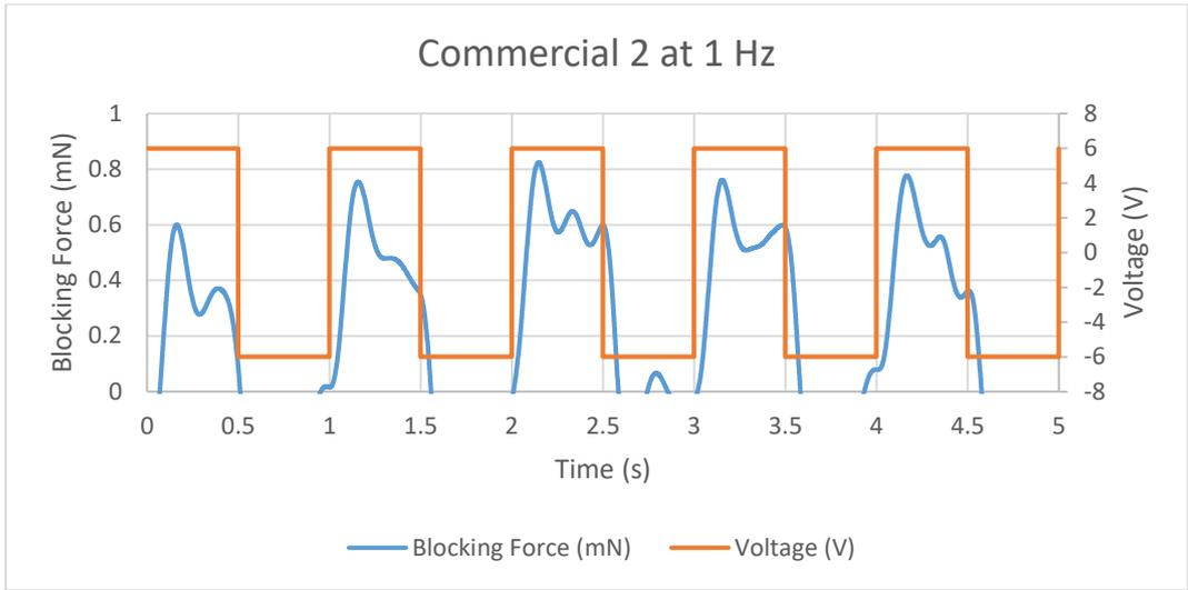
Figure 11.45 Blocking Force of Commercial 2 IPMC at 1 Hz
