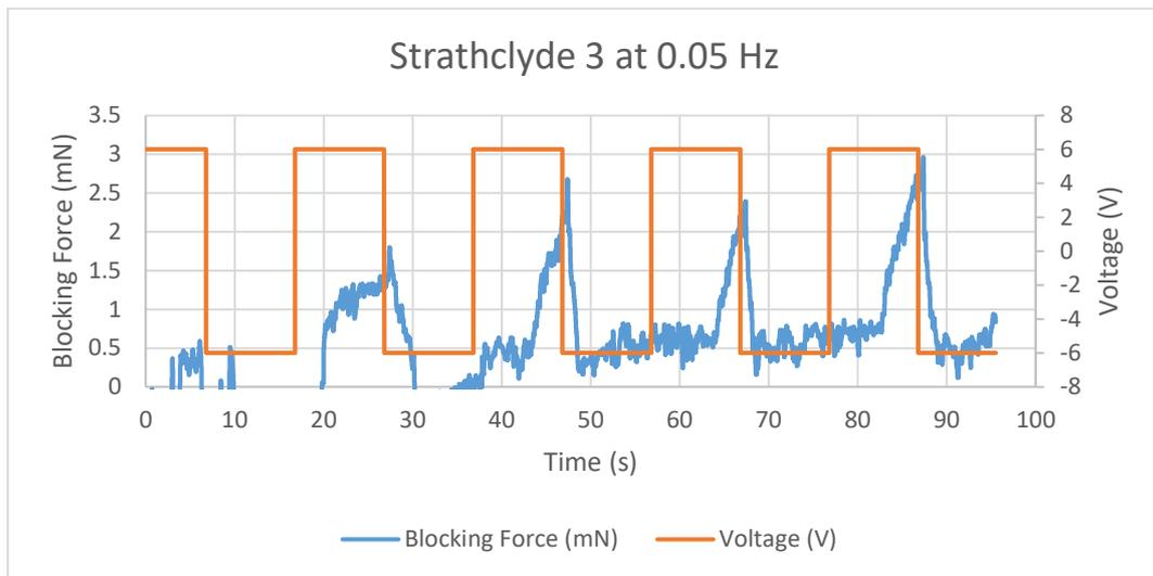
Figure 11.69 Blocking Force of Strathclyde 3 IPMC at 0.05 Hz
