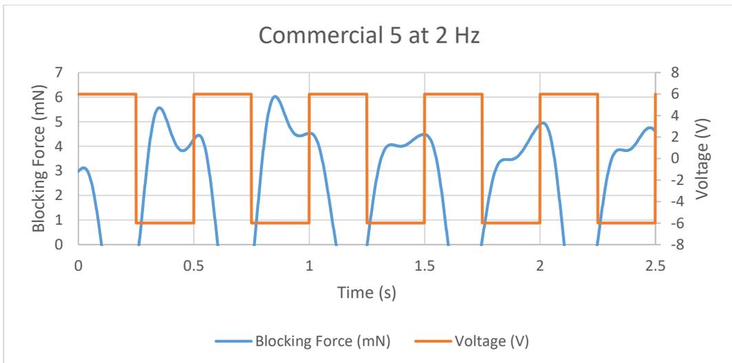
Figure 11.56 Blocking Force of Commercial 5 IPMC at 2 Hz
