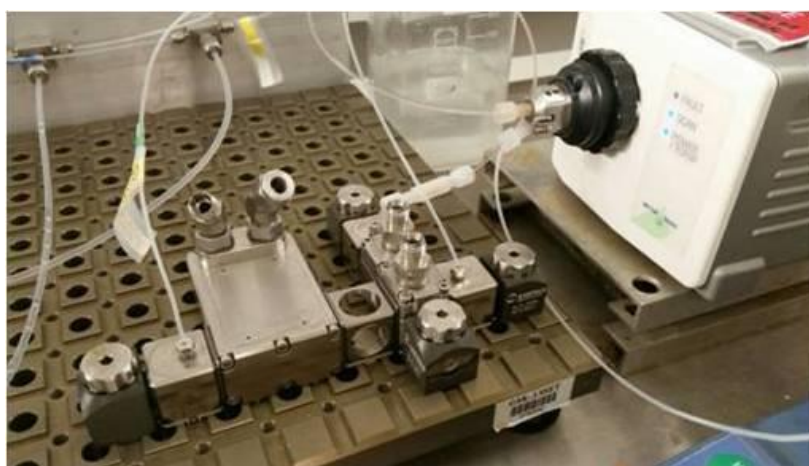
Figure 32 - Photograph of the flow React IR equipment set up.
