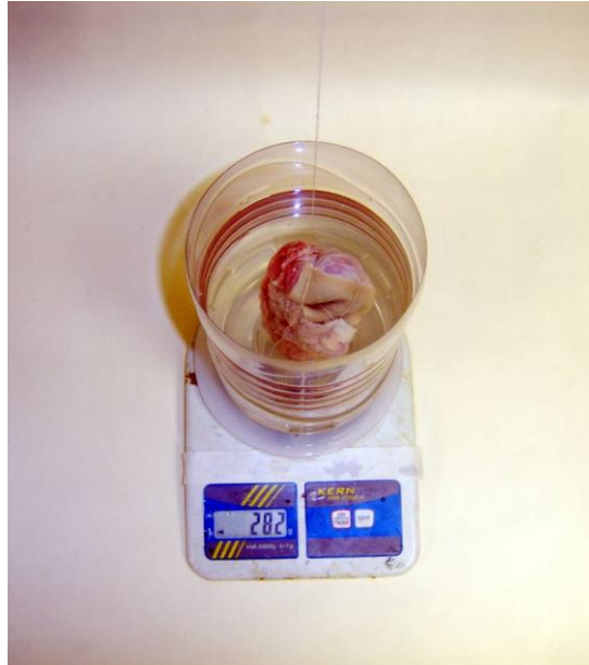
Figure 5-6: Volume measurement using water suspension method
