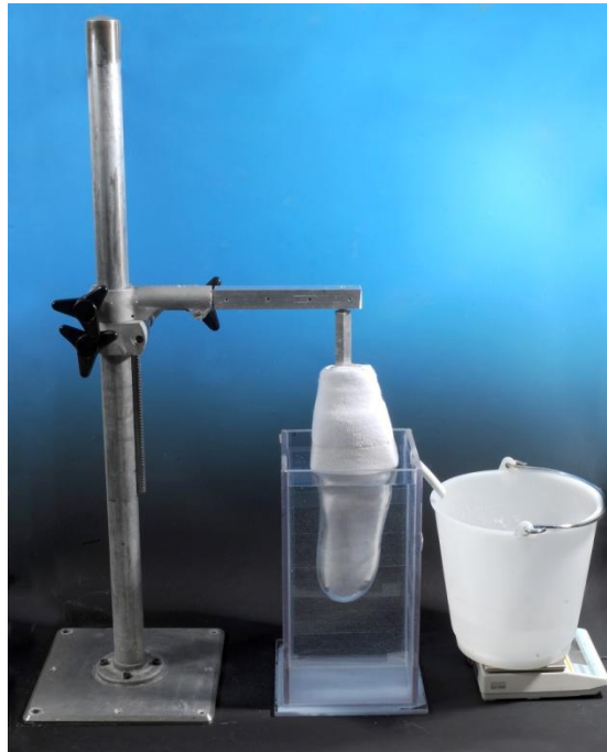
Figure 6-5: Water weighting of residual limb covered with one layer of towel sock
