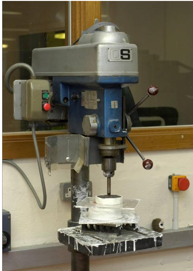
Figure 5-3: Wrapping POP using a drill
