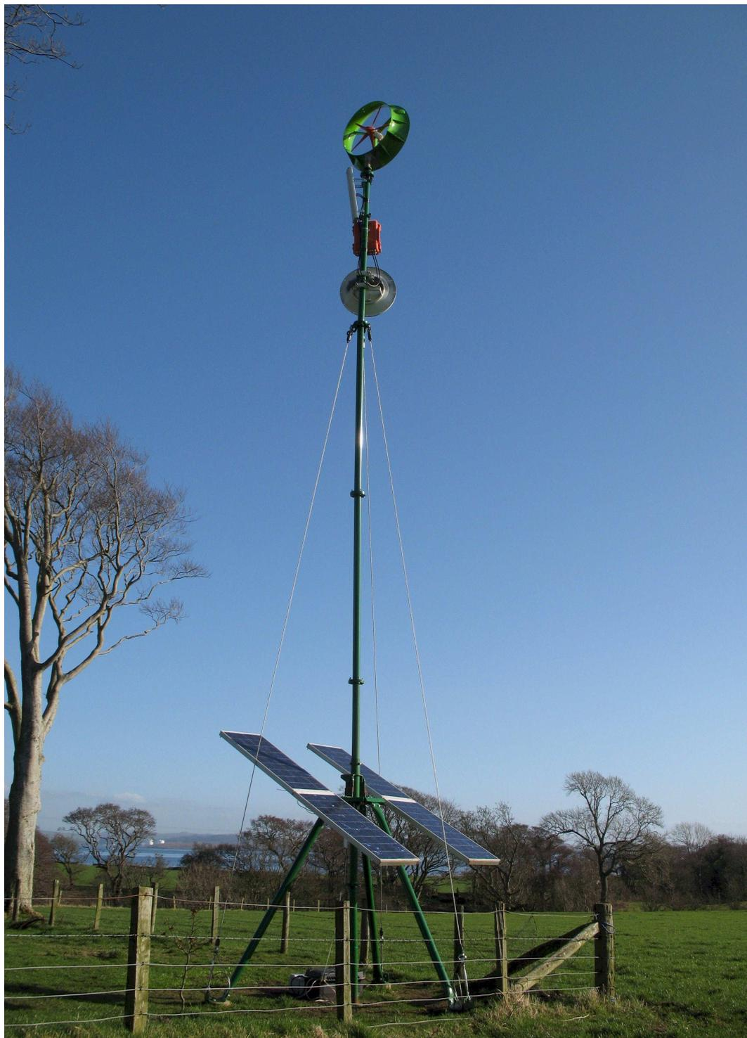
Figure 3.1: Prototype “WindFi” base station on the Isle of Bute, Scotland. The base of the unit includes photovoltaic modules and a battery bank (underground). The 10 m mast supports the wind turbine, antennas and radio equipment, housed in an orange weather-proof case just below the wind turbine.
