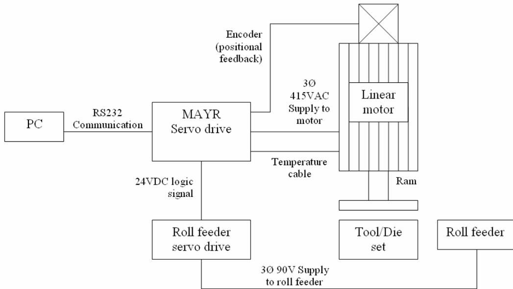
Fig. 5.1: The machine control architecture and the servo roll-feeder.
