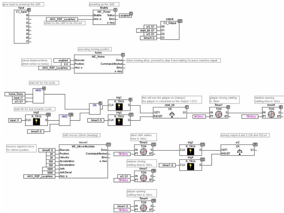
Fig. 8.10: CoDeSys GUI programming for the high-precision feeder.
