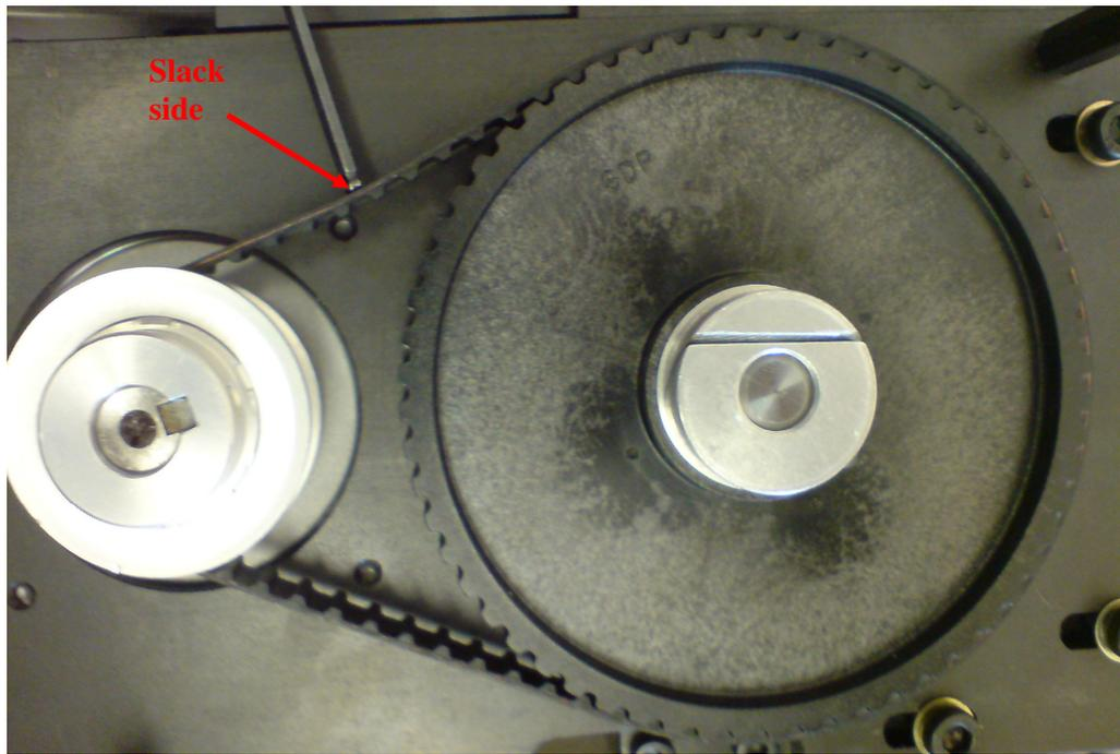
Fig. 5.23: The slack side of the belt and pulley mechanism, which also contributes to positional inaccuracies.
