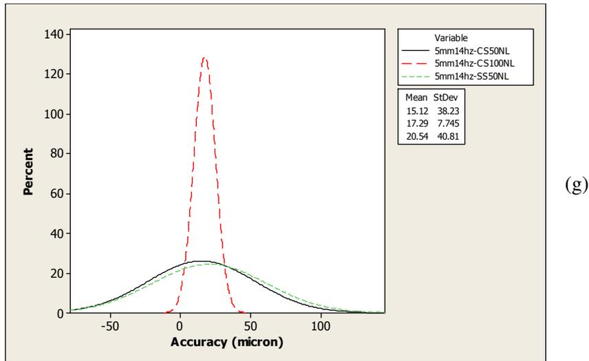
Fig. 5.16: Recorded positional accuracy for various materials in the non-lubrication case for all feed-frequencies and at 1mm feed distance: (a) to (g) represent feeding frequencies of 1-14Hz, respectively.
