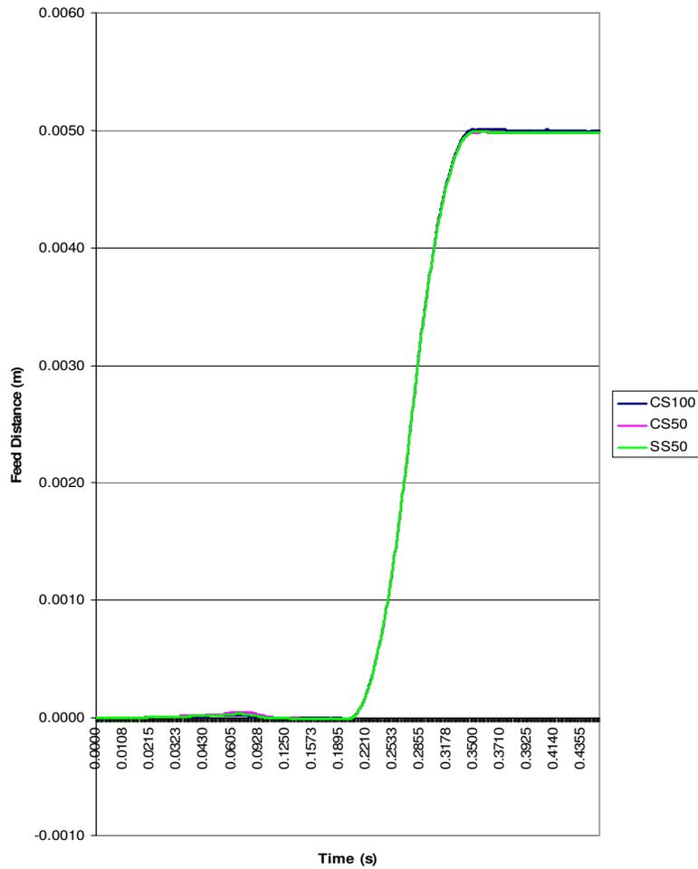
Fig. 4.13: Feeding characteristics for all strips for 5mm feed distance configured at 45-45 motion-profile with brake force at 2Hz feed frequency.
