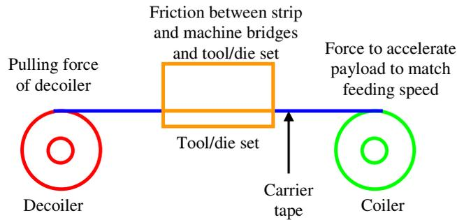
Fig. 10.6: Types of forces acting on the transportation system.
