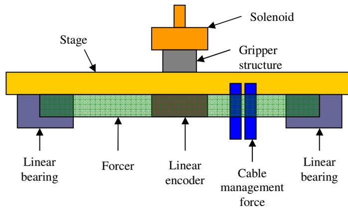
Fig. 9.1: Side-view anatomy of the developed feeder and payload estimation.
