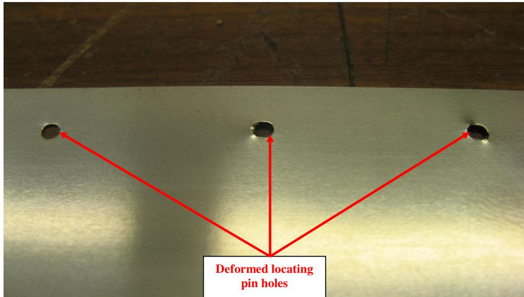
Fig. 5.17: Mis-location of feeding by using a micro-servo roll-feeder. It can be seen clearly that the pilot holes have suffered some deformation during positioned by locating pins.
