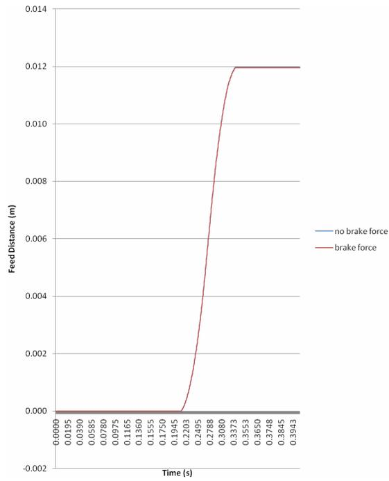
Fig. 10.15: Feed characteristic for 2Hz feed-frequency and 45-45 motion profile.
