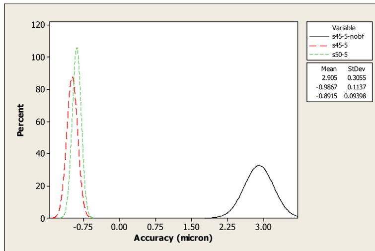
Fig. 7.27: Settled positional accuracy pattern for different motion profile curve and effect of brake force for SS50 strip at 5mm feed distance and 2Hz feed frequency.
