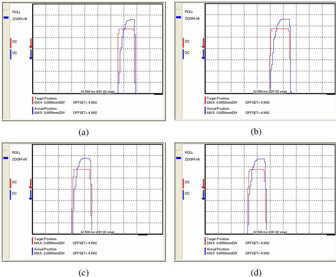
Fig. 9.6: The response of the feeder to various motion-profile time-frames: (a) 15-15%; (b) 30-30%; (c) 45-45; and (d) 50-50%.
