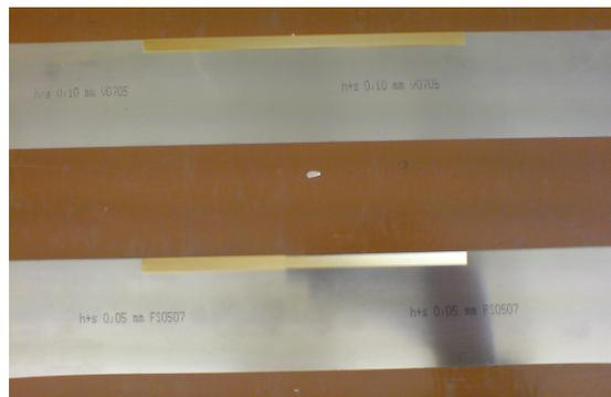
Fig. 5.6: The linear-tape-scale fixed onto the strips.
