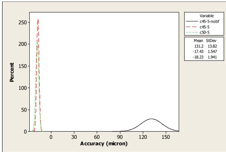
Fig. 4.25: Settled-positional accuracy-pattern for different motion-profile curves and the effect of brake force for CS50 strip at 5mm feed distance and 2Hz feed frequency.
