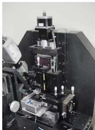
Fig. 2.7: Developed micro-punching press machine [Byung et al., 2005].
