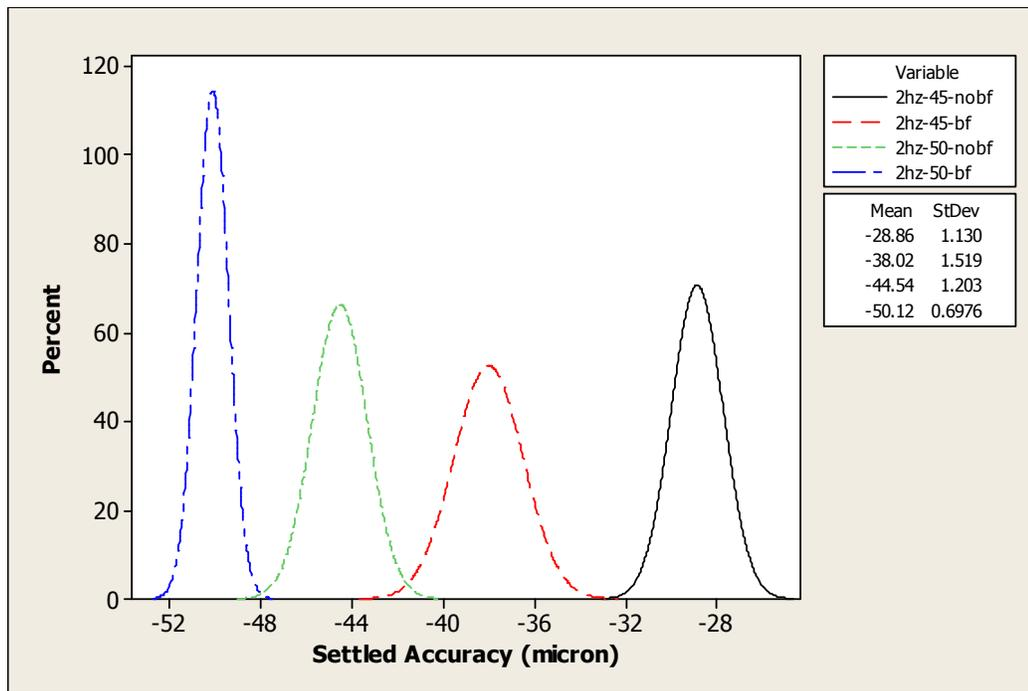
Fig. 10.18: The effect of brake-force for both motion-profiles at 2Hz feed-frequency.
