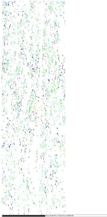
Fig. 3.21: EBSD mapping image of indexed  $<1\mu\text{m}$  grain size.
