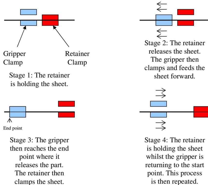
Fig. 2.13: Working principle of gripper feeder.
