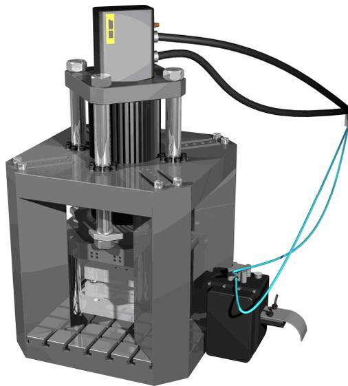
Fig. 6.1: 3D model of the micro-sheet-forming machine.
