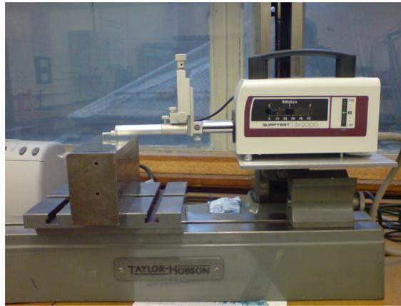
Fig. 3.1: Mitutoyo Surftest SV2000 equipment used to measure surface roughness.
