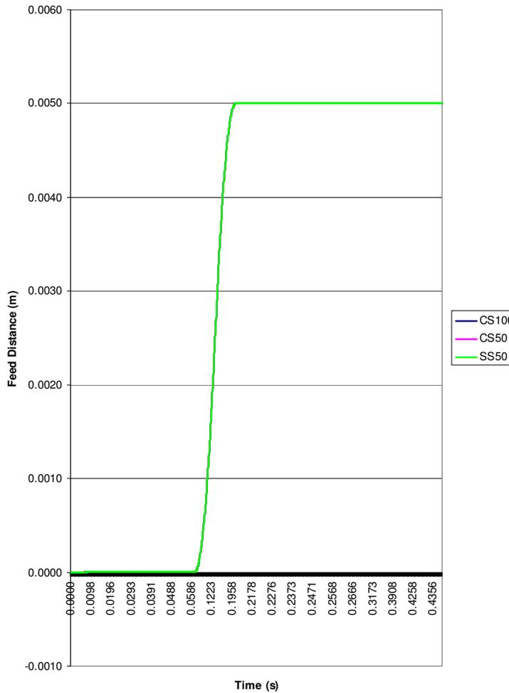
Fig. 7.7: Feeding characteristic for all strips for 5mm feed distance, 2Hz frequency configured at 45-45 motion profile without brake force.
