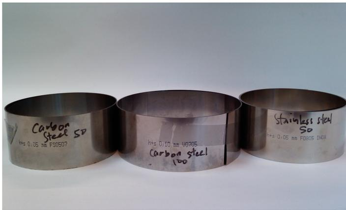
Fig. 3.3: Carbon- and stainless-steel strips used in the research.
