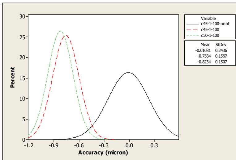
Fig. 7.19: Settled positional accuracy pattern for different motion profile curve and effect of brake force for CS100 strip at 1mm feed distance and 2Hz feed frequency.
