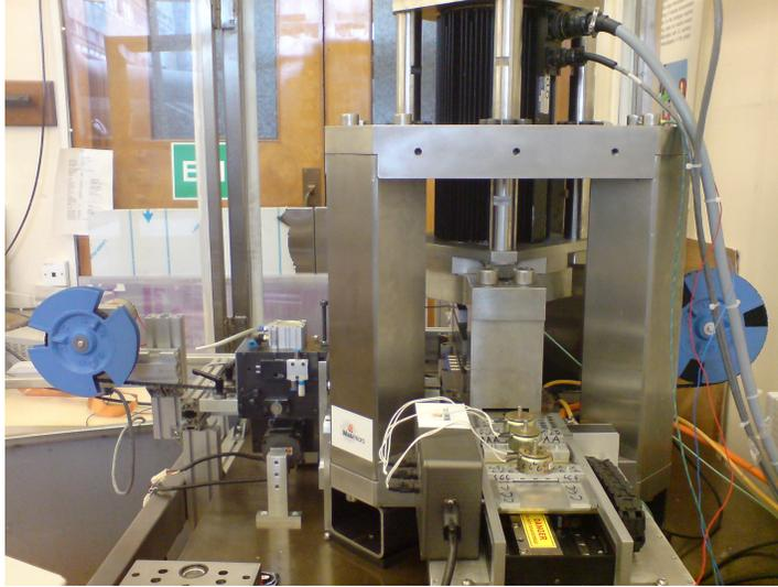
Fig. 10.5: Part-transport system developed for the handling of finished micro-parts.
