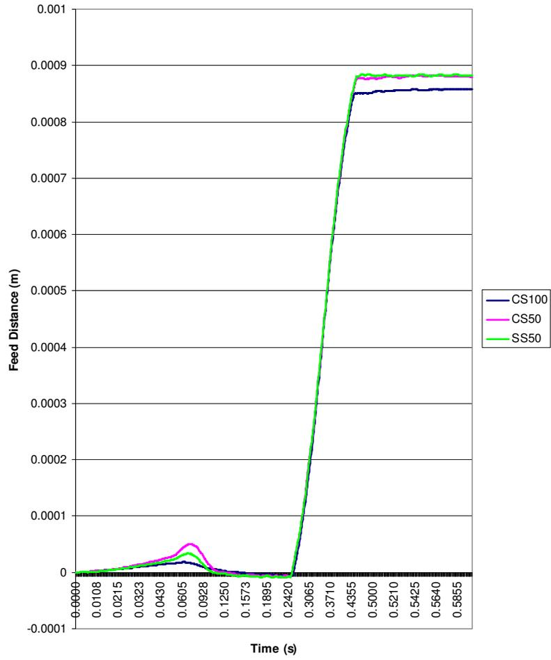
Fig. 4.6: Feeding characteristics for all strips for 1mm feed distance configured at 45-45 motion-profile with brake force at 1Hz feed frequency.
