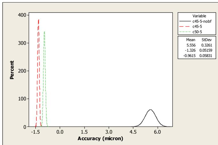
Fig. 7.23: Settled positional accuracy pattern for different motion profile curve and effect of brake force for CS50 strip at 5mm feed distance and 2Hz feed frequency.
