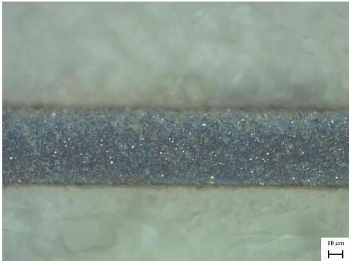
Fig. 3.15: CS50 at 500x magnifications, showing iron carbide/cementite (white colour).
