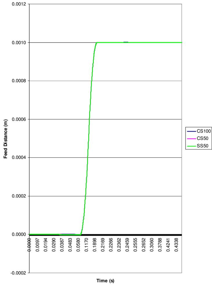
Fig. 7.13: Feeding characteristic for all strips for 1mm feed distance, 2Hz frequency configured at 50-50 motion profile with brake force.
