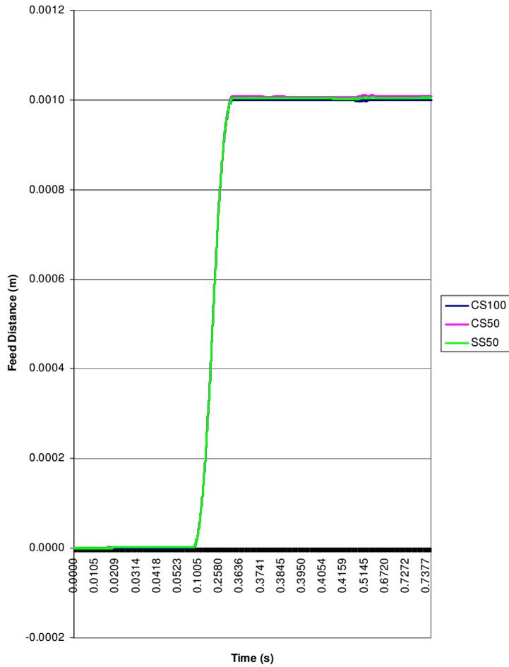
Fig. 7.4: Feeding characteristic for all strips for 1mm feed distance, 1Hz frequency configured at 45-45 motion profile without brake force.
