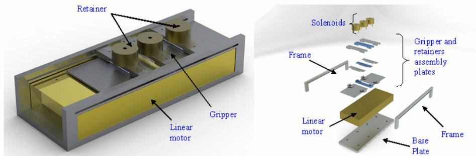
Fig. 8.1: Conceptual design of the high-precision micro-forming feeder.
