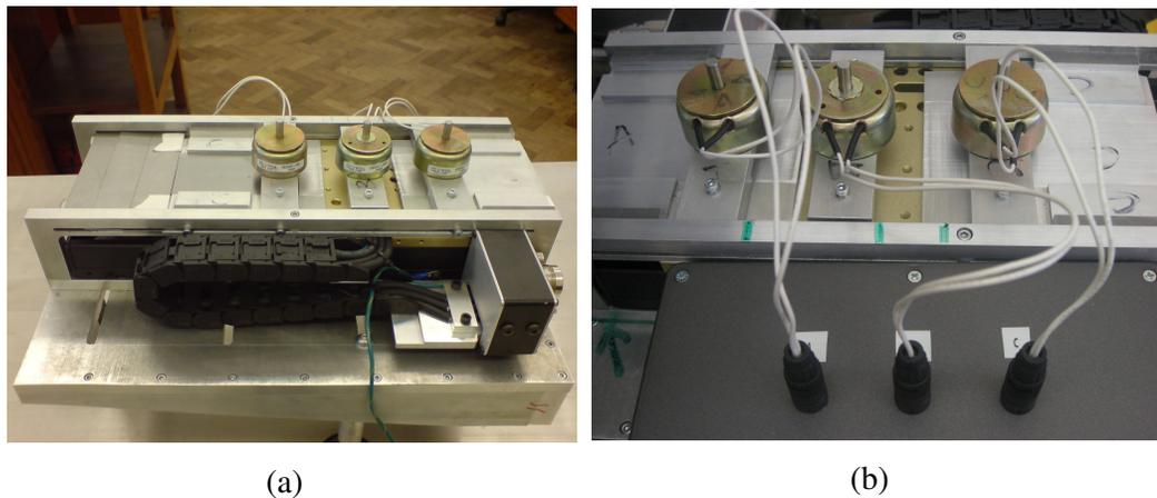
Fig. 8.7: (a) fully assembled frame; and (b) installed clamping solenoids.
