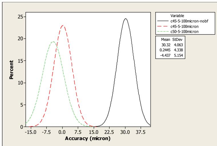
Fig. 4.26: Settled-positional accuracy-pattern for different motion-profile curves and the effect of brake force for CS100 strip at 5mm feed distance and 2Hz feed frequency.
