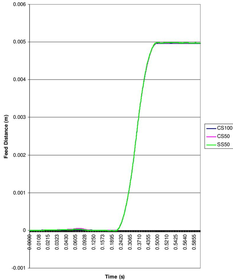
Fig. 4.9: Feeding characteristics for all strips for 5mm feed distance configured at 50-50 motion-profile with brake force at 1Hz feed frequency.
