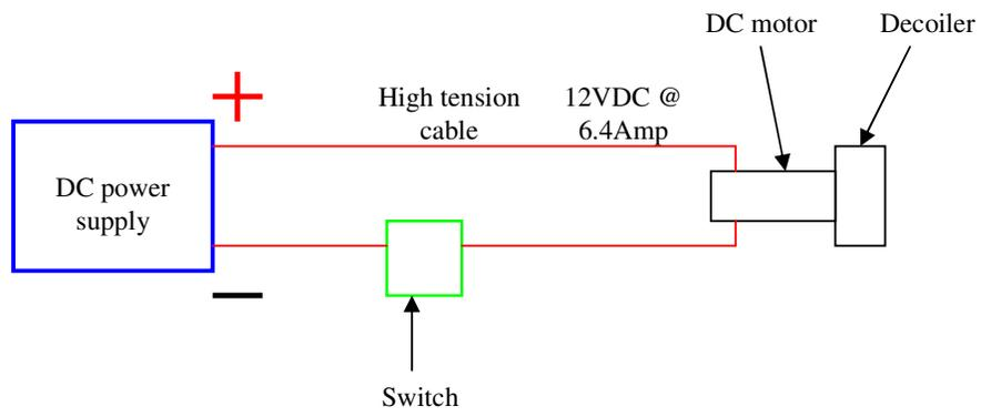
Fig. 9.4: Schematic diagram of the controlling brake force exerted by the DC motor on then uncoiler/decoiler.
