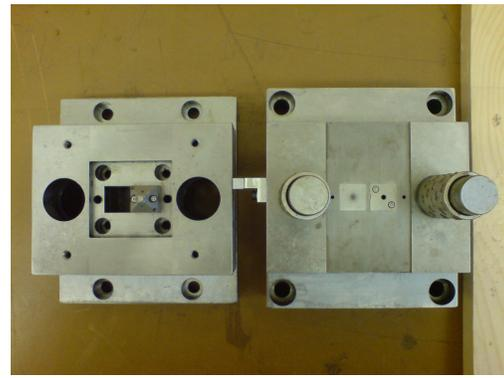
Fig. 2.9: Single-stage tool with a square punch and dies for micro-sheet-forming.
