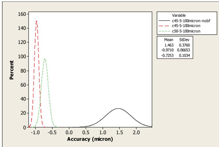
Fig. 7.24: Settled positional accuracy pattern for different motion profile curve and effect of brake force for CS100 strip at 5mm feed distance and 1Hz feed frequency.
