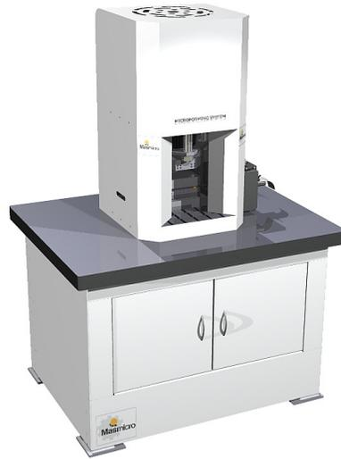
Fig. 2.8: A bench-top micro-sheet-forming machine, designed by the University of Strathclyde [Qin, 2009].
