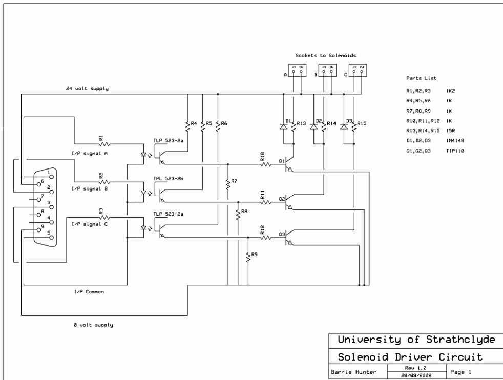
Fig. 8.13: Solenoid-driver circuit which uses an opto-coupler as a high-current switch-over relay.
