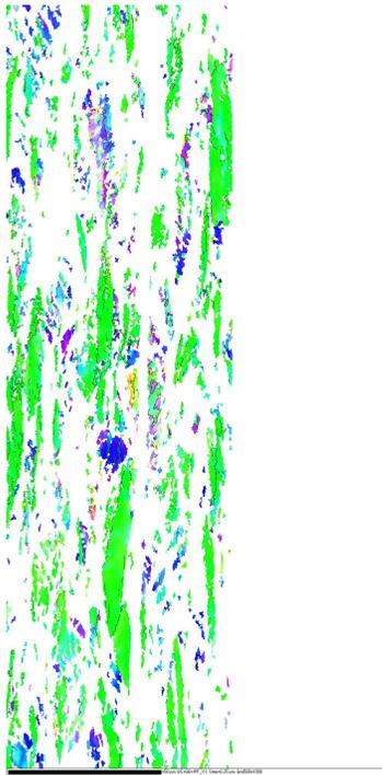
Fig. 3.22: EBSD mapping image of indexed  $>1\mu\text{m}$  grain size.
