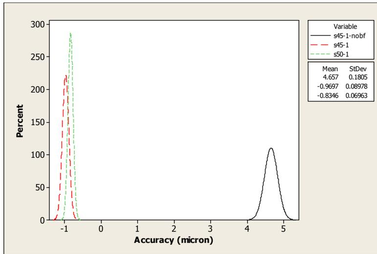
Fig. 7.20: Settled positional accuracy pattern for different motion profile curve and effect of brake force for SS50 strip at 1mm feed distance and 1Hz feed frequency.
