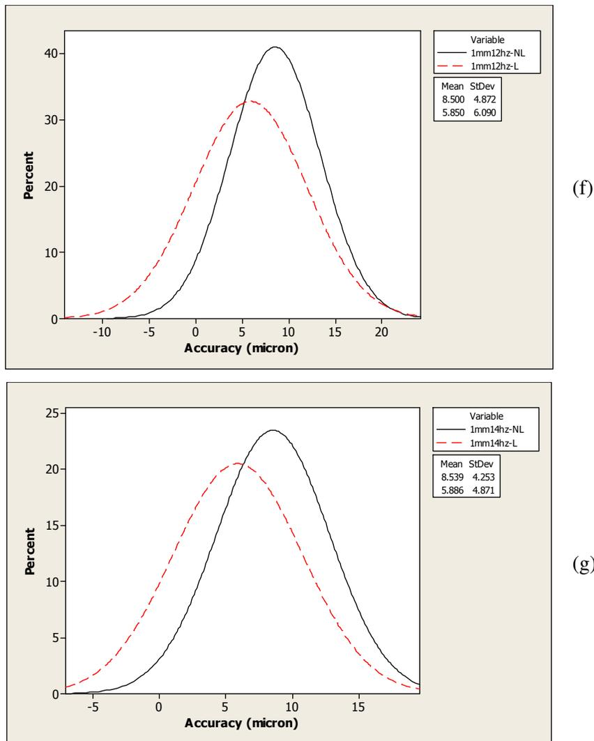
Fig. 5.13: Recorded positional accuracy for various feed-frequencies at 1mm feed-distance: (a) to (g) represent 1, 2, 3, 6, 9, 12 and 14Hz (representing all frequency-range cases).
