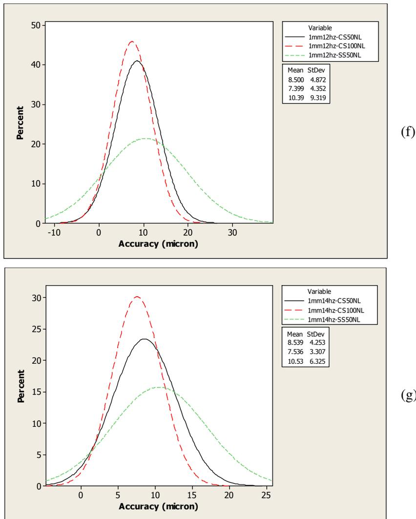
Fig. 5.15: Recorded positional accuracy for various materials in the non-lubrication case for all feed frequencies and at 1mm feed-distance: (a) to (g) represent feeding frequencies of 1-14Hz, respectively.
