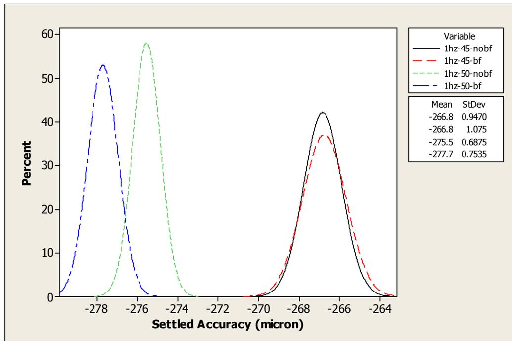
Fig. 10.17: The effect of brake-force for both motion-profiles at 1Hz feed-frequency.
