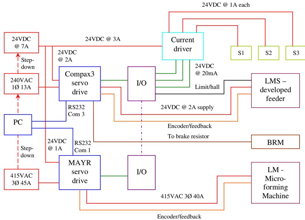
Fig. 8.12: Schematic diagram of the connections of the developed feeder with the micro-forming machine.
