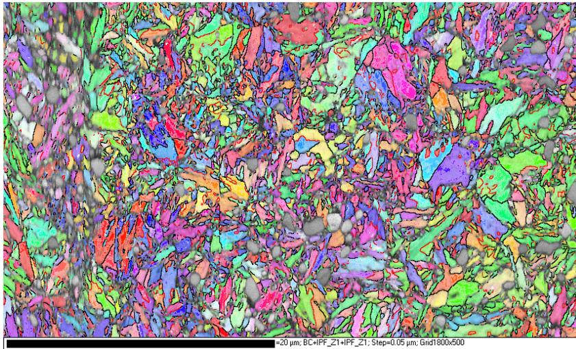
Fig. 3.18: EBSD microstructure-mapping image of CS100 strip.
