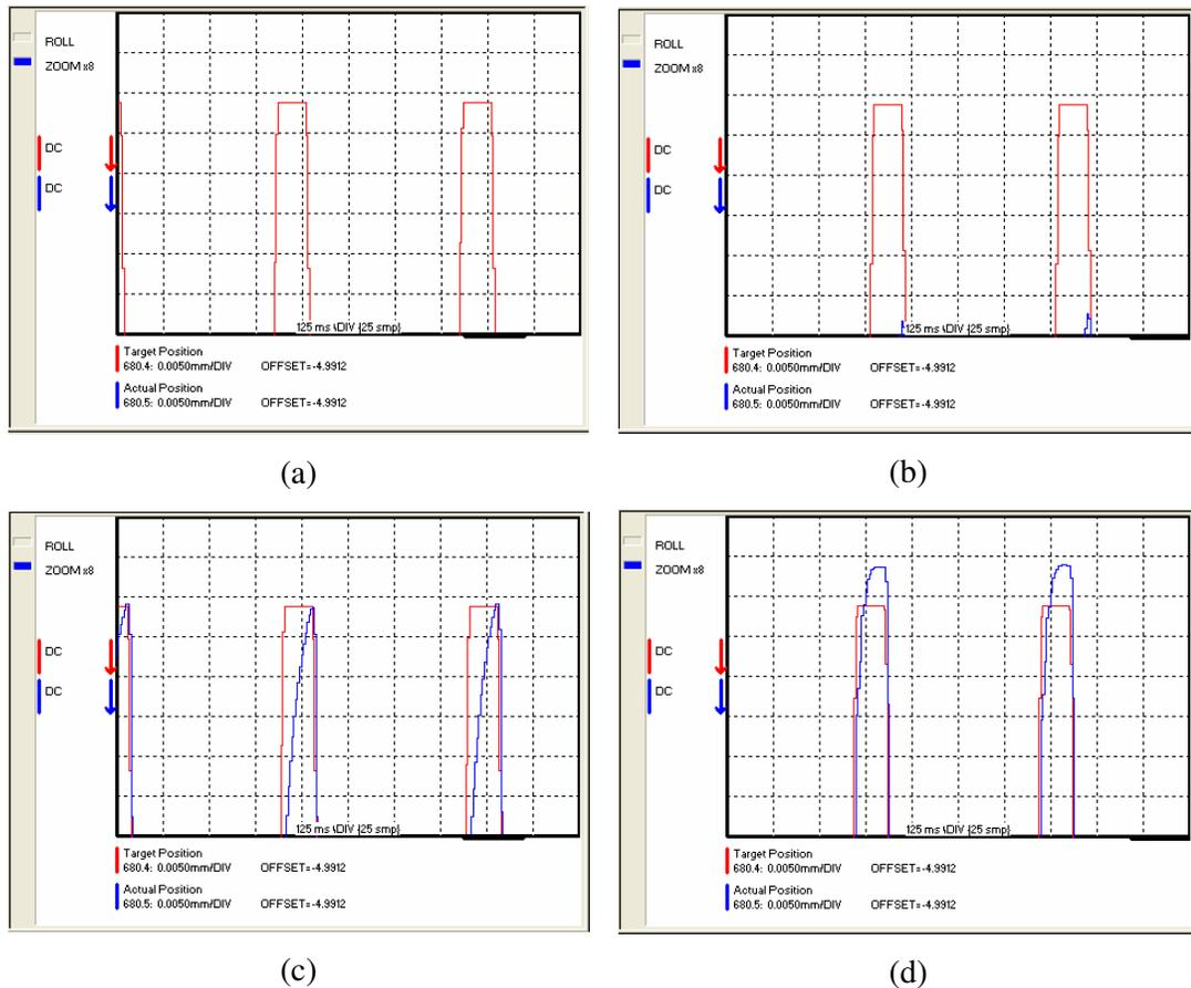
Fig. 9.5: Various load configurations tested for better positional accuracy: (a) 300g; (b) 1000g; (c) 1500g; and (d) 2300g.
