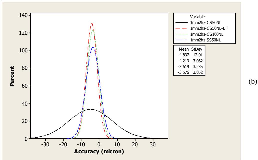
Fig. 5.19: Feeder performance at 1mm feed-distance for all tested strip-types and thicknesses: (a) 1Hz; and (b) 2Hz.
