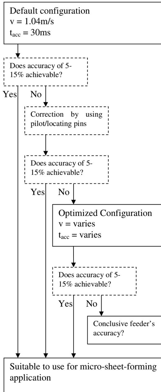
Fig. 5.7: Flowchart of the experiments' procedure.
