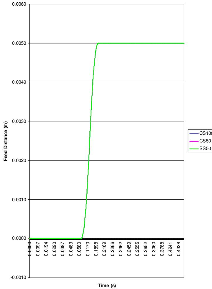
Fig. 7.15: Feeding characteristic for all strips for 5mm feed distance, 2Hz frequency configured at 50-50 motion profile with brake force.
