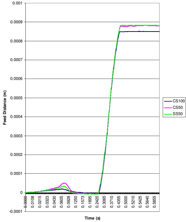
Fig. 4.8: Feeding characteristics for all strips for 1mm feed distance configured at 50-50 motion-profile with brake force at 1Hz feed frequency.
