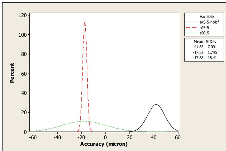
Fig. 4.27: Settled-positional accuracy-pattern for different motion-profile curves and the effect of brake force for SS50 strip at 5mm feed distance and 2Hz feed frequency.
