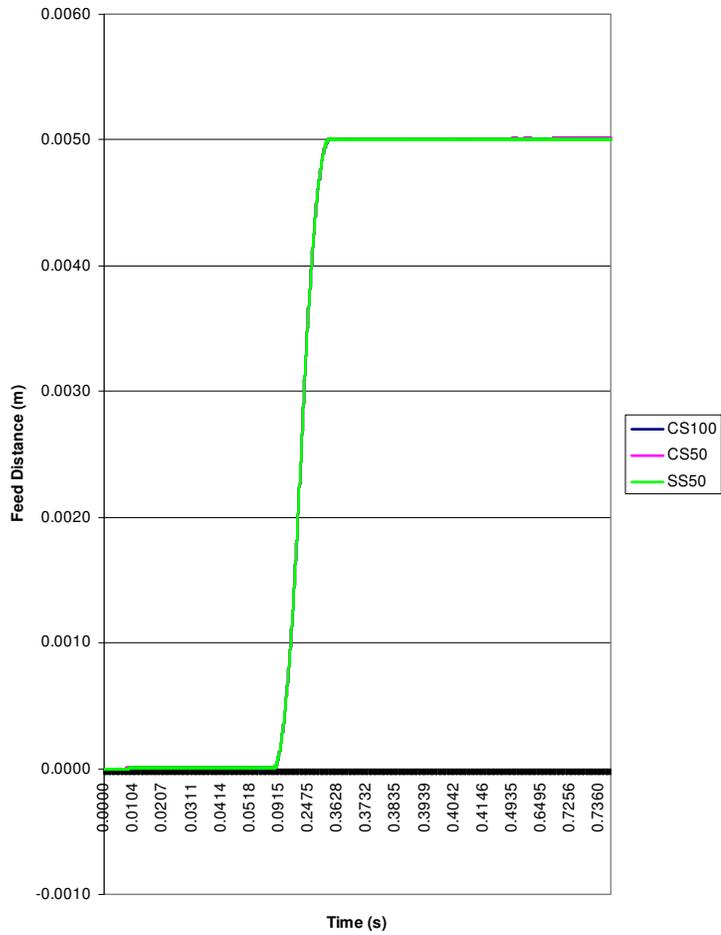
Fig. 7.6: Feeding characteristic for all strips for 5mm feed distance, 1Hz frequency configured at 45-45 motion profile without brake force.
