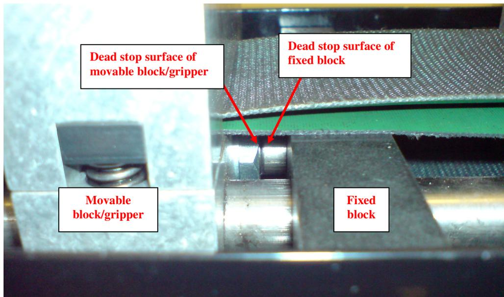
Fig. 5.28: The movable block hits the fixed block during feeding and gradually dislocates the fixed block.
