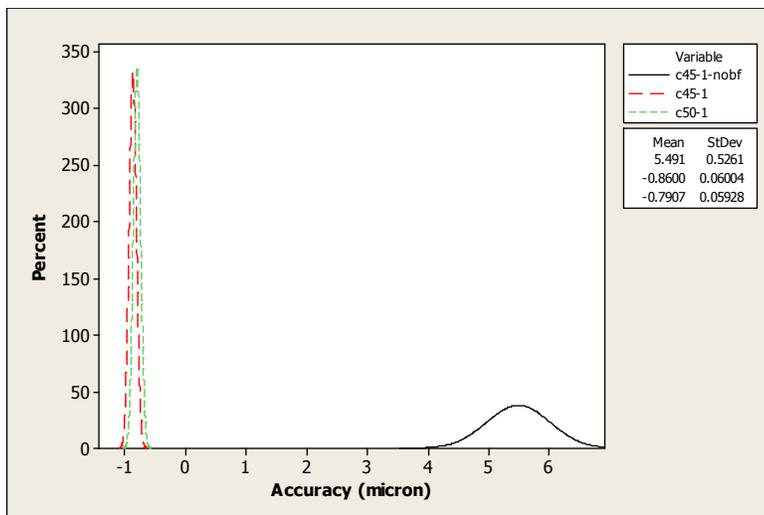
Fig. 7.17: Settled positional accuracy pattern for different motion profile curve and effect of brake force for CS50 strip at 1mm feed distance and 2Hz feed frequency.
