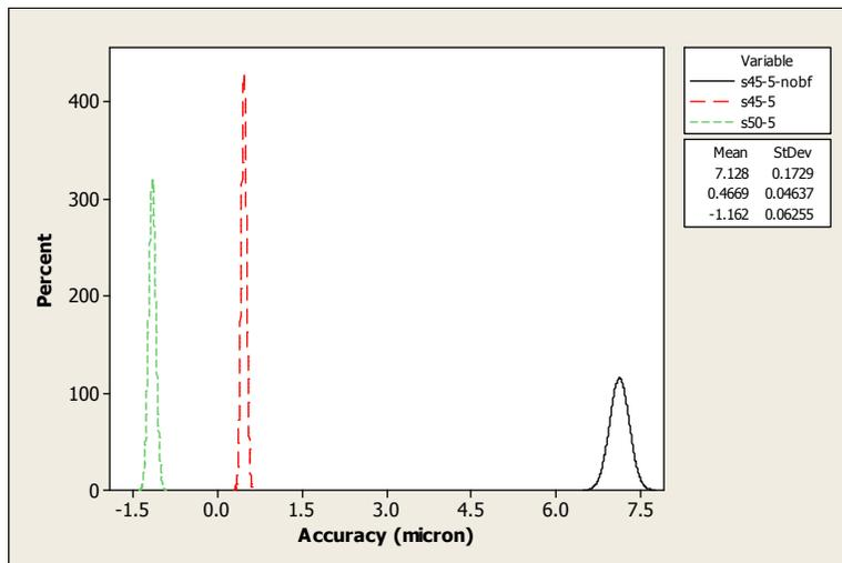
Fig. 7.26: Settled positional accuracy pattern for different motion profile curve and effect of brake force for SS50 strip at 5mm feed distance and 1Hz feed frequency.
