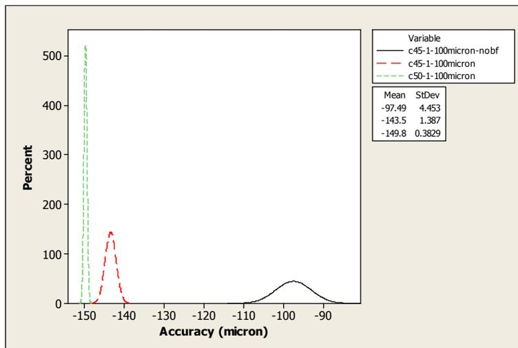
Fig. 4.17: Settled-positional accuracy-pattern for different motion-profiles curve and the effect of brake force for CS100 strip at 1mm feed distance and 1Hz feed frequency.
