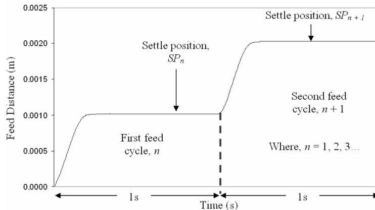
Fig. 5.9: Settling-time curve.
