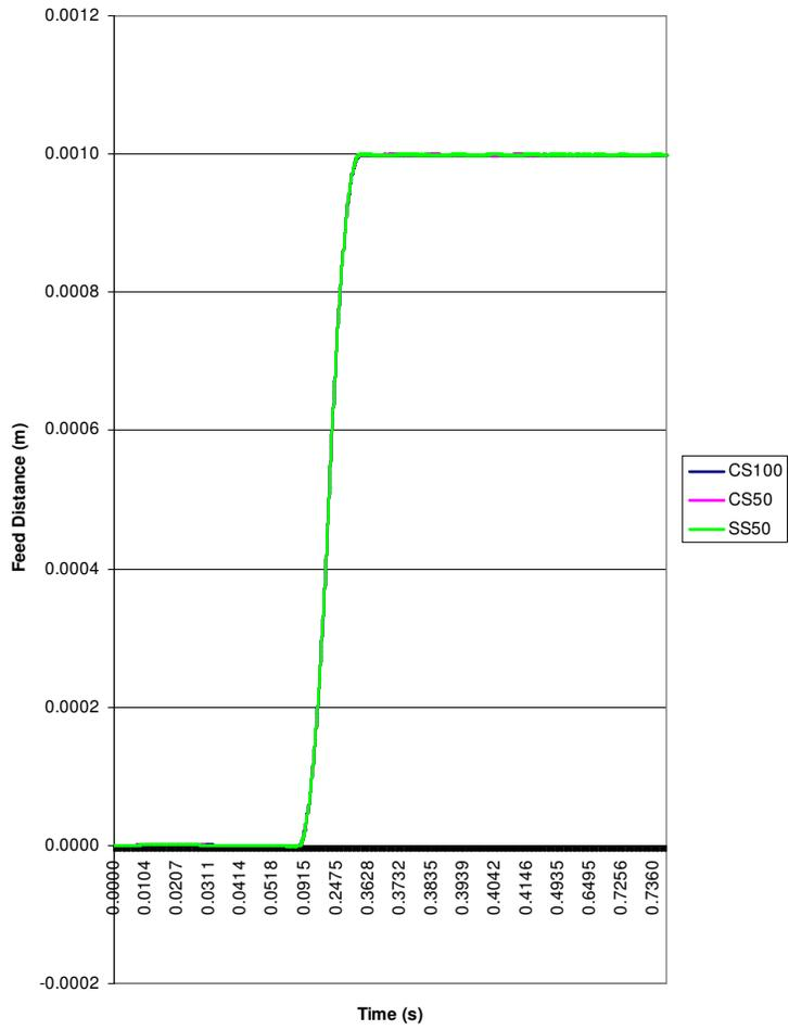
Fig. 7.12: Feeding characteristic for all strips for 1mm feed distance, 1Hz frequency configured at 50-50 motion profile with brake force.
