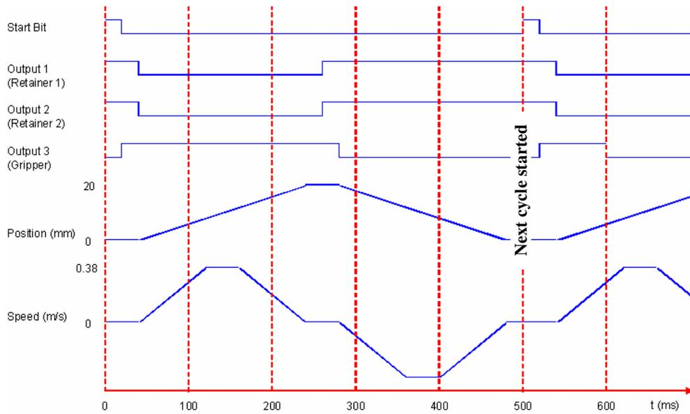
Fig. 8.9: Time-based control- and trigger-sequence.
