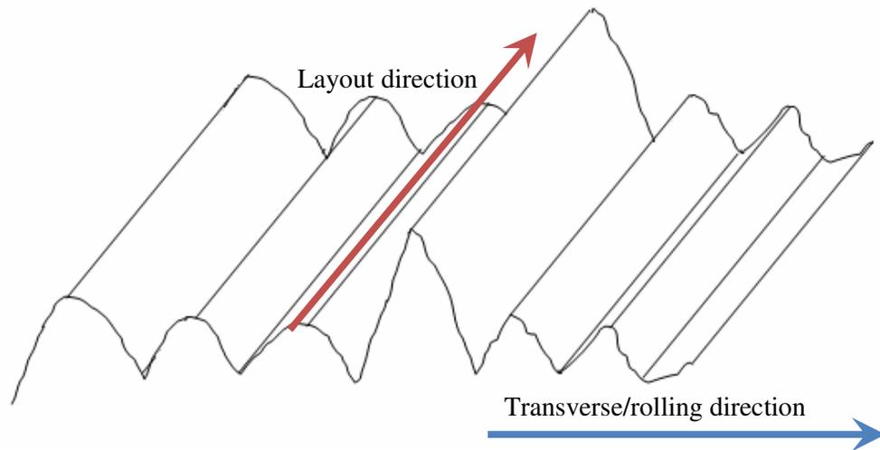
Fig. 3.23: Surface-roughness pattern.
