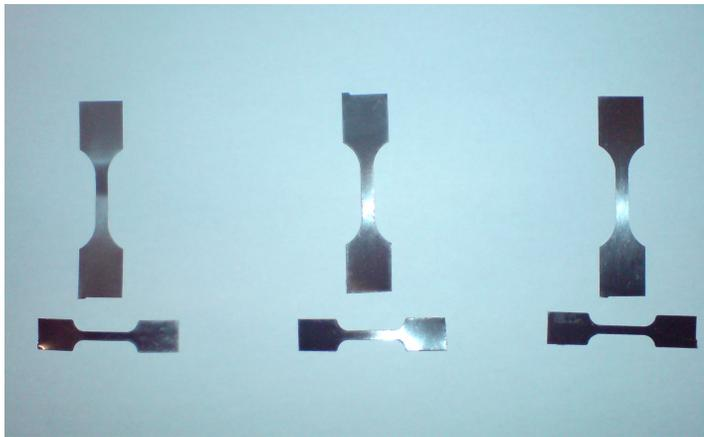
Fig. 3.4: Tensile testing specimens.
