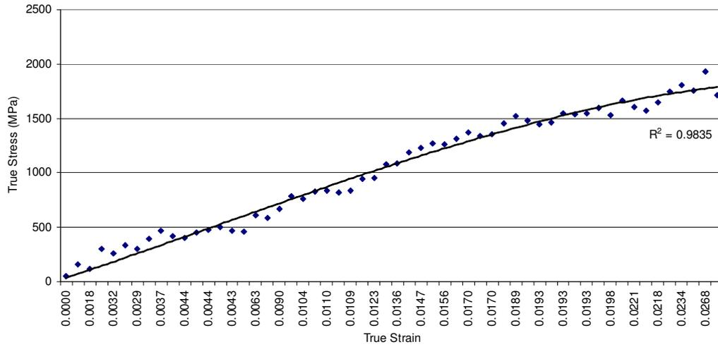
Fig. 3.9: Stress- (long stroke, not hyphen)strain curve for 50µm thick carbon steel strip in transverse direction.
