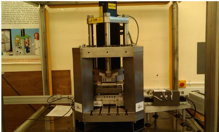
Fig. 10.1: Micro-forming machine developed at the University of Strathclyde.
