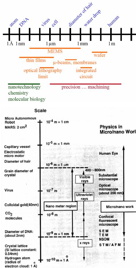
Fig. 2.1: Parts scales and dimensions [Kolesar et al., 2000].
