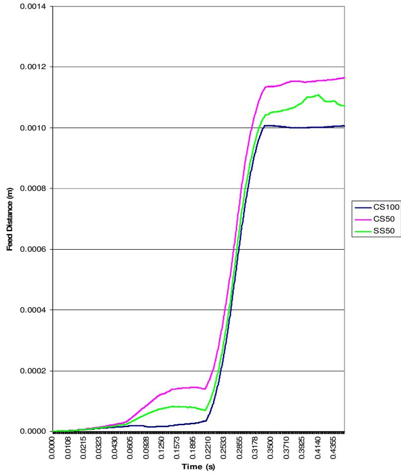
Fig. 4.10: Feeding characteristics for all strips for 1mm feed distance configured at 45-45 motion-profile without brake force at 2Hz feed frequency.
