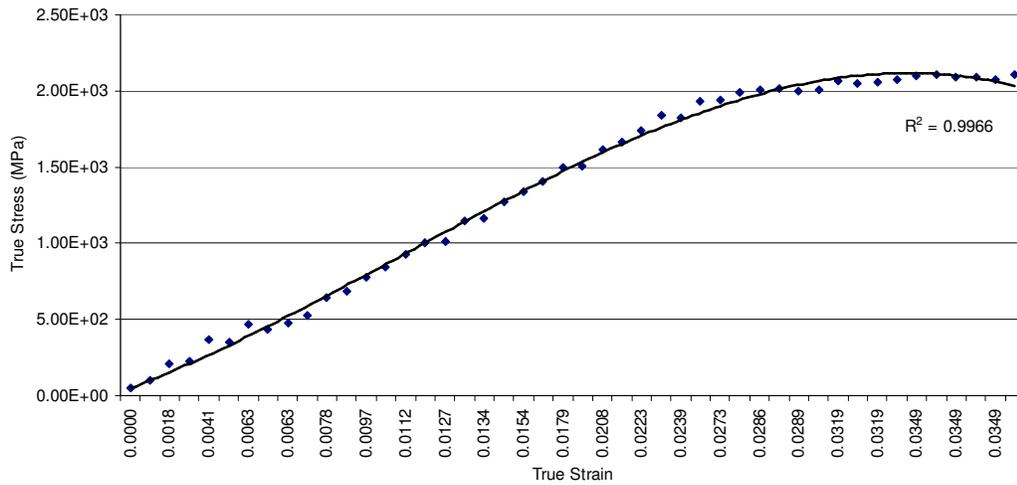
Fig. 3.10: Stress-(long stroke, not hyphen)strain curve for 50µm thick carbon steel strip in layout direction.
