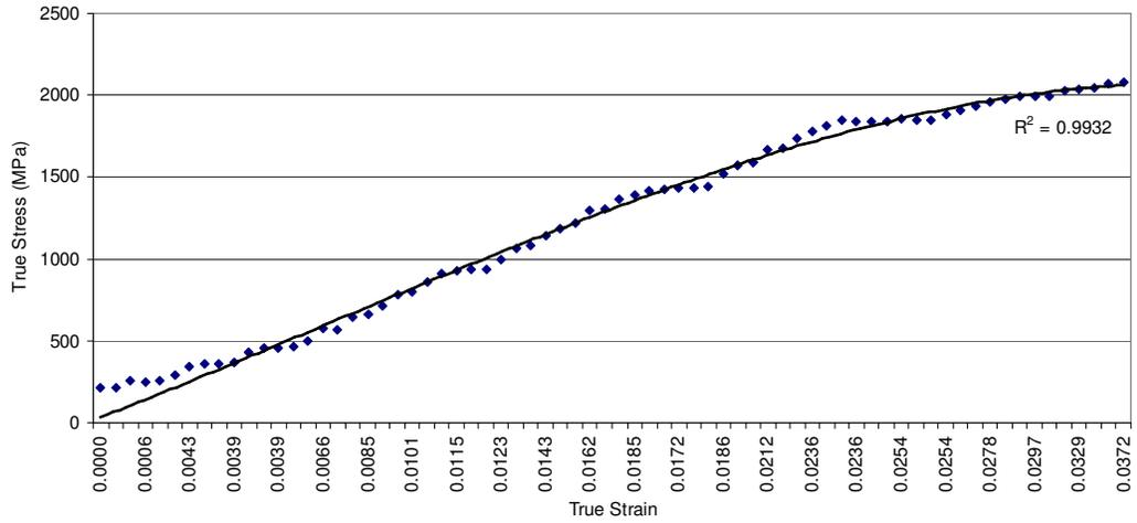
Fig: 3.11: Stress-(long stroke)strain curve for 100µm thick carbon steel strip in transverse direction.
