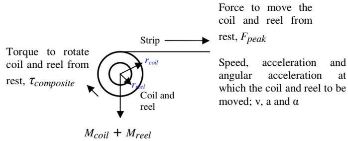
Fig. 6.5: Free-body diagram of the coil and reel producing a total of torque labelled as  $\tau_{composite}$ .
