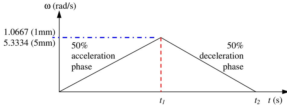
Fig. 4.3: Illustration of the 50-50 motion-profile curve
