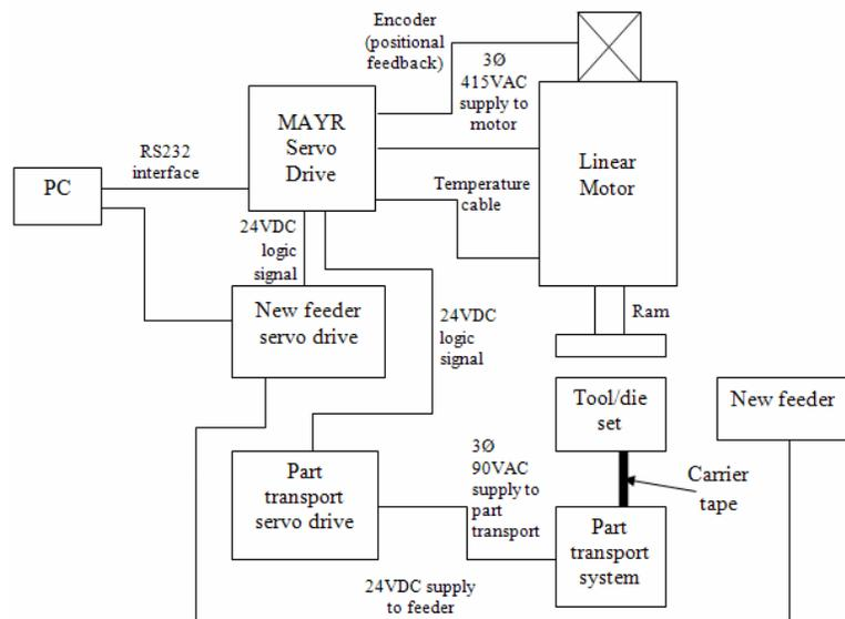
Fig. 10.4: Integrated feeder and part-transport system of the micro-sheet-forming machine.
