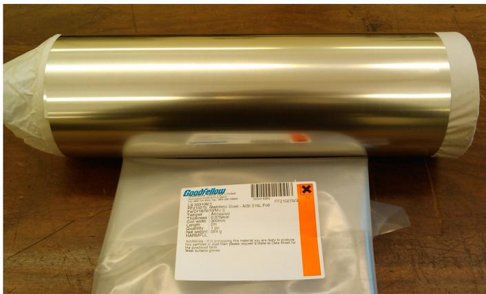
Fig. 10.3: Stainless-steel strip used for part-transport testing.
