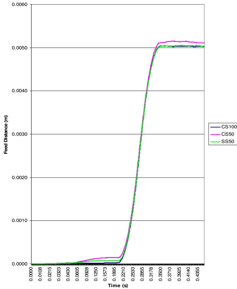
Fig. 4.11: Feeding characteristics for all strips for 5mm feed distance configured at 45-45 motion-profile without brake force at 2Hz feed frequency.
