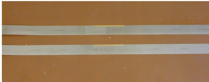
Fig. 5.5: 50 $\mu$ m and 100 $\mu$ m carbon-steel strip used in the experiments.
