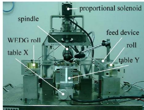
Fig. 2.6: Solenoid driven micro-forming machine [Chern et al., 2006a].
