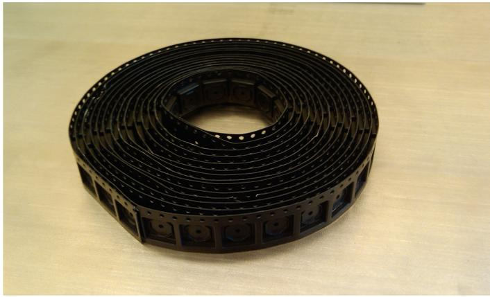
Fig. 10.2: Pocketed/embossed carrier-tape used for the tests.
