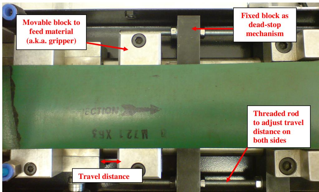
Fig. 5.27: Position of the movable/gripper and the fixed block of the pneumatic gripper-feeder.
