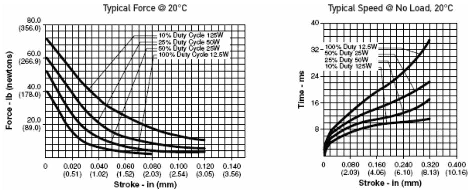
Fig. 8.5: Performance-chart force against stroke length, and stroke-length against response-time; of the flat-face-type solenoid [LEDEX].
