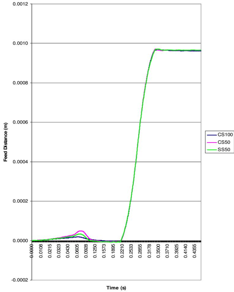
Fig. 4.14: Feeding characteristics for all strips for 1mm feed distance configured at 50-50 motion-profile with brake force at 2Hz feed frequency.
