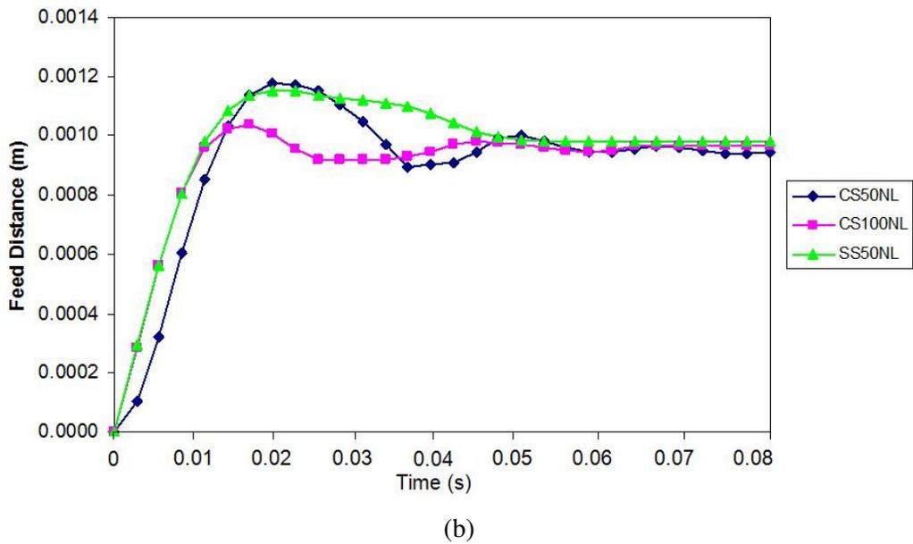
Fig. 5.25: Overshoot and settling-time at 1mm feed-distance for the non-lubricated case: (a) 1Hz; and (b) 2Hz feeding frequency.
