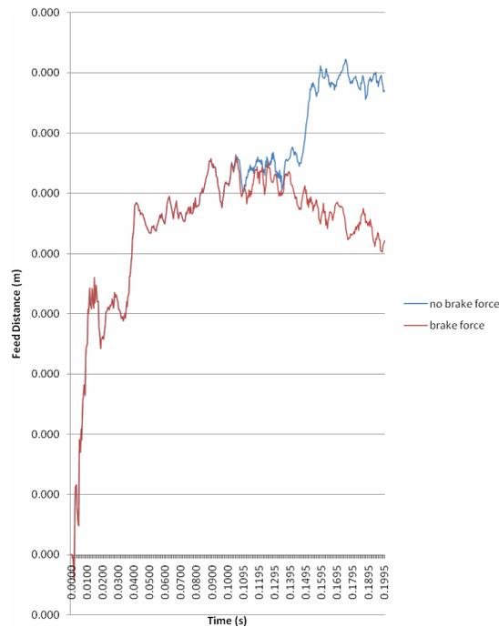
Fig. 10.13: FE analysis results for the preliminary step just before feeding starts for 2Hz feed-frequency and 45-45 motion-profile.
