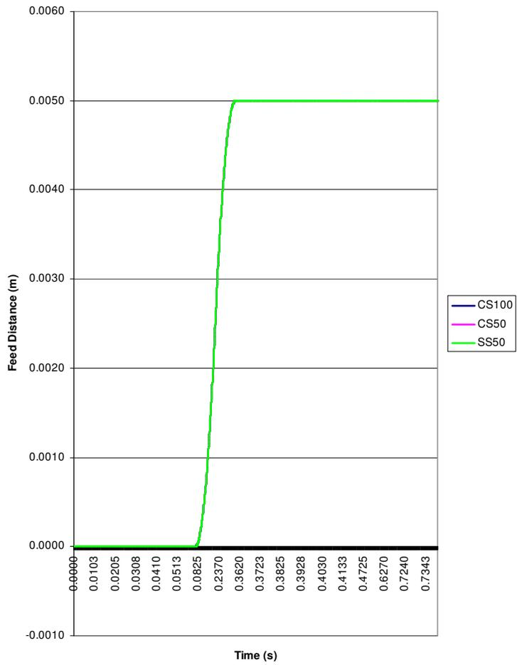
Fig. 7.14: Feeding characteristic for all strips for 5mm feed distance, 1Hz frequency configured at 50-50 motion profile with brake force.
