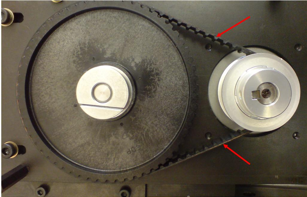
Fig. 5.22: The red arrows show irregularities on the servo roll-feeder drive-belt. A clear difference in belt composition can be seen between A and B.
