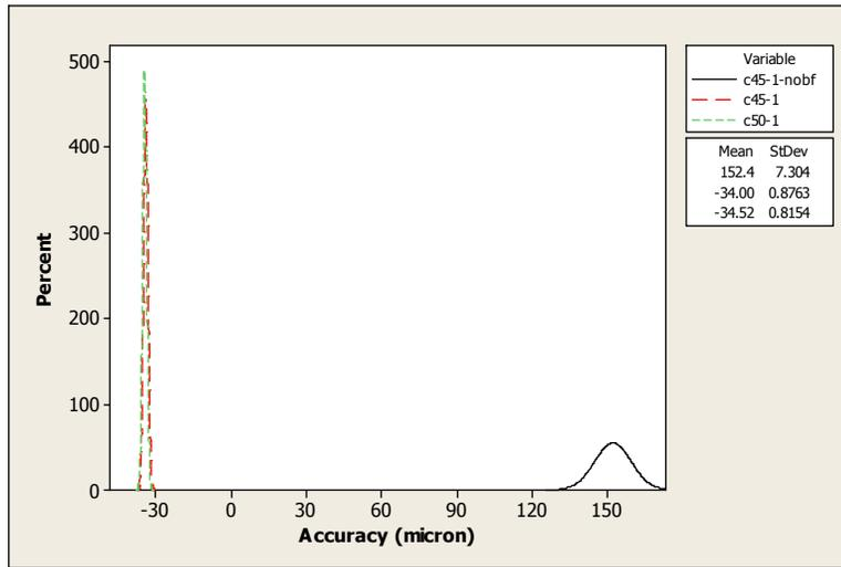
Fig. 4.19: Settled-positional accuracy-pattern for different motion-profile curves and the effect of brake force for CS50 strip at 1mm feed distance and 2Hz feed frequency.
