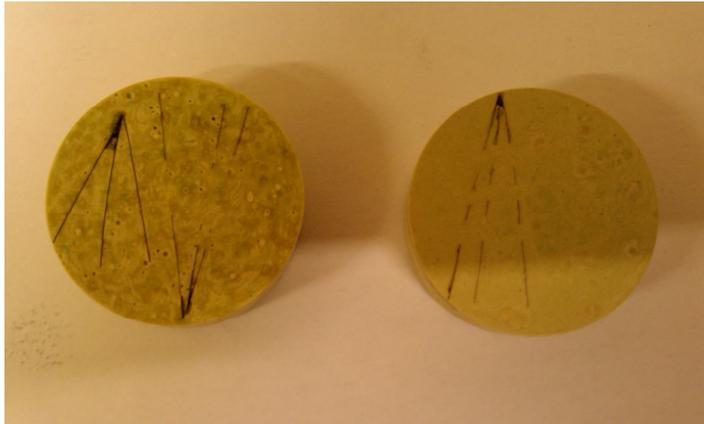
Fig. 3.6: Prepared EBSD specimens.
