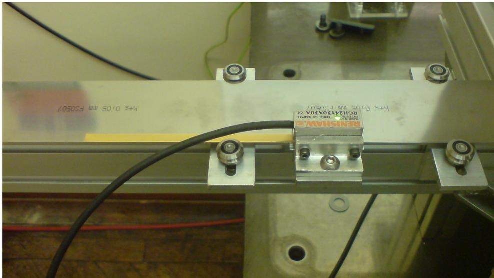
Fig. 5.4: Installation of the linear encoder on the machine structure.
