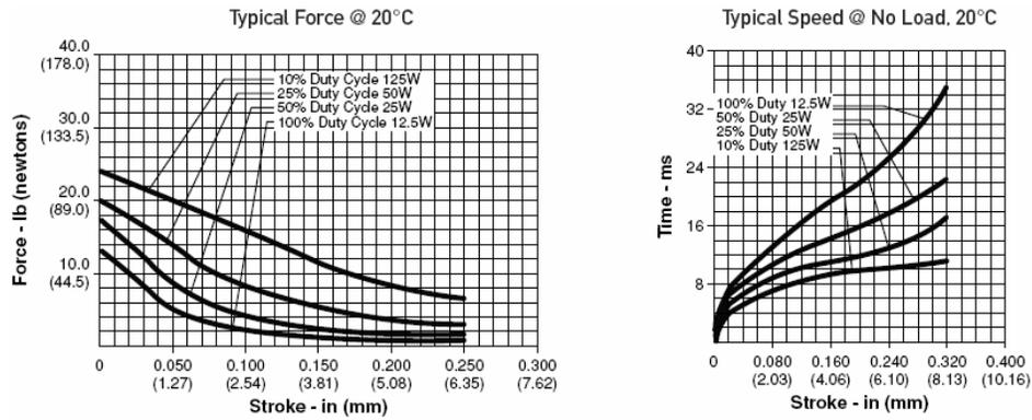
Fig. 8.4: Performance-chart force against stroke-length; and stroke-length against response-time; of the conical-Face-type solenoid [LEDEX].
