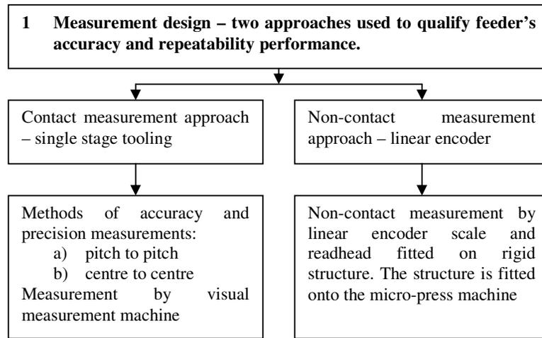
Fig. 2.16: Two approaches used to determine feeder performance: contact and non-contact methods.
