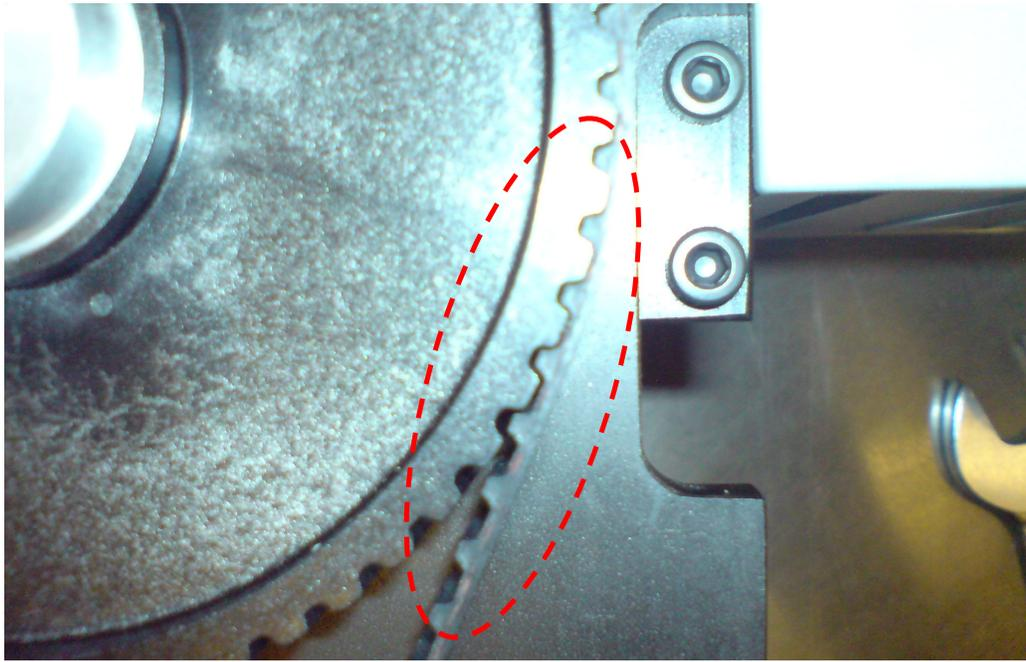
Fig. 5.24: Clearance between the pulley's teeth and the belt's grooves, which does contribute to positional inaccuracies.
