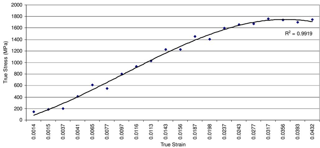
Fig: 3.14: Stress-(long stroke) strain curve for 50µm thick stainless steel strip in layout direction.
