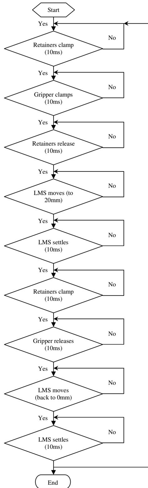
Fig. 8.8: Cycle-sequence flowchart for the feeding process.
