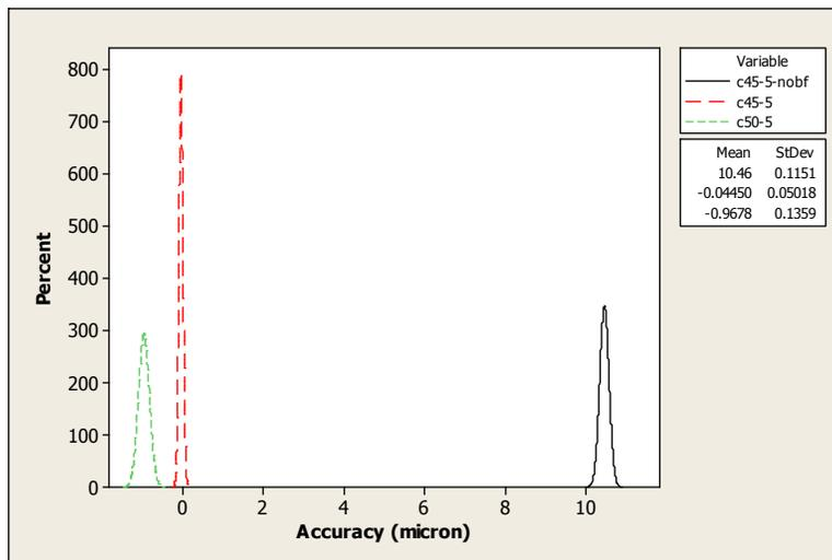
Fig. 7.22: Settled positional accuracy pattern for different motion profile curve and effect of brake force for CS50 strip at 5mm feed distance and 1Hz feed frequency.
