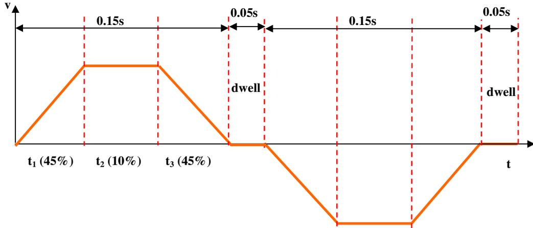
Fig. 6.4: Trapezoidal profile representing the acceleration of the forcer in one cycle.
