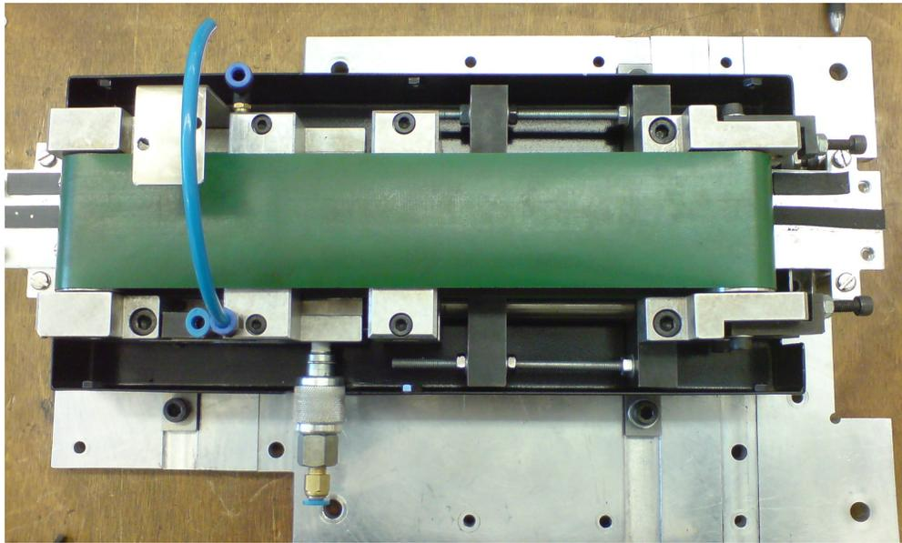
Fig. 5.3: The air gripper-feeder used in the experiments.
