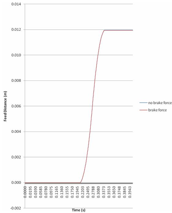
Fig. 10.16: Feed characteristics for 2Hz feed-frequency and 50-50 motion-profile.
