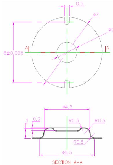
Fig. 1.1: Micro-hat design specification – part that is intended to be produced.
