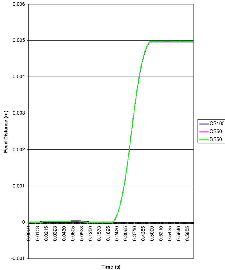
Fig. 4.7: Feeding characteristics for all strips for 5mm feed distance configured at 45-45 motion-profile with brake force at 1Hz feed frequency.
