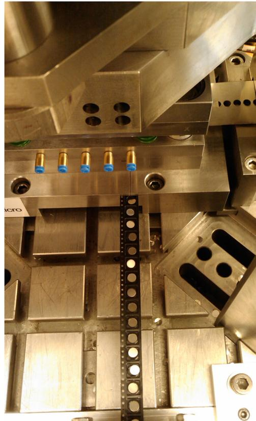
Fig. 10.20: Collection of parts/products at 2Hz feed-frequency.
