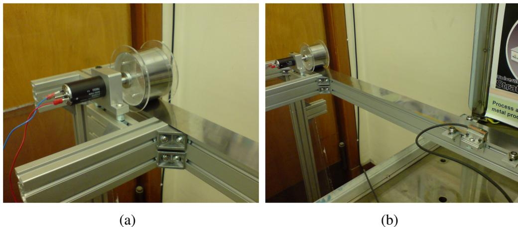
Fig. 9.3: (a) the DC motor is used to generate brake-force which is transferred to and acts on the reel; and (b) the whole brake-force and linear-encoder system.
