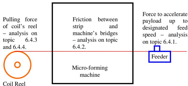
Fig: 6.2: Types of related forces, friction between parts and payloads that contribute to total peak- and continuous-forces calculation.
