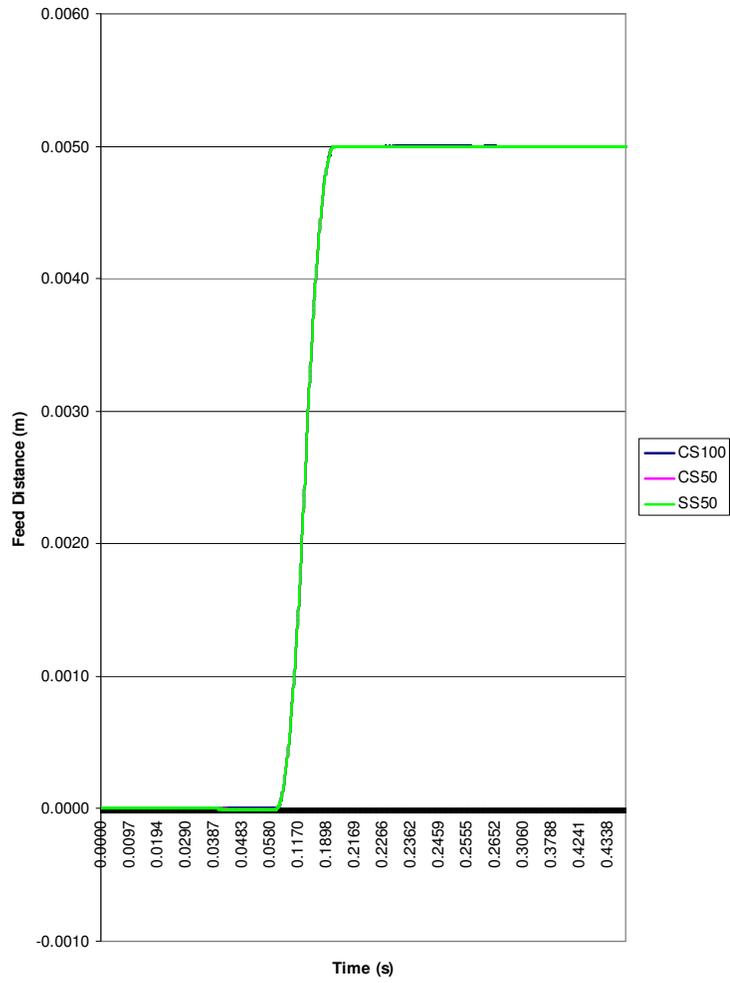
Fig. 7.11: Feeding characteristic for all strips for 5mm feed distance, 2Hz frequency configured at 45-45 motion profile with brake force.
