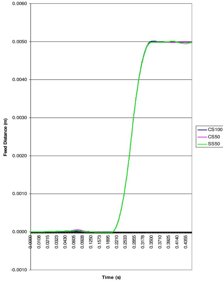
Fig. 4.15: Feeding characteristics for all strips for 5mm feed distance configured at 50-50 motion-profile with brake force at 2Hz feed frequency.
