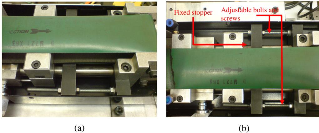
Fig. 2.15: Showing: (a) a pneumatic gripper feeder; and (b) the location of adjustment screws and bolts to change feed distance.
