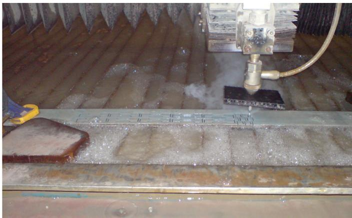
Fig. 3.5: Abrasive water-jet cutting used to prepare the specimens.
