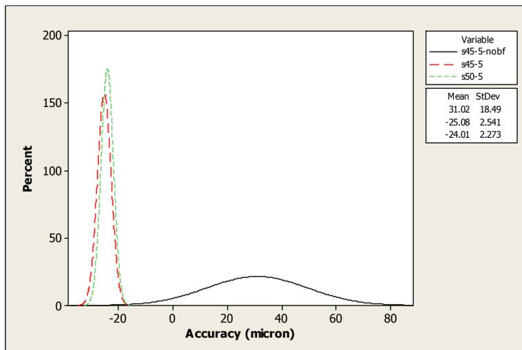
Fig. 4.24: Settled-positional accuracy-pattern for different motion-profile curves and the effect of brake force for SS50 strip at 5mm feed distance and 1Hz feed frequency.
