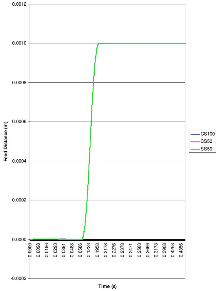
Fig. 7.9: Feeding characteristic for all strips for 1mm feed distance, 2Hz frequency configured at 45-45 motion profile with brake force.
