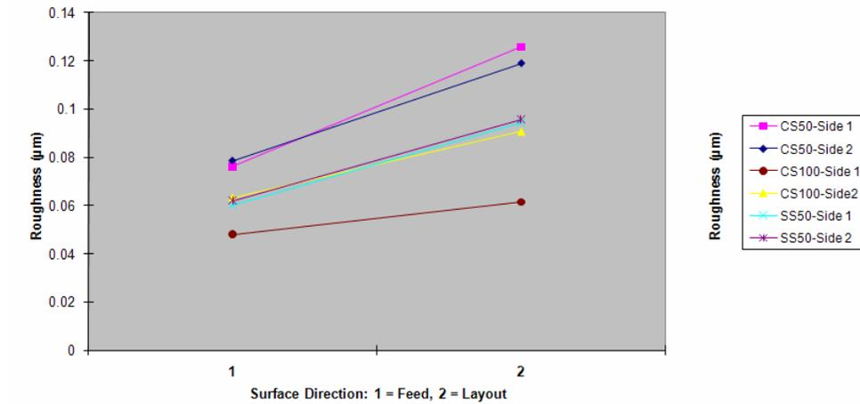
Fig. 3.8: Measured surface-roughness of strip materials.
