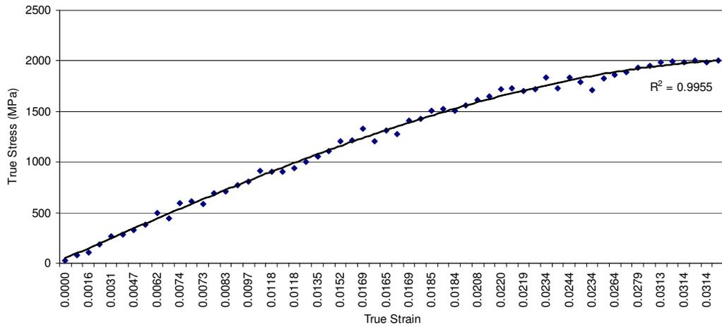
Fig: 3.12: Stress-(long stroke)strain curve for 100µm thick carbon steel strip in layout direction.
