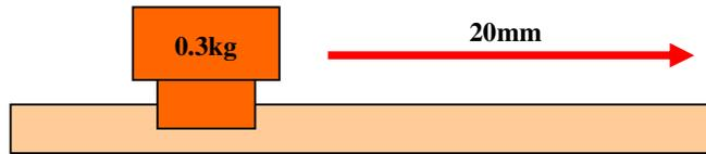
Fig. 6.3: Diagram of the load exerted on the forcer, and the direction and distance of movement.
