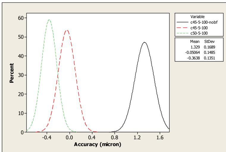
Fig. 7.25: Settled positional accuracy pattern for different motion profile curve and effect of brake force for CS100 strip at 5mm feed distance and 2Hz feed frequency.
