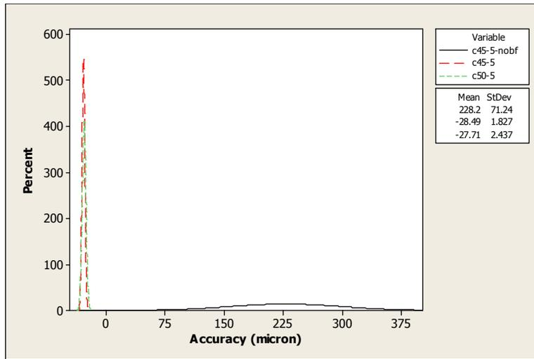
Fig. 4.22: Settled-positional accuracy-pattern for different motion-profile curves and the effect of brake force for CS50 strip at 5mm feed distance and 1Hz feed frequency.
