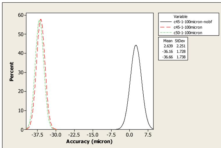
Fig. 4.20: Settled-positional accuracy-pattern for different motion-profile curves and the effect of brake force for CS100 strip at 1mm feed distance and 2Hz feed frequency.
