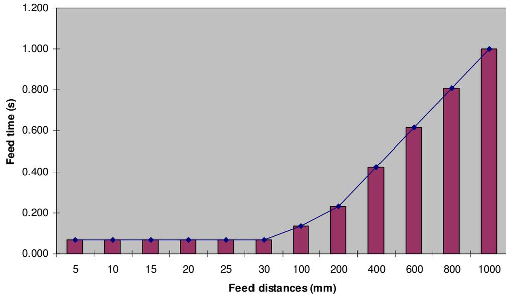
Fig. 5.2: Feeder feeding-performance.
