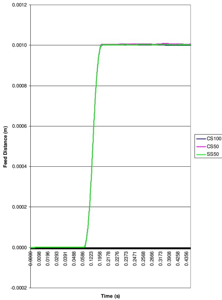
Fig. 7.5: Feeding characteristic for all strips for 1mm feed distance, 2Hz frequency configured at 45-45 motion profile without brake force.
