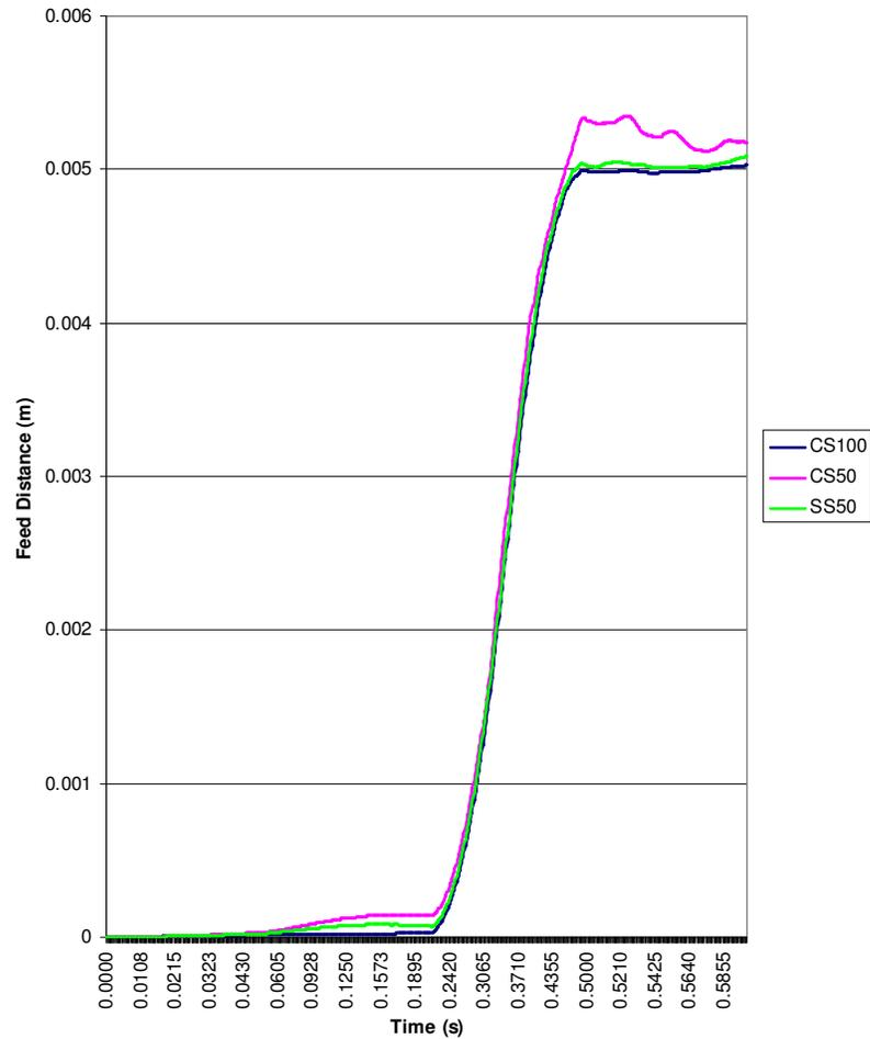
Fig. 4.5: Feeding characteristics for all strips for 5mm feed distance configured at 45-45 motion-profile without brake force at 1Hz feed frequency.
