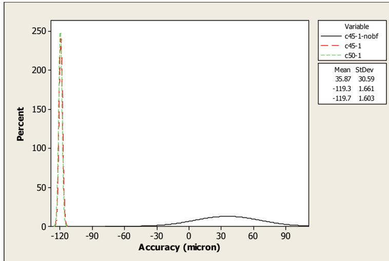
Fig. 4.16: Settled-positional accuracy-pattern for different motion-profile curves and the effect of brake force for CS50 strip at 1mm feed distance and 1Hz feed frequency.
