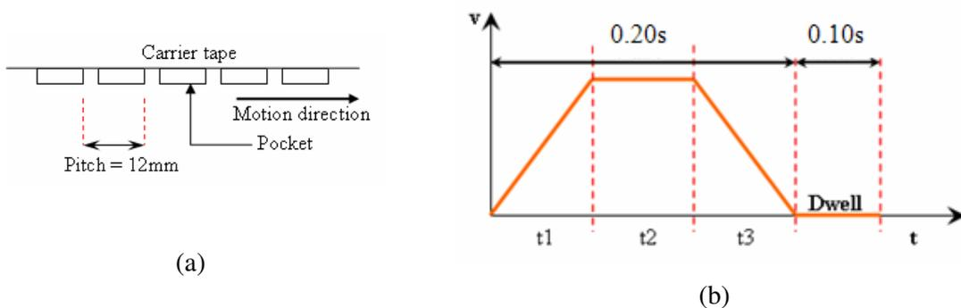
Fig. 10.7: (a) the load exerted on the forcer, and the direction and distance of movement, and (b) trapezoidal profile representing the acceleration and deceleration of the coiler in one cycle.
