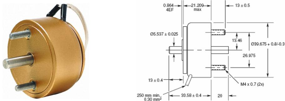
Fig. 8.3: (a) the solenoid used, and (b) solenoid dimensions [LEDEX].
