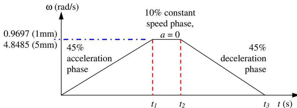
Fig. 4.2: Illustration of the 45-45 motion-profile curve.
