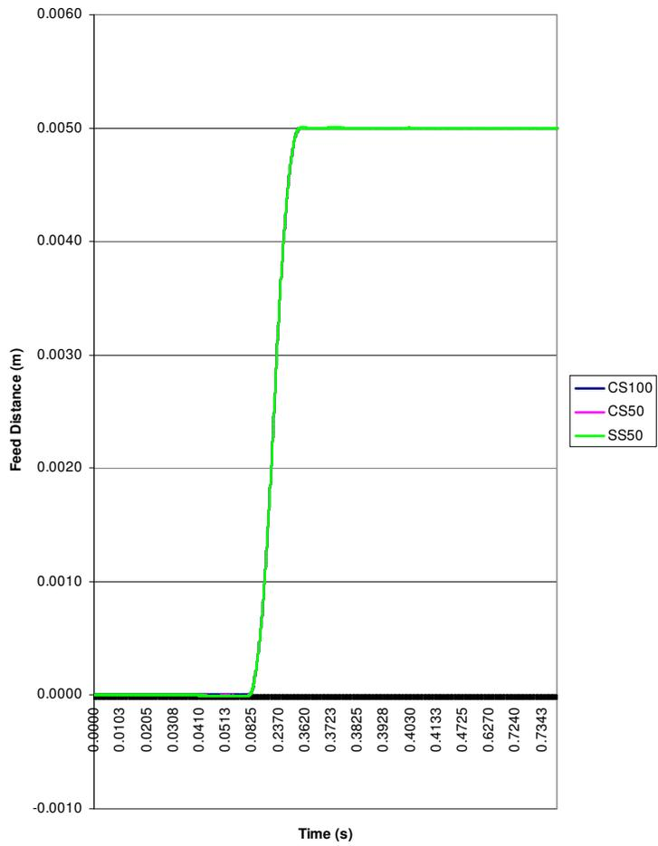
Fig. 7.10: Feeding characteristic for all strips for 5mm feed distance, 1Hz frequency configured at 45-45 motion profile with brake force.
