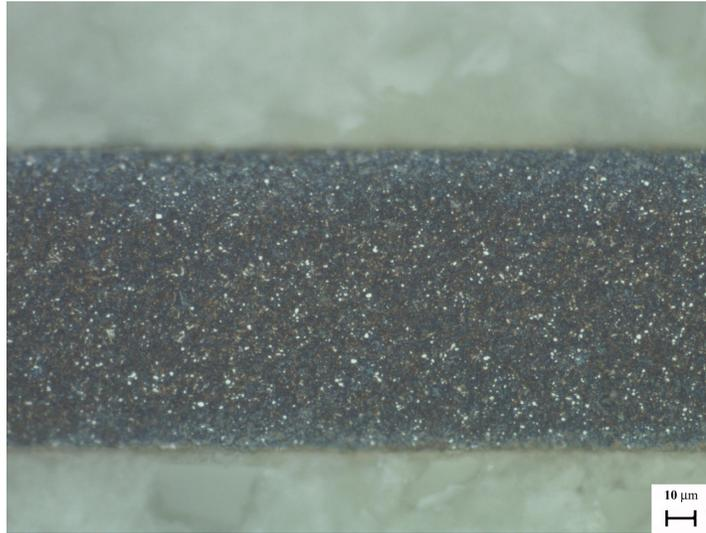
Fig. 3.17: Light-microscopy image of CS100 strip at 500x magnification with cementite shown (white colour).
