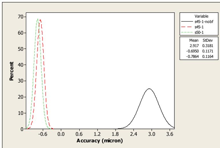
Fig. 7.21: Settled positional accuracy pattern for different motion profile curve and effect of brake force for SS50 strip at 1mm feed distance and 2Hz feed frequency.
