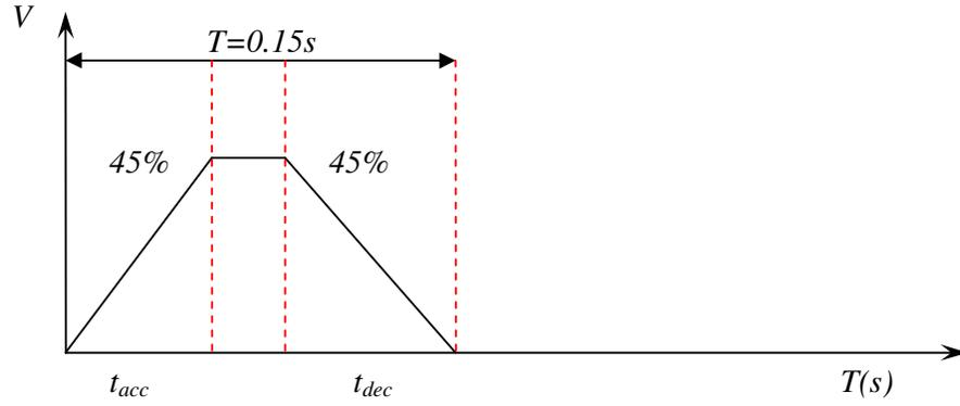
Fig. 9.2: Acceleration and deceleration time-frame for the 2Hz feeding-frequency motion-profile.
