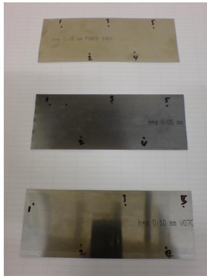
Fig. 3.7: Surface-roughness measuring point on each strip material.
