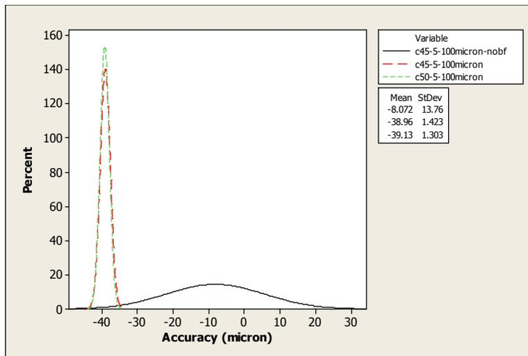
Fig. 4.23: Settled-positional accuracy-pattern for different motion-profile curves and the effect of brake force for CS100 strip at 5mm feed distance and 1Hz feed frequency.
