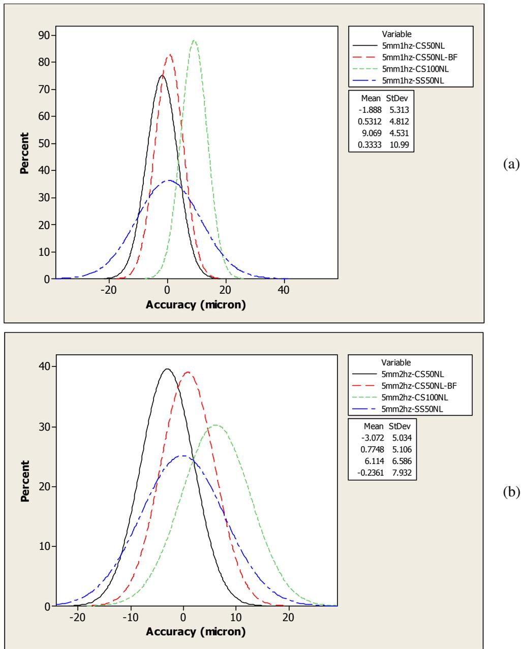
Fig. 5.20: Feeder performance at 5mm feed-distance for all tested strip-types and thicknesses: (a) 1Hz; and (b) 2Hz.
