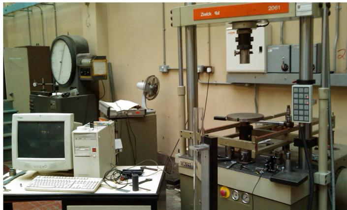
Fig. 3.2: Zwick REL universal testing machine Model 2061 used to determine material mechanical properties.
