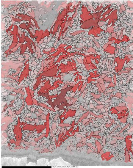
Fig. 3.16: EBSD microstructure mapping image of CS50 strip.
