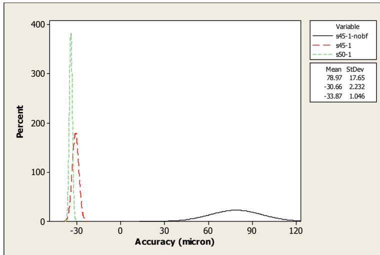
Fig. 4.21: Settled-positional accuracy-pattern for different motion-profile curves and the effect of brake force for SS50 strip at 1mm feed distance and 2Hz feed frequency.
