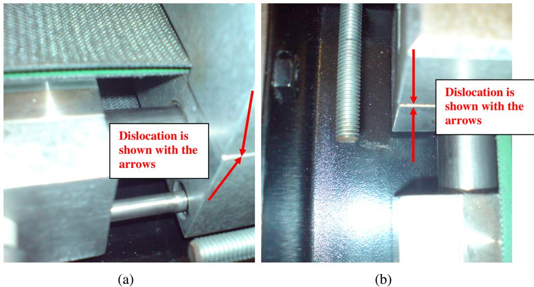
Fig. 5.29: Dislocation on both the right (a) and the left (b) of the movable block/gripper after several times of feeding.
