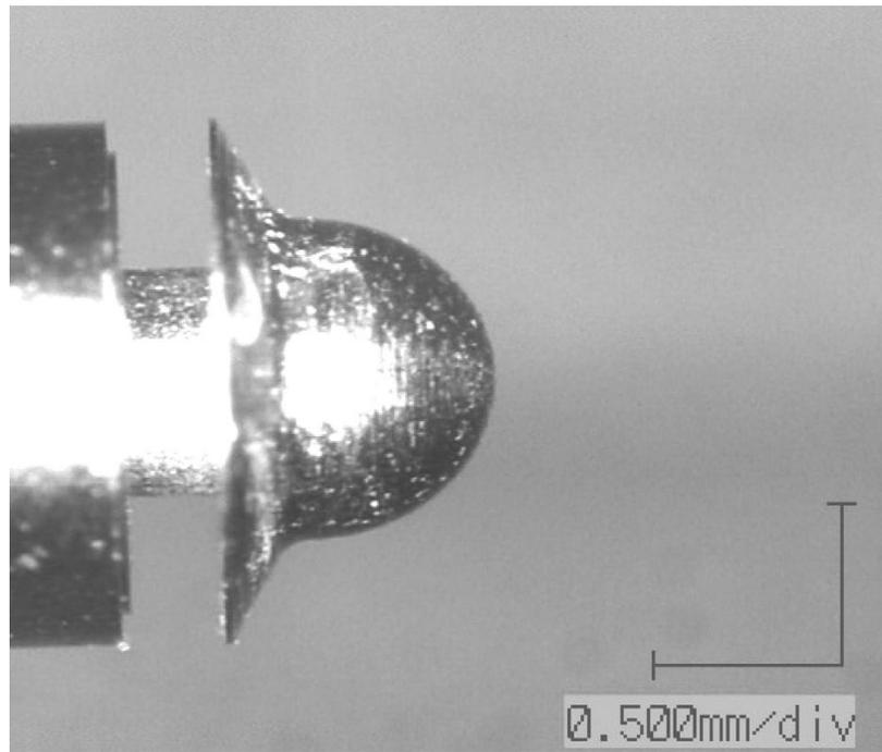
Fig. 2.3: Machined ‘microhat’ by MEL revised microlathe micro-machine [Okazaki et al., 2004].
