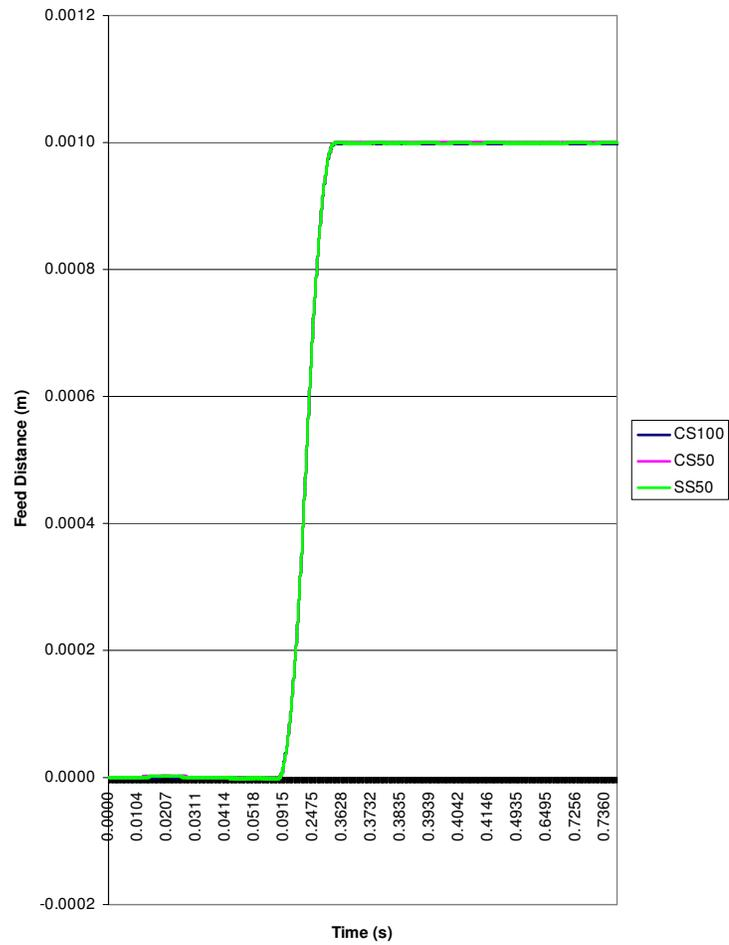
Fig. 7.8: Feeding characteristic for all strips for 1mm feed distance, 1Hz frequency configured at 45-45 motion profile with brake force.
