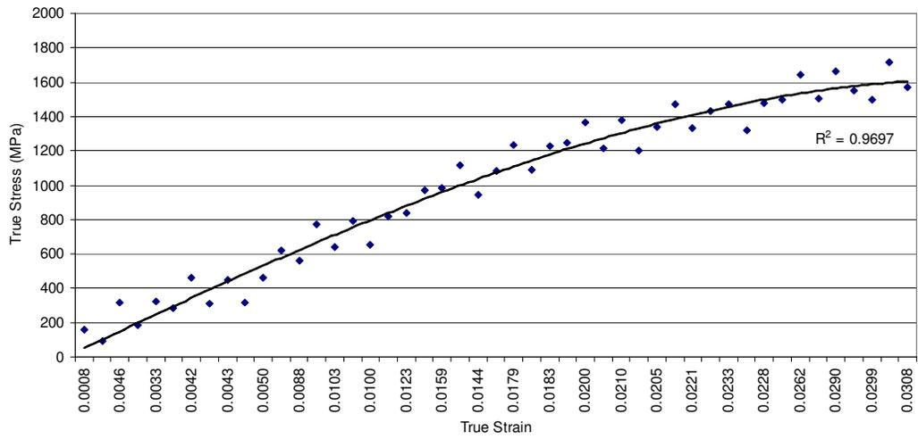
Fig: 3.13: Stress-(long stroke) strain curve for 50µm thick stainless steel strip in transverse direction.
