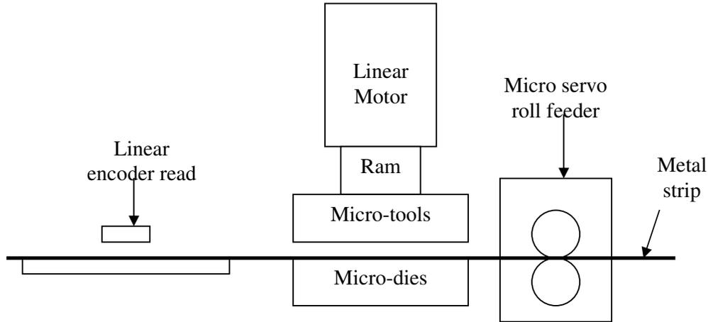
Fig. 5.8: Placement of the linear encoder on the machine and the experimental set-up.
