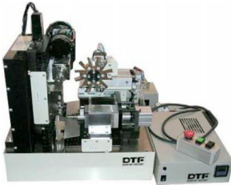
Fig. 2.4: Desktop turning centre developed by DTF Study Group.
