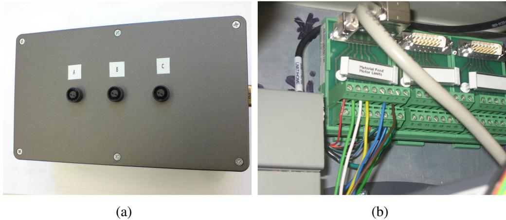
Fig. 8.14: (a) the solenoid driver circuit box uses an RS232 interface to communicate with the Compax3 servo-drive through an I/O terminal in (b): the 3 sockets connect the retainers and the gripper solenoids.
