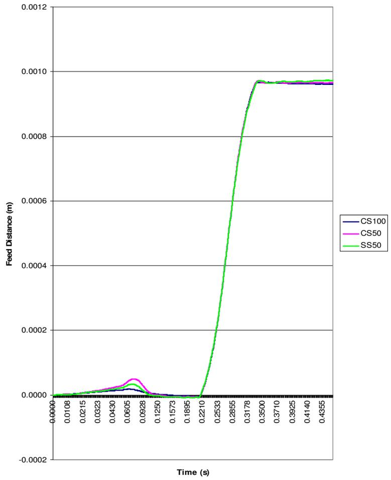
Fig. 4.12: Feeding characteristics for all strips for 1mm feed distance configured at 45-45 motion-profile with brake force at 2Hz feed frequency.
