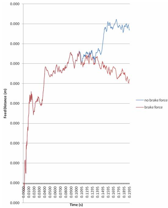
Fig. 10.14: FE analysis results for the preliminary step just before feeding starts for 2Hz feed-frequency and 50-50 motion-profile.
