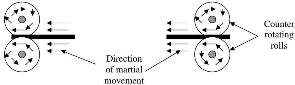
Fig. 2.12: Working principle of the roll feeder.
