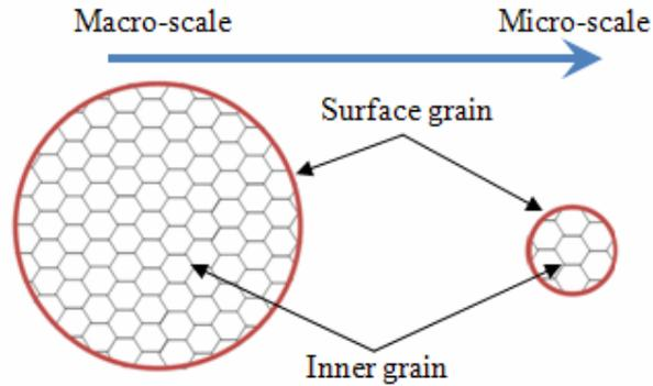
Fig. 3.24: Grain distribution in a material section of different material/feature size.
