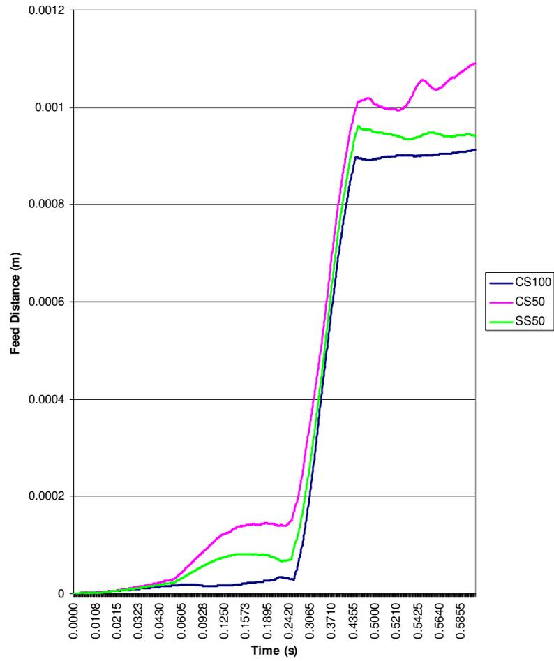
Fig. 4.4: Feeding characteristics for all strips for 1mm feed distance configured at 45-45 motion-profile without brake force at 1Hz feed frequency.
