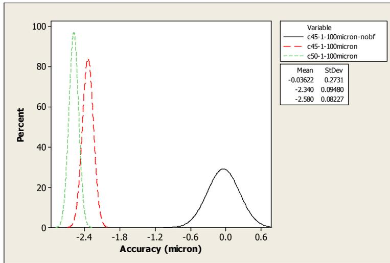
Fig. 7.18: Settled positional accuracy pattern for different motion profile curve and effect of brake force for CS100 strip at 1mm feed distance and 1Hz feed frequency.
