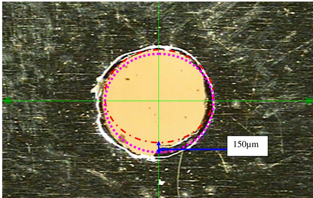
Fig. 5.18: A deformed locating-pin hole.
