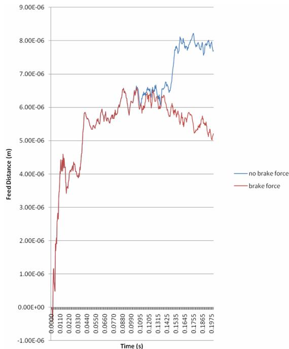
Fig. 10.9: FE analysis results for the preliminary step just before feeding starts for 1Hz feed-frequency and 45-45 motion-profile.
