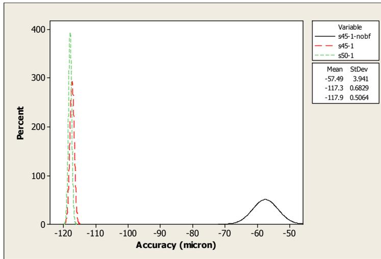
Fig. 4.18: Settled-positional accuracy-pattern for different motion-profile curves and the effect of brake force for SS50 strip at 1mm feed distance and 1Hz feed frequency.
