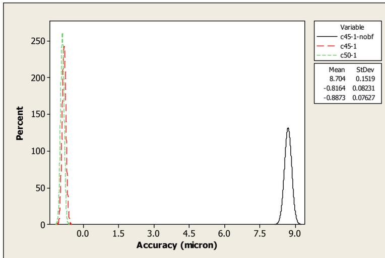
Fig. 7.16: Settled positional accuracy pattern for different motion profile curve and effect of brake force for CS50 strip at 1mm feed distance and 1Hz feed frequency.
