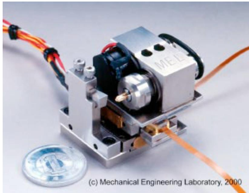
Fig. 2.2: Micro lathe with numerical control [Okazaki et al., 2004].
