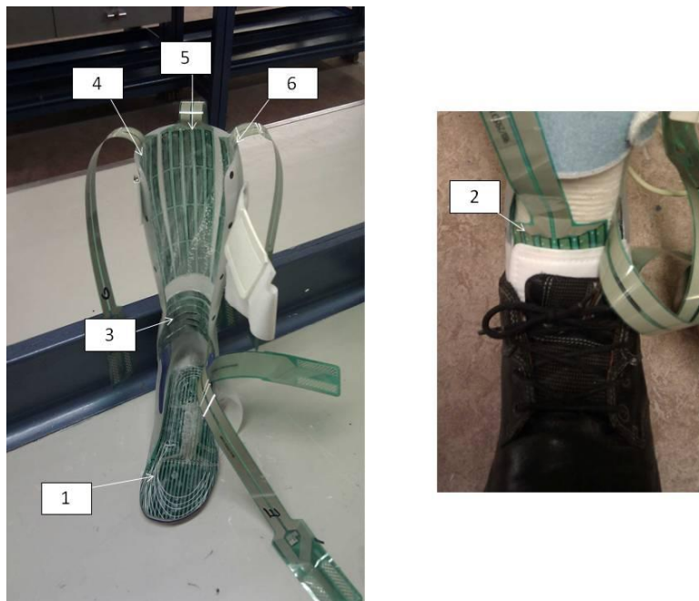
Figure 7-2: Sensor positions: 1 = plantar foot, 2 = strap, 3 = achilles tendon, 4 = medial calf, 5 = central calf, 6 = lateral calf
