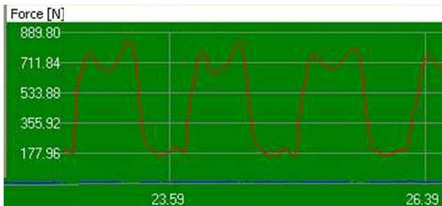
Figure 7-9: Screen shot of the force vs. time graph showing three complete gait cycles
