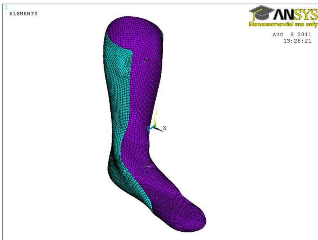
Figure 9-1: The meshed geometry with 18530 nodes and 6153 elements
