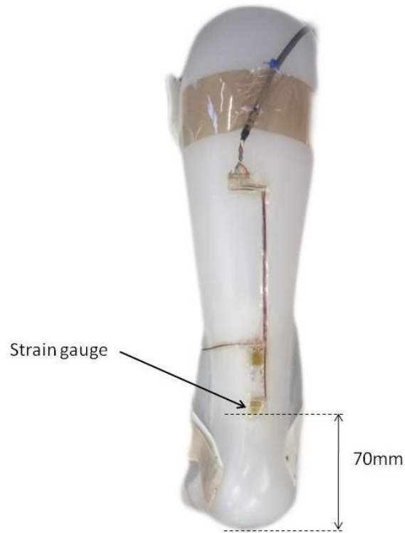
Figure 9-12: Posterior view of the AFO with strain gauge attached
