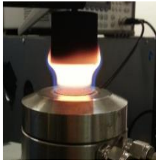
Figure 6-2: Flame @ \phi = 2.3 with stabilisation plate
