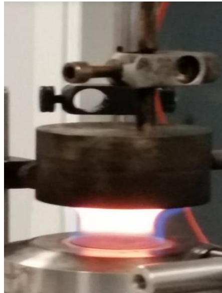
Figure 6-4: Burner with large plate(64 mm diameter) with thermocouple inserted into the stabilisation plate @ \phi = 2.2
