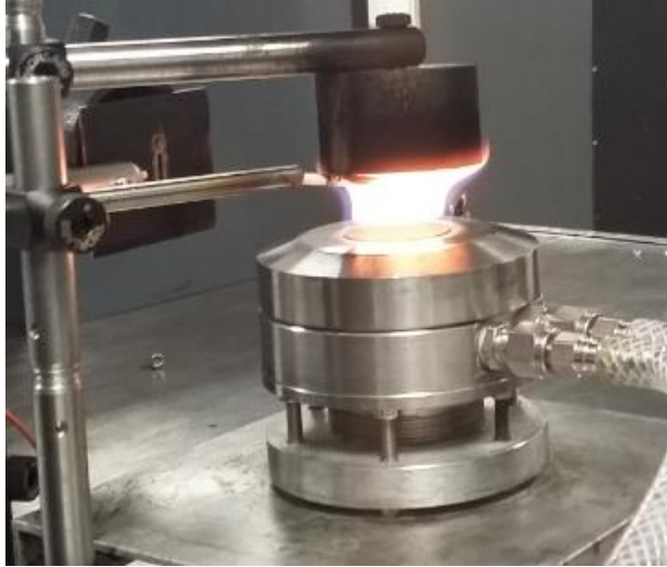
Figure 6-3: Burner with larger plate (64 mm diameter) and thermocouple intruding on the flame @ \phi = 2.2
