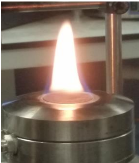
Figure 6-1: Flame @ \phi = 2.3 with no stabilisation plate
