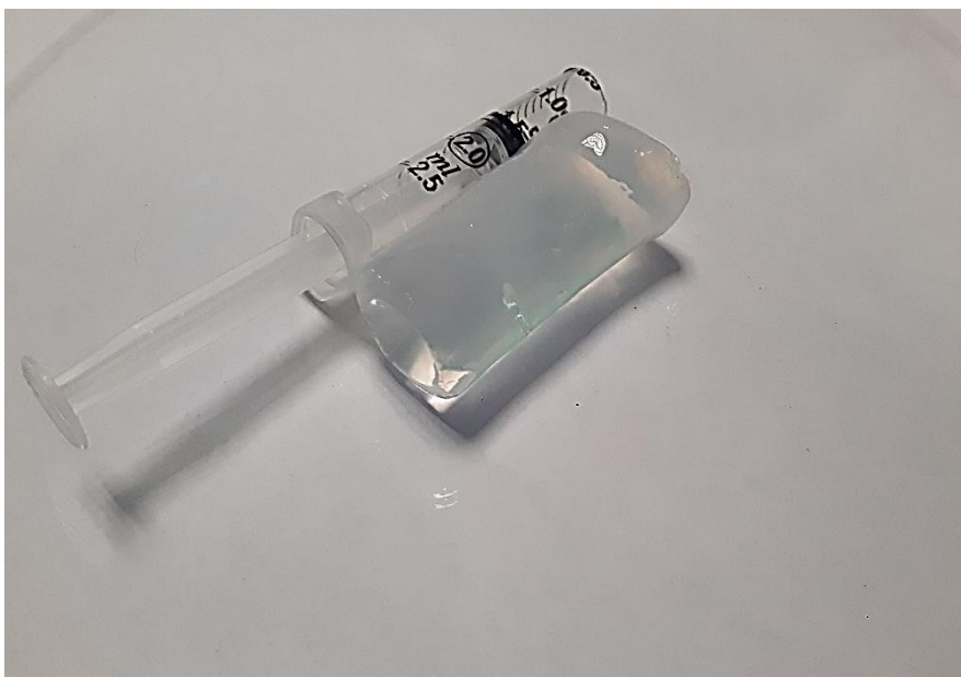
Figure 5.1: Syringe (2 mL) used as mould, and the resulting swollen \text{poly}(\text{SA}_{21.25}\text{-CO-NIPAM}_{78.09}\text{-CO-MBA}_{0.66}) hydrogel.
