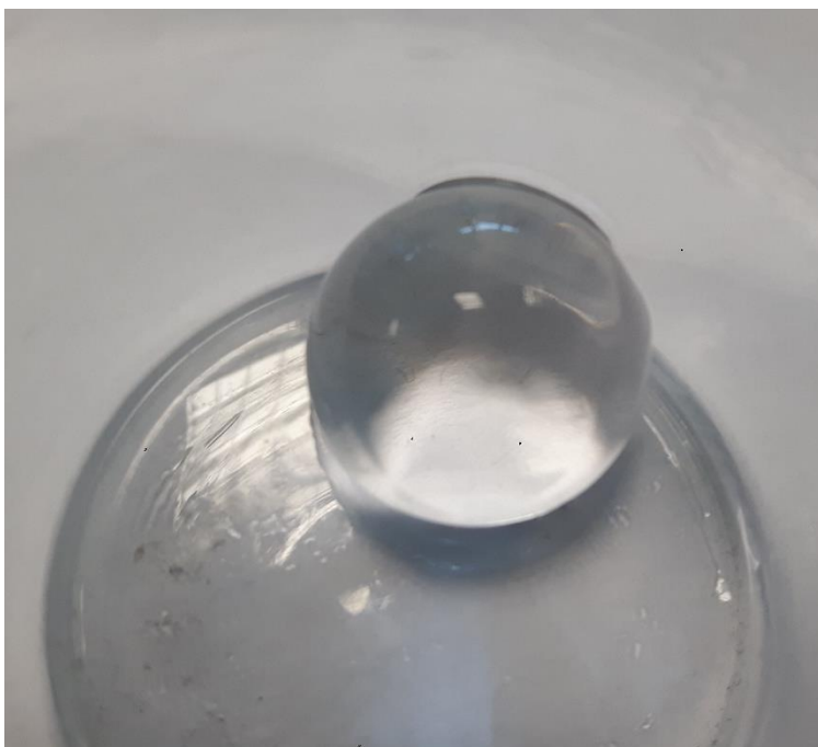
Figure 3.6: Image of a bead swollen in excess DD water, produced by the synthesis of lightly crosslinked poly(AA-co-SA) via TLSP whereby, 0.065 mol % (10 mg) of MBA was added to the monomer feed. \varnothing = 32.2 mm.
