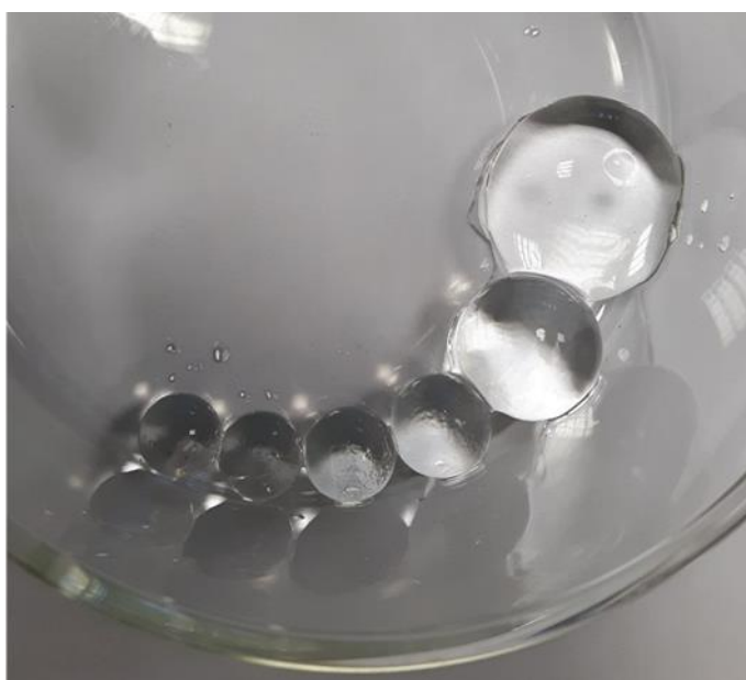
Figure 3.5: Image of individual beads swollen in excess DD water, produced by the synthesis of lightly crosslinked poly(AA-co-SA) via TLSP. The crosslinker quantity added to the monomer feed solution decreases from 0.45 to 0.13 mol % (70 to 20 mg) in steps of 0.06 mol % (10 mg) from left to right.
