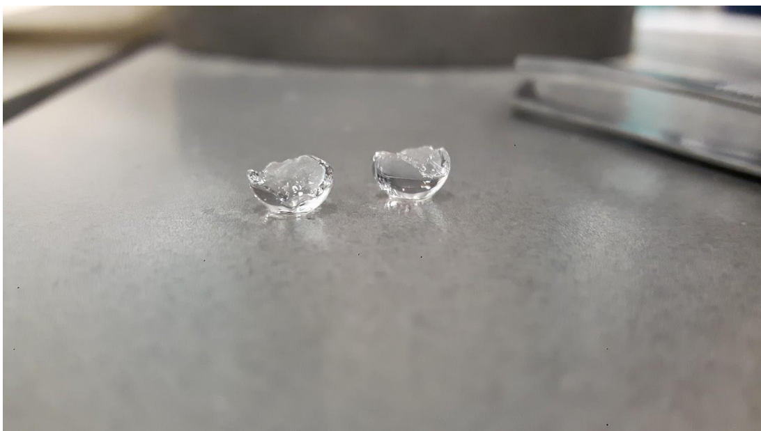
Figure 7.7: Poly( \text{Ca}^{2+} -alginate-co-AM-co-SA-co-MBA) hydrogel sphere split in two parts during a compression test.
