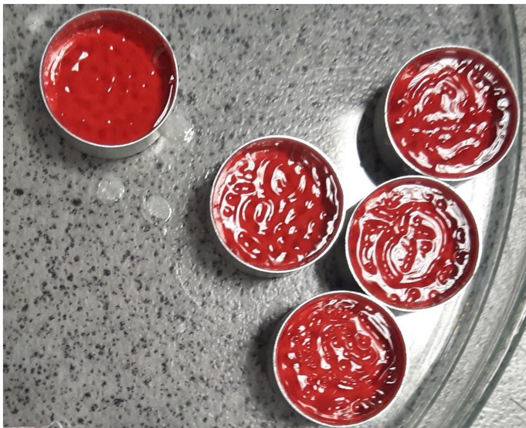
Figure 5.2: Solution polymerisation in PTFE-coated vial caps used for gas chromatography.
