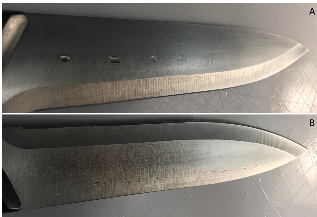
Figure 6.1: The blade of a chef knife (21 cm in length) showing the liquid deposition after tapping (A) and sliding (B) a swollen commercial hydrogel bead contained within a couplant holder from left to right.
