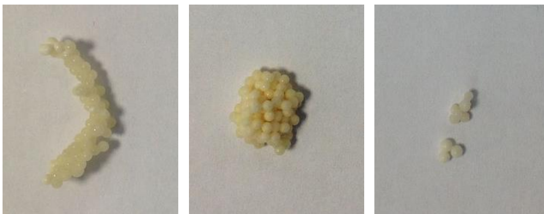
Figure 2.6: Beads produced by sedimentation polymerisations in ½ light, ½ heavy m. oil (left) and 350 cSt (middle) and 10,000 cSt (right) silicone oil.
