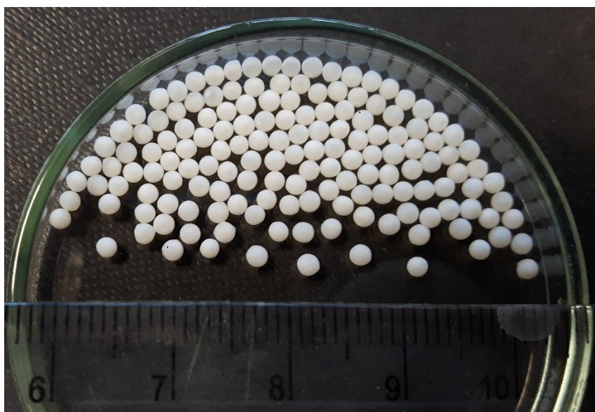
Figure 4.8: Digital picture of a typical product of dry poly( \text{Ca}^{2+} -alginate-co-AM 98.863 -co-SA 0.999 -co-MBA 0.138 ) beads synthesised by TLSP.
