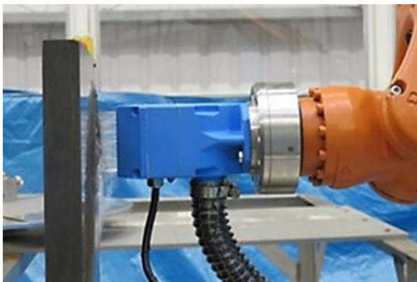
Figure 1.7: Example of an ultrasonic probe using a water jet to apply couplant.
