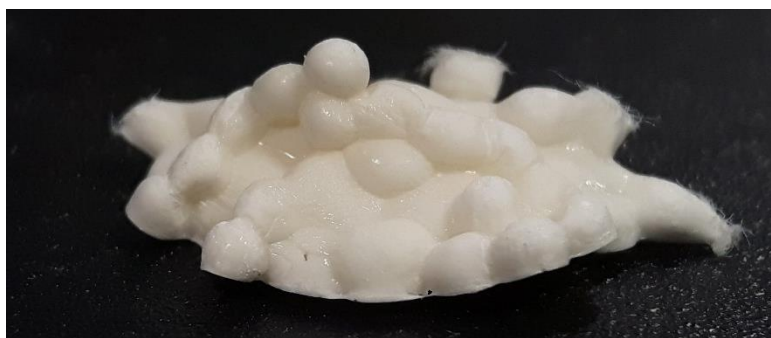
Figure 4.9: Digital picture of coagulated poly( Ca^{2+} -alginate-co-AM-co-SA-co-MBA) hydrogel prepared by sedimentation polymerisation.
