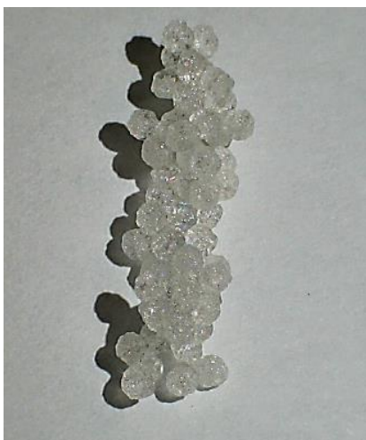
Figure 2.4: Coagulated beads prepared by sedimentation polymerisation.
