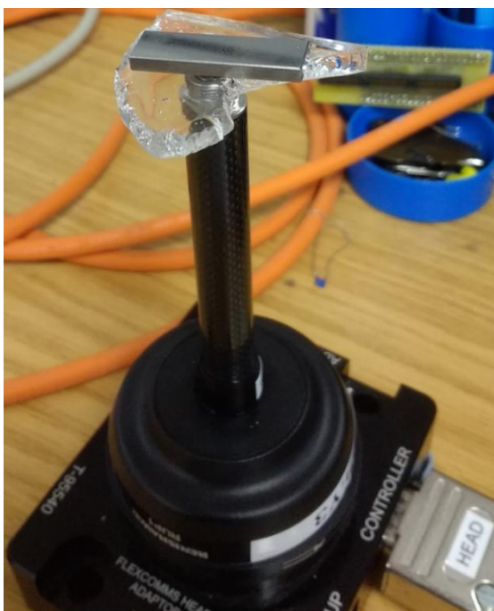
Figure 8.6: Digital picture of a piece of poly(AMPS-co-MBA)/poly(AM-co-MBA) DN hydrogel placed on top of a transducer and covered by a stainless-steel part to resemble a measurement.
