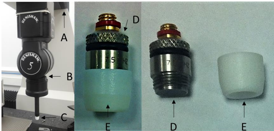
Figure 1.3: CMM (A) with an RUP-1 (B) including transducer and couplant holder (C) (left), 7.5 MHz transducer (D) connected (middle) and unconnected (right) to a couplant holder (E).
