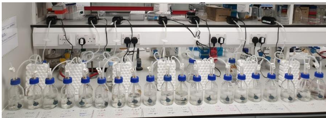
Fig. S8. Acute toxicity test set-up for Ofloxacin.
