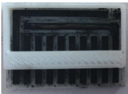
Figure 5.11: Chips produced from filling of channels printed out of PETG with a 2:1 carbon black: paraffin wax paste mixture.
