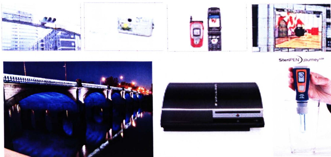
Figure 1.2 Some applications of III-nitrides. Clockwise from top left-hand side: Traffic signal lights, digital camera backlighting, cellular phone backlighting, giant outdoor screens [10], a bridge across the river Clyde in Glasgow [11], Sony Playstation 3 Blu-ray player [9], and Hydro-Photon SteriPEN™ for water purification [12].
