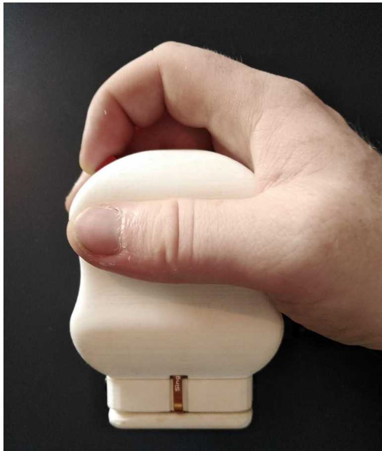
Figure 5.4 – Prototype system completed view in use. The system fits comfortably in the hand, with an easy-to-use push button on the surface to activate the IR LEDs. The hand is kept clear of the SingleTact™ pressure sensors, eliminating interference through contact.
