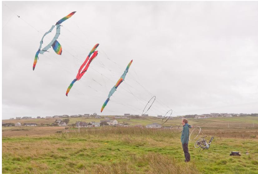
Figure 3.5: Image of a Daisy Kite prototype undergoing field tests. Three soft rotors are shown (September 2016).
