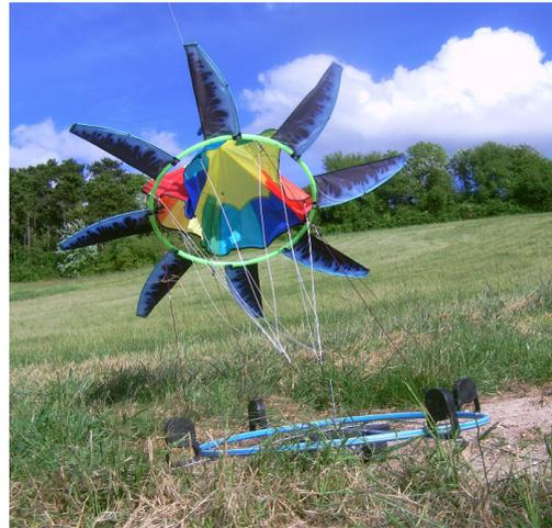
Figure 2.10: Image of the Rotating Reeling Parotor prototype [7]
