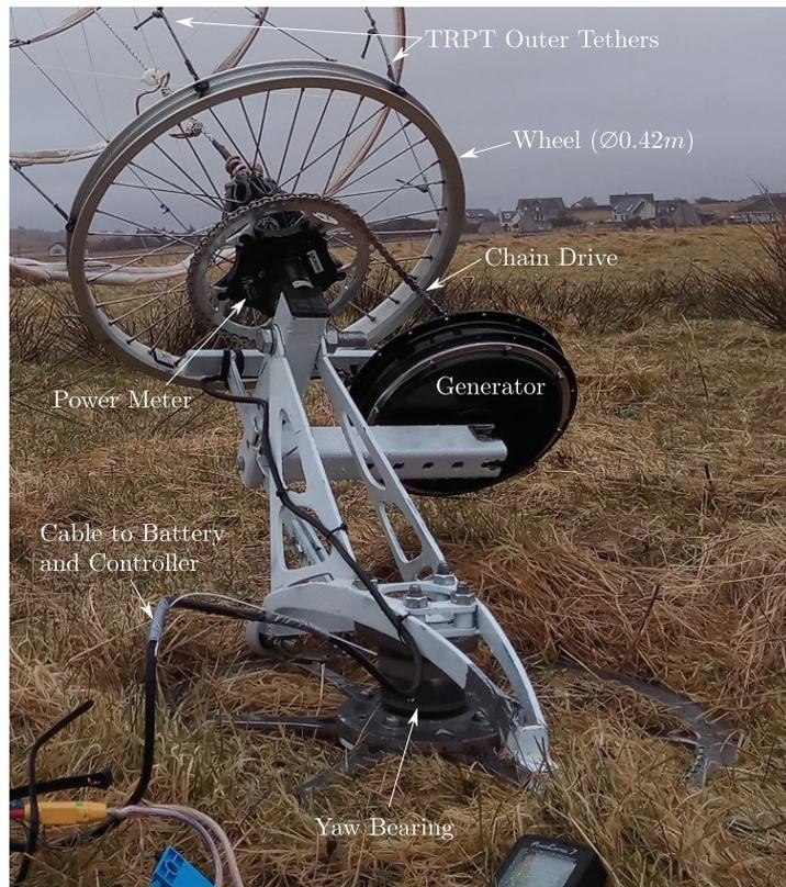
Figure 3.14: Image of the Daisy Kite ground station with key components labelled.
