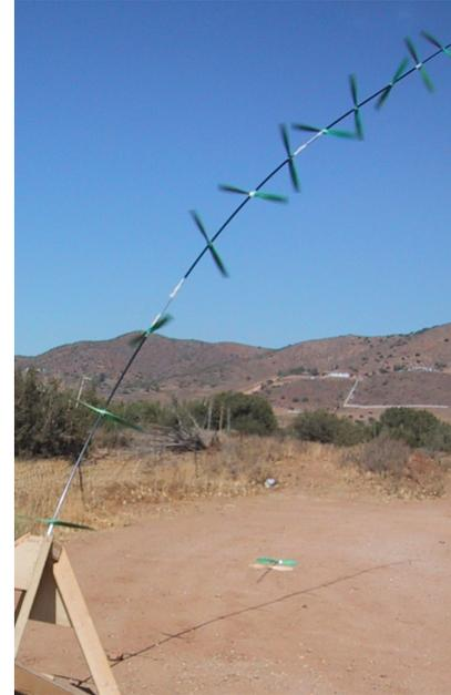
Figure 2.14: Image showing one of Selsam Innovations Superturbine prototypes [12]
