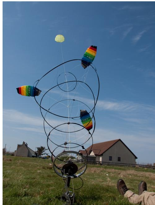
Figure 3.19: Image of the first Daisy Kite prototype for which performance data has been collected (May 2017).
