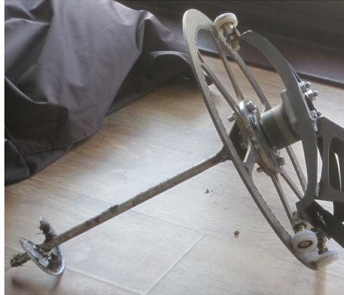
Figure 3.15: Image of the Daisy Kite's ground station screw anchor.
