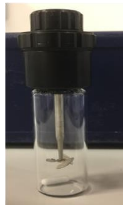
Figure 6-5 Crystalline instrument (left) close-up of an individual 8 ml crystalline vial with the top stirrer (right).
