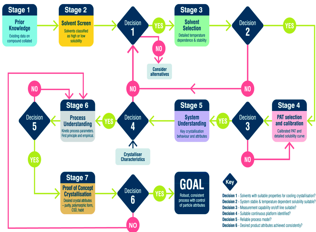
Figure 1-25 Workflow for seeded continuous crystallisation. Adapted from Brown et al. [150].
