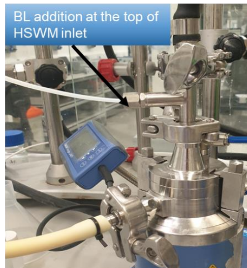
Figure 6-36 Modified BL addition point via T-Piece at the inlet of the HSWM
