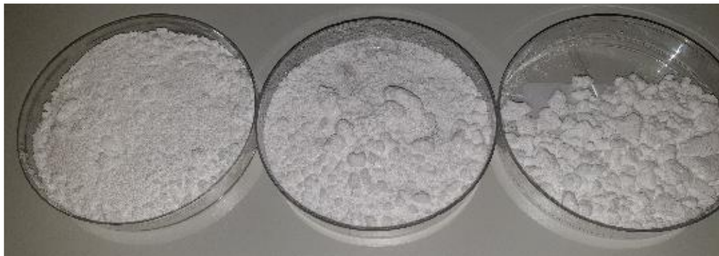
Figure 6-10 Washing protocol; No wash, Heptane wash and water wash from left to right.
