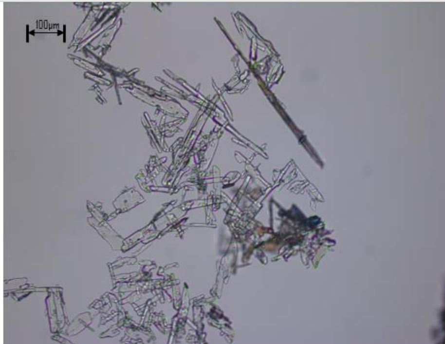
Figure 6-17 (Top) PSD of primary BA crystals before and after the pre-milling and (Bottom) microscopic image of the primary crystals, small needles of BA can be observed.
