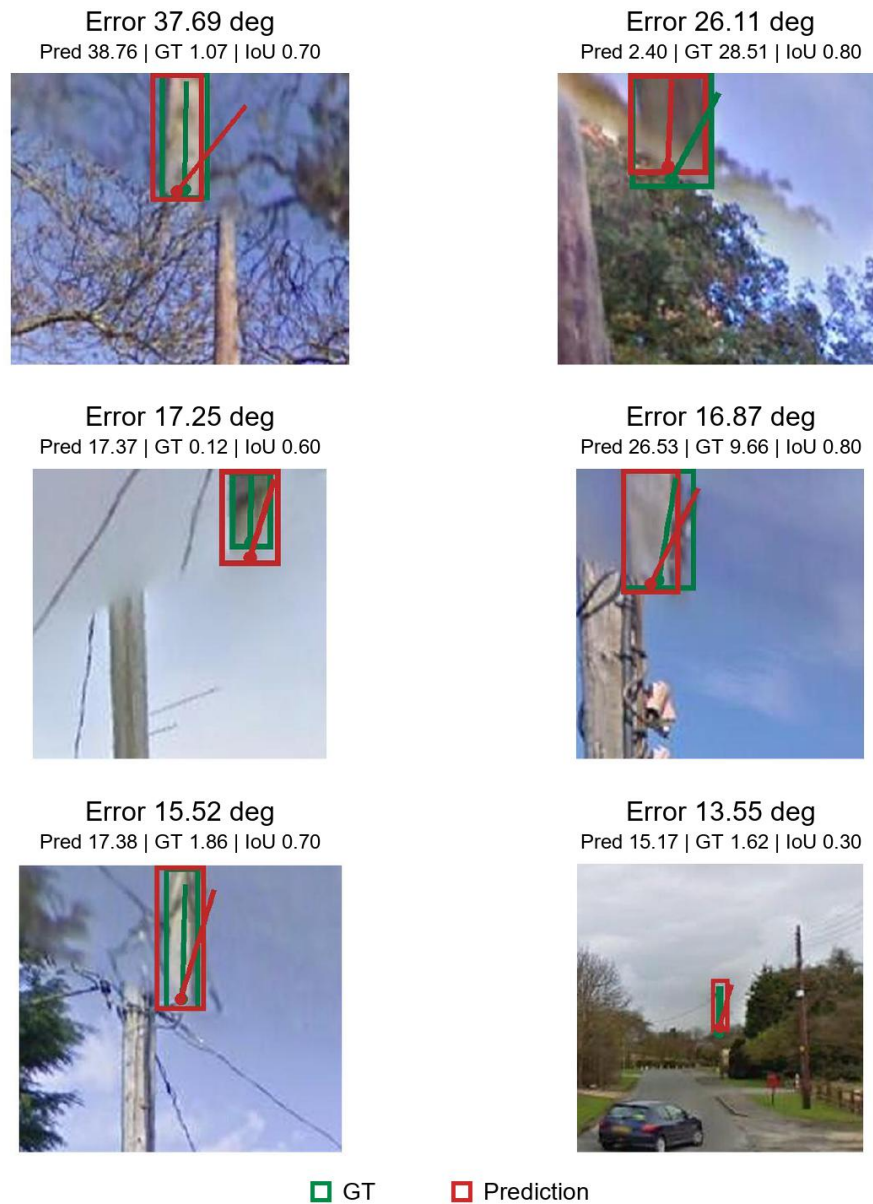
Figure 4.21: Highest-error DETR segmentation lean-angle examples. Green indicates the ground truth and red indicates the prediction.
