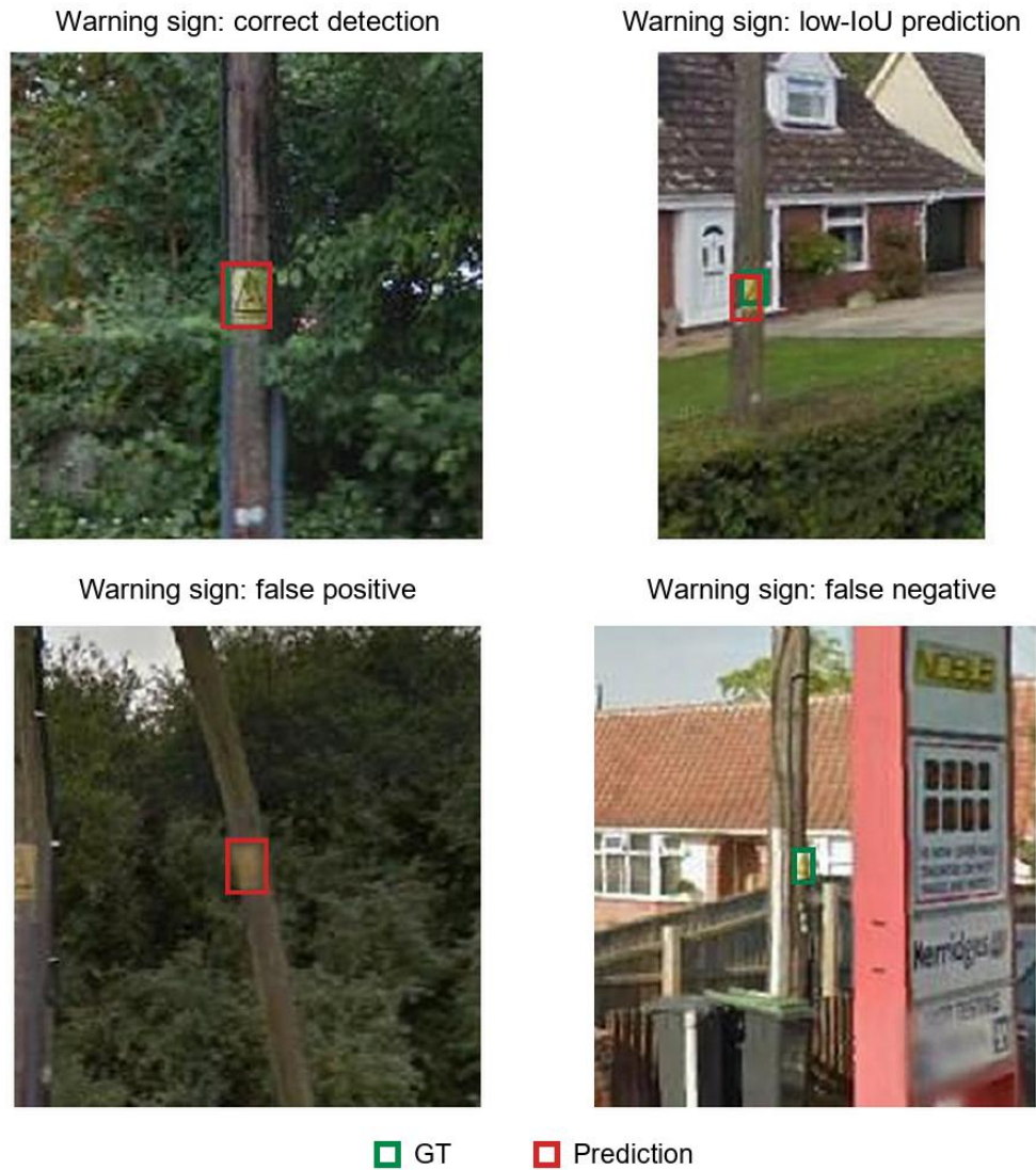
Figure 3.8: Representative DETR warning-sign detection outcomes on the held-out test split, including a correct detection, a low-IoU detection, a false positive, and a false negative. Green boxes show ground truth and red boxes show predictions.
