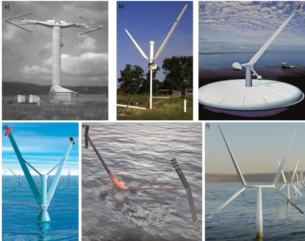
Figure 3.13: a) Musgrove 250 turbine [4], b) 5kW V-Rotor tested by Sharpe and Taylor [5], c) Single bladed V-VAWT concept [6], d) Taylor V-Turbine [5], e) The aerogenerator concept [6], and f) the X-Rotor wind turbine concept.
