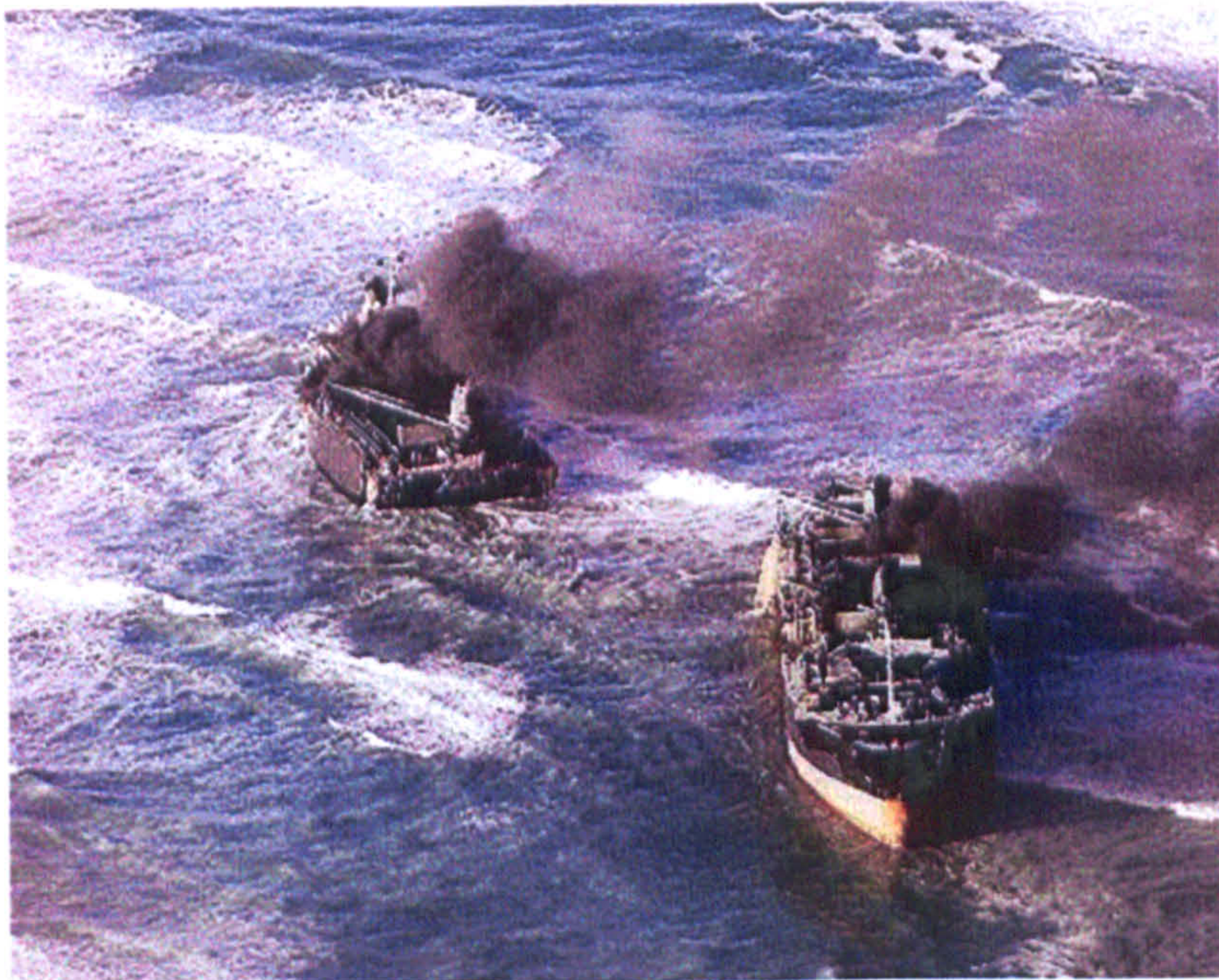
Figure 1.1: Complete hull failure in a stranded bulk carrier, NEW CARISSA
