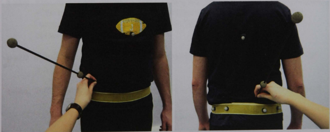
Figure 4.18: Pointer trial calibration of anatomical landmarks of the pelvis (right ASIS and right PSIS)
