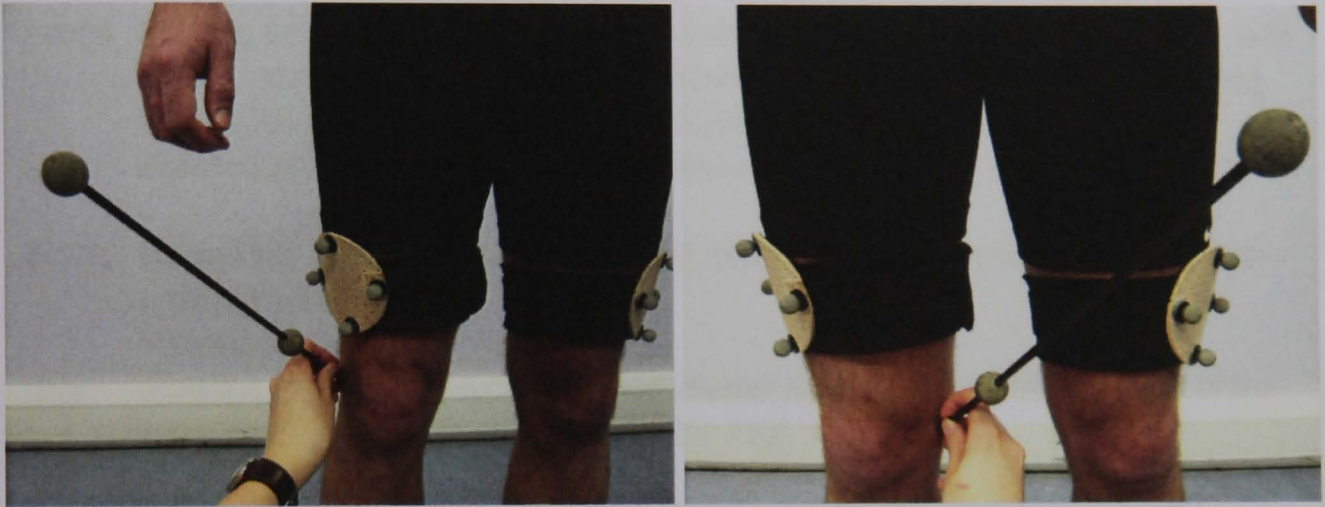
Figure 4.23: Pointer trial calibration of anatomical landmarks of the femur (right lateral and right medial epicondyle)
