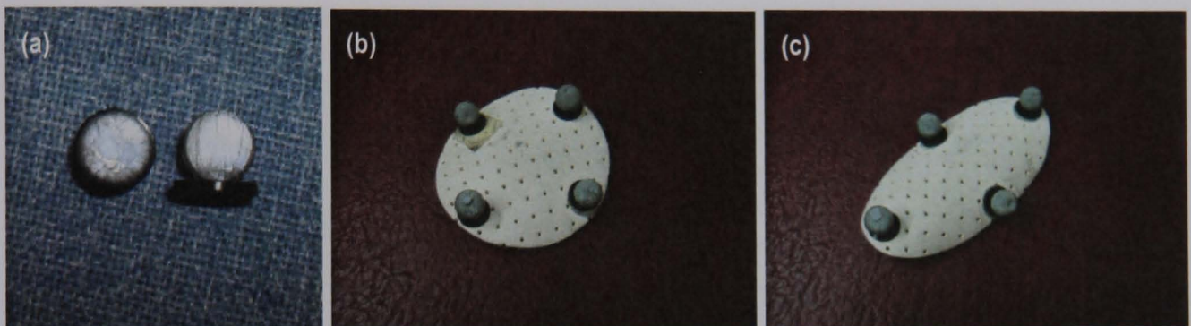
Figure 4.7: Individual 14mm markers (a) and marker clusters for thigh (b) and shank (c) segments
