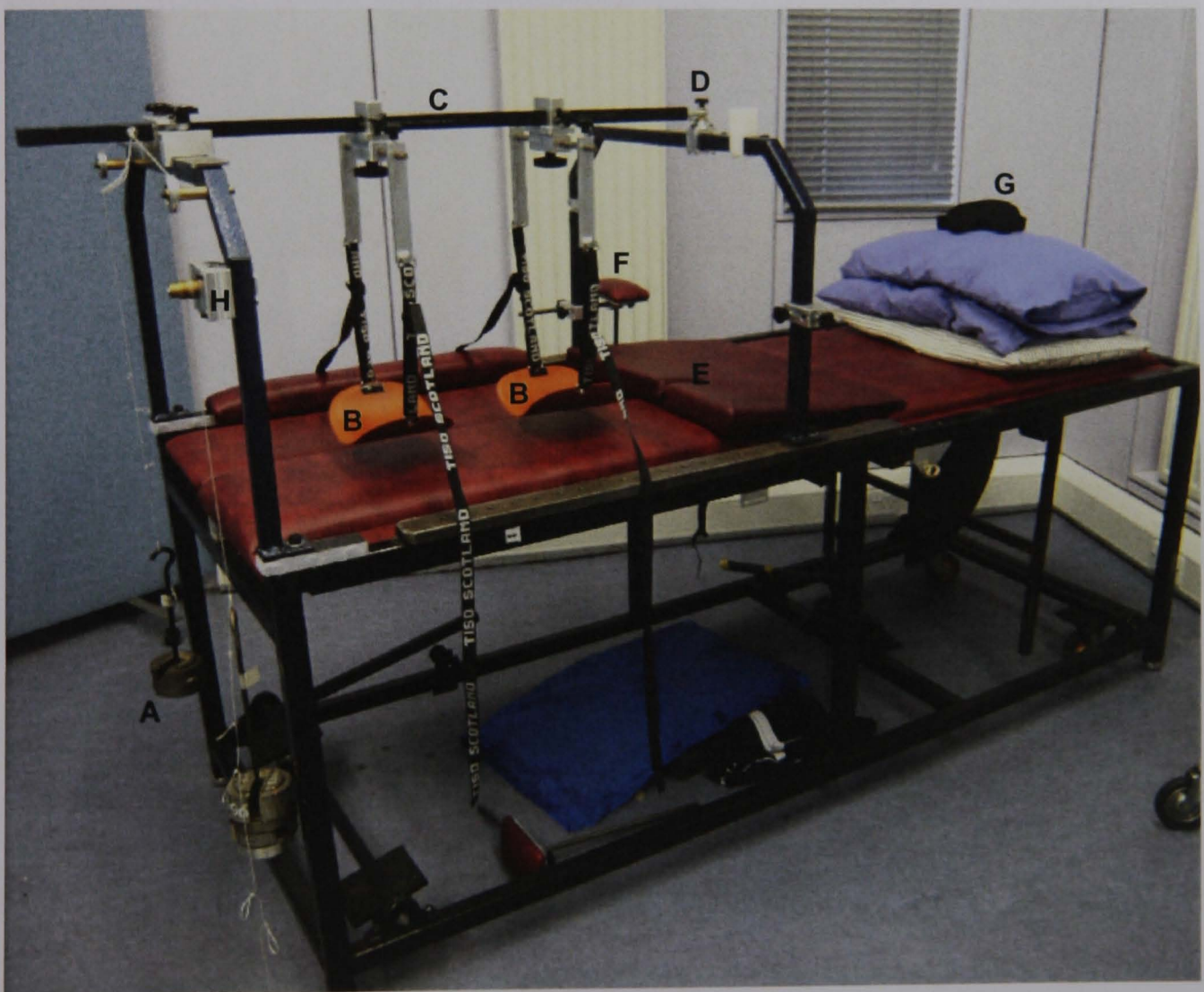
A-Pulley system; B-Limb cradles; C-Limb suspension beam, D-Sliding pivot point of beam, E-Padded wedge; F-Padded pelvis clamp; G-Eye mask; H-Viscous damper
