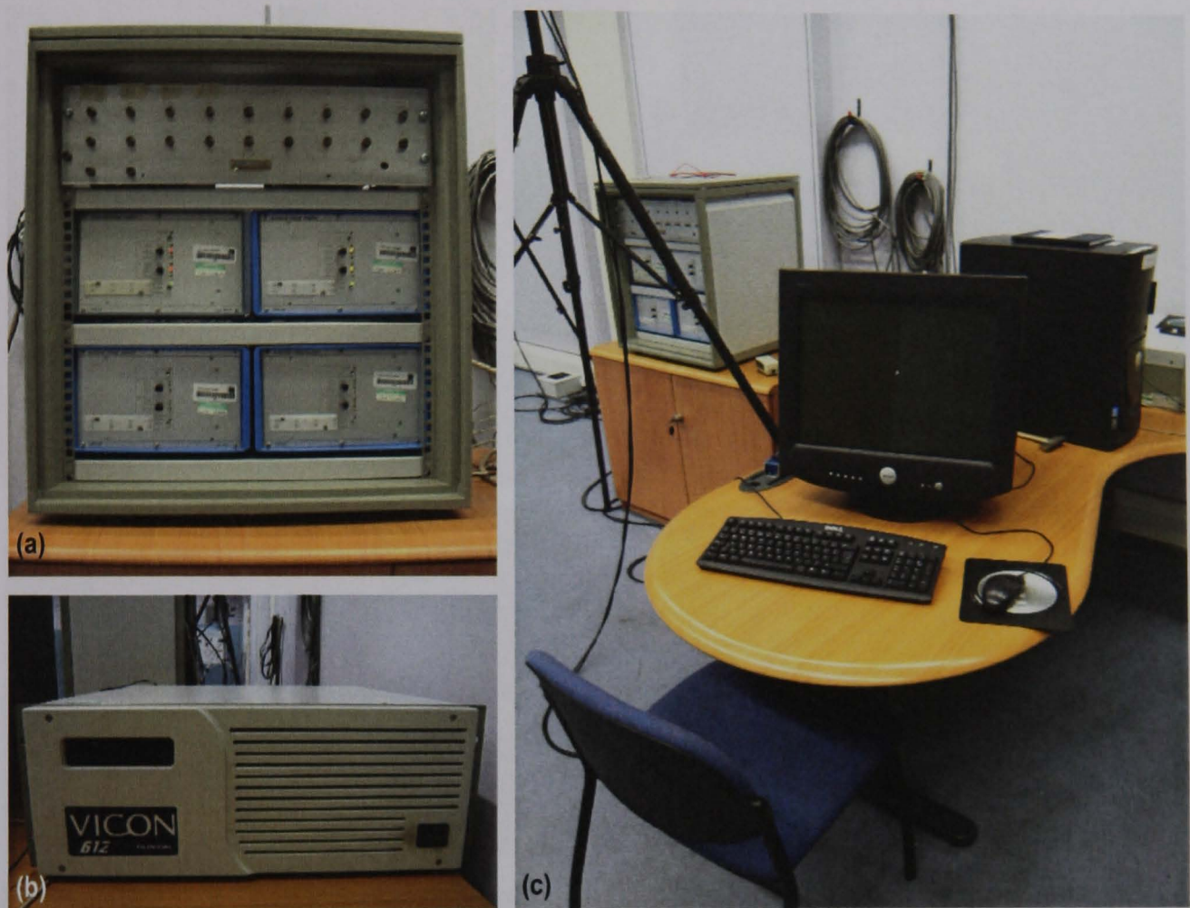
Figure 4.5: Patch-panel with force plate panels (a), Vicon data station (b) and PC (c)
