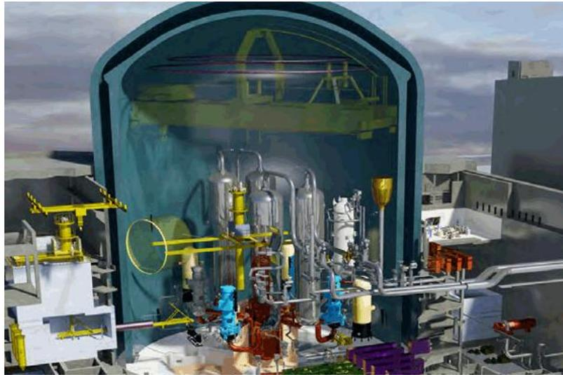
**Figure 1.2 - 3D Model of the EPR Reactor**
