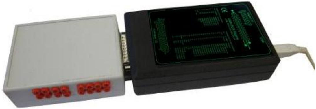
Figure 5.5: EMG/FSR preamplifier connected to the USB-DUX Sigma board. The preamplifier (white box) connects directly to the USB-DUX Sigma data acquisition device (black box) via a D-connector so the equipment is compact for easy attachment to the participant during walking. The eight bi-polar sockets for connecting to the surface EMG electrodes are visible on the side of the preamplifier box (red).
