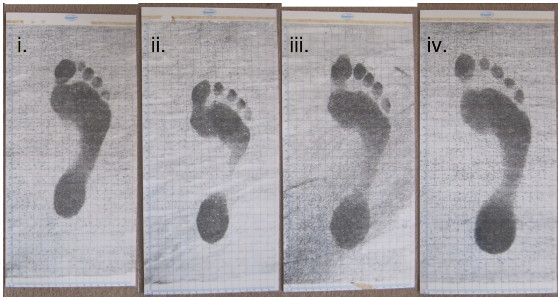
Figure 4.2: Foot impression sheets were used to make insoles for each study participant. The ink is deposited on the film in the areas of highest pressure under the feet. This allows accurate measurement of where the FSRs should be positioned on the insole for recording foot contact data. Each photo (i-iv) is a foot impression from a different subject.
