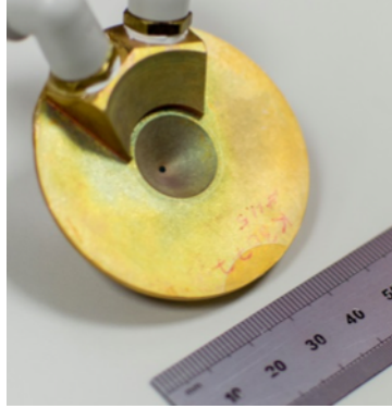
Figure 4.2: Photo of the mount used to clamp the SDL chip.
