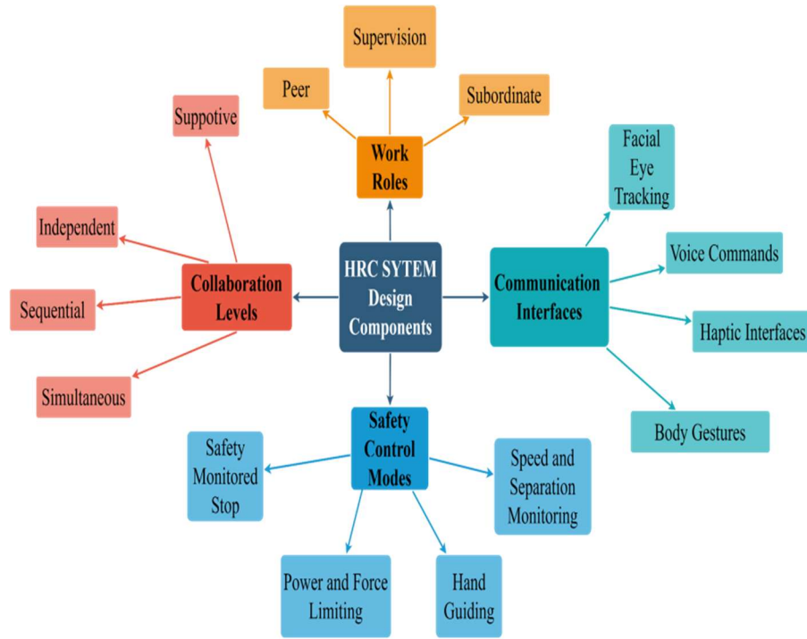
Figure 3.1 Structural components of HRC system.
