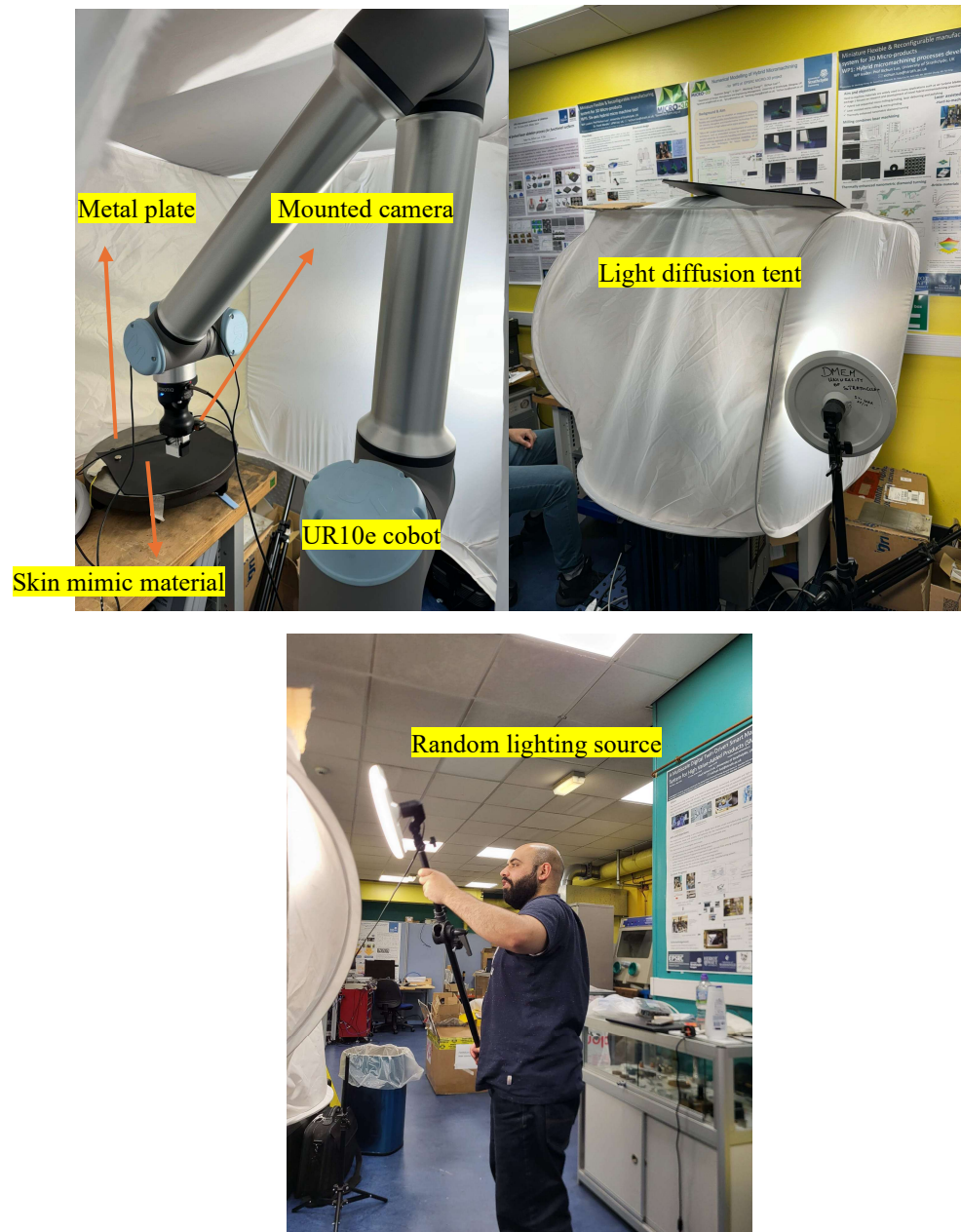
Figure 4.5. Experimental setup with cobot, camera, and lighting conditions
