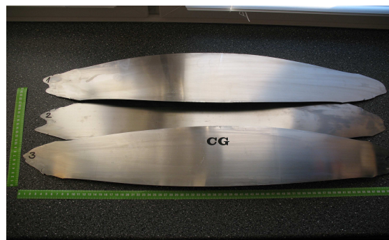
Fig. 3.17: Aluminium sheets AA 1070 after side upsetting and rolling
