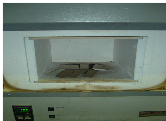
Fig. 3.15: Annealing process of aluminium sheet AA 1050
