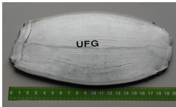
Fig. 3.25: Upset sample of 3.8 – 4.0 mm thickness
