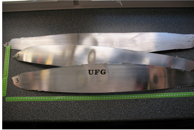
Fig. 3.26: UFG sheets produced after 6 passes of cold-rolled
